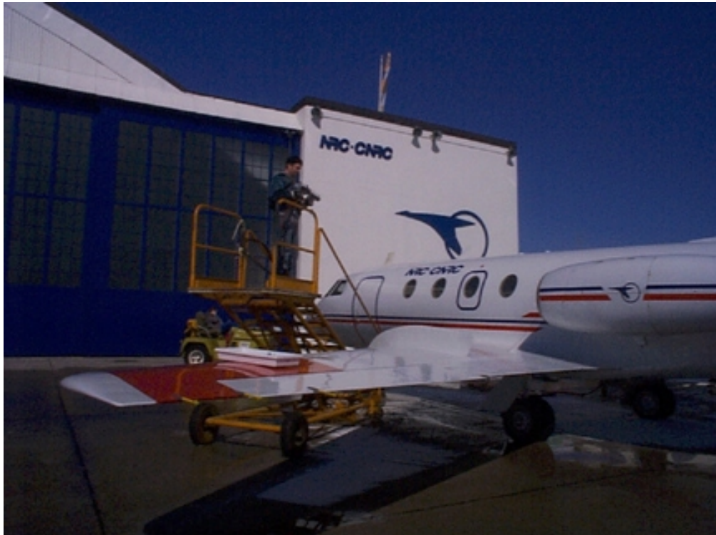
Photo 2.16: Calibration Tests with Freezing Rain Sprayer at NRC
