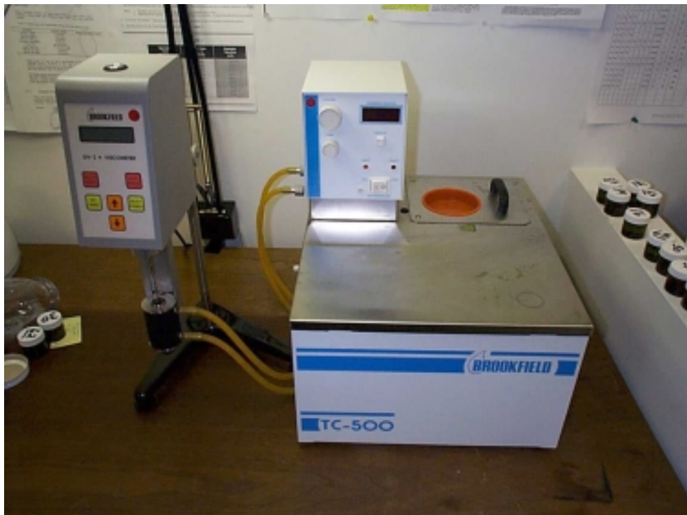
Photo 2.18: Brookfield Digital Viscometer Model DV-1+ and Temperature Bath
