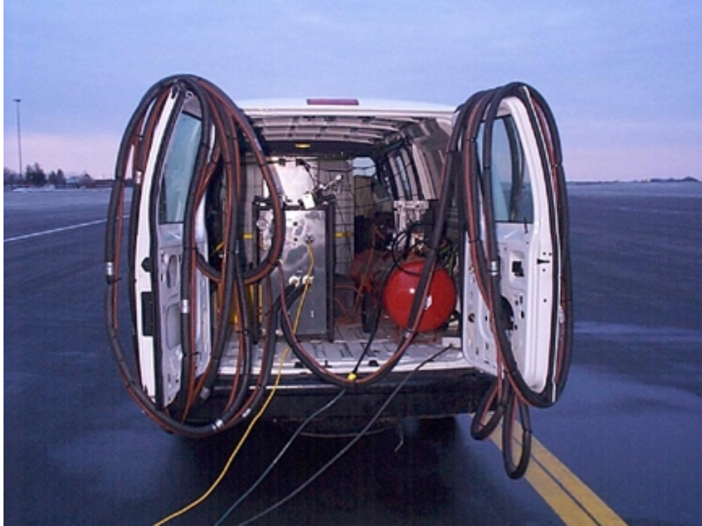
Photo 2.15: Freezing Rain Sprayer with Hoses
