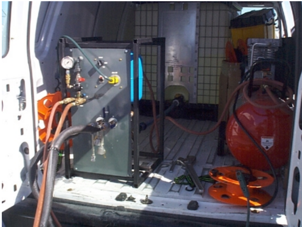
Photo 2.14: Freezing Rain Sprayer in Rental Van
