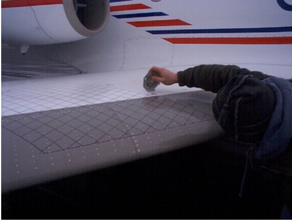
Photo 2.9: Thickness Measurement Following Takeoff Run
