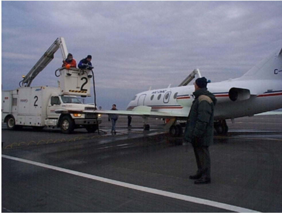
Photo 2.5: Freezing Rain Sprayed on Falcon 20
