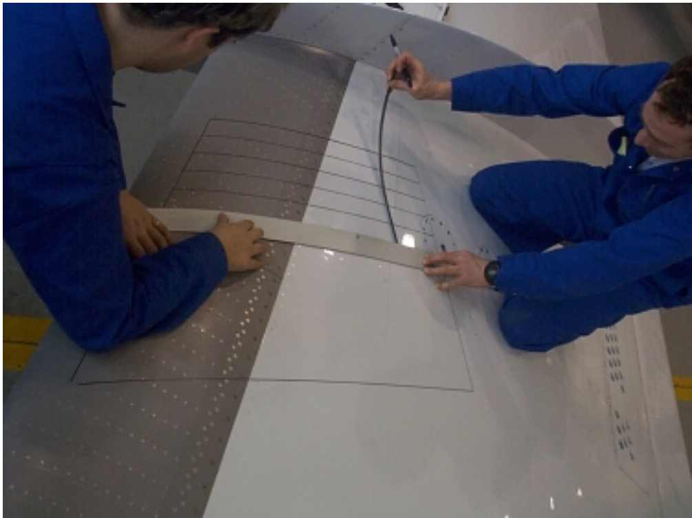
Photo 2.2: Drawing of Grid on Falcon 20 Wing
