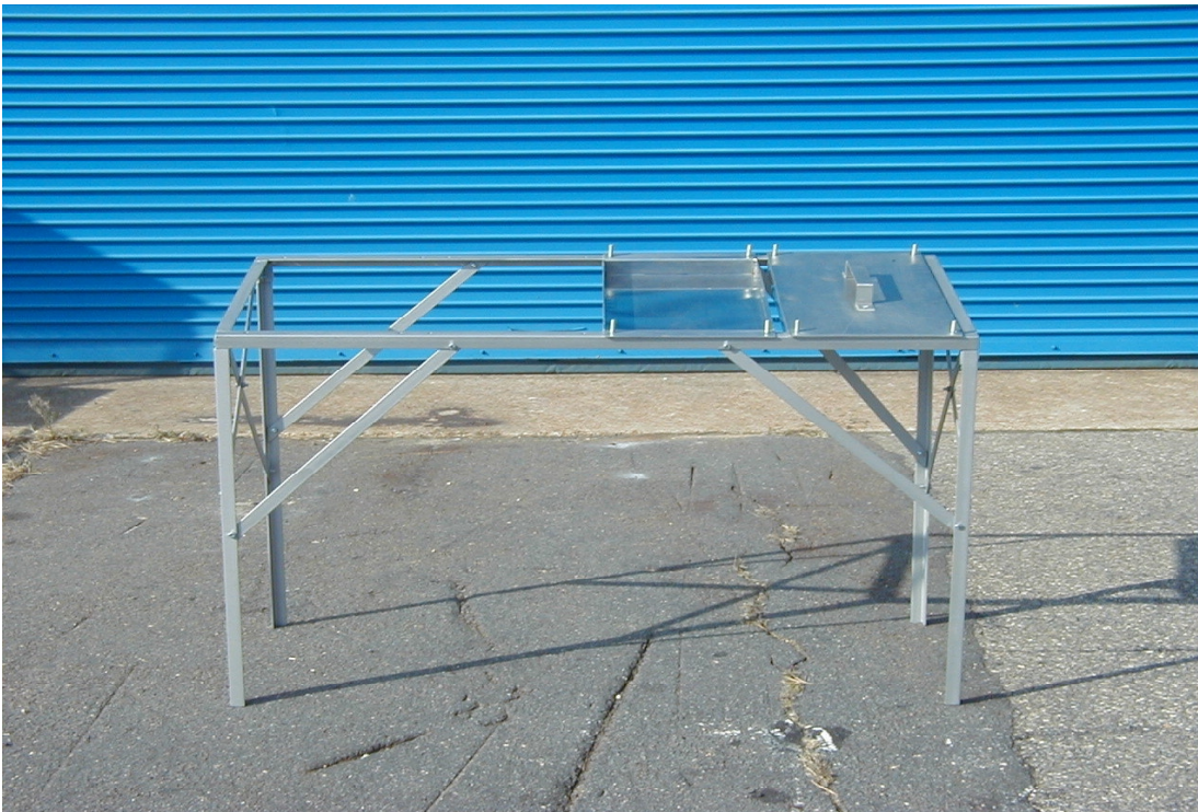
Photo 4.4: Test Stand Used for CRDA Rate Measurements
