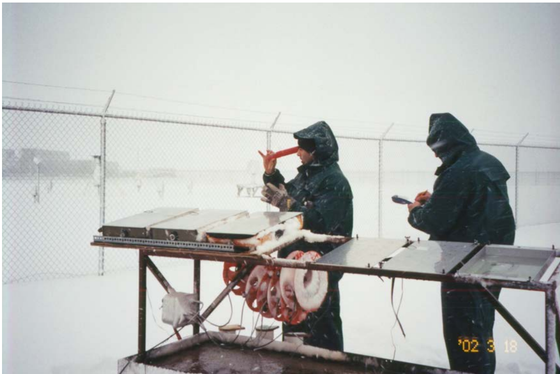
Photo 4.2: APS Test Site – Test Stand Used for Type I Endurance Time Tests
