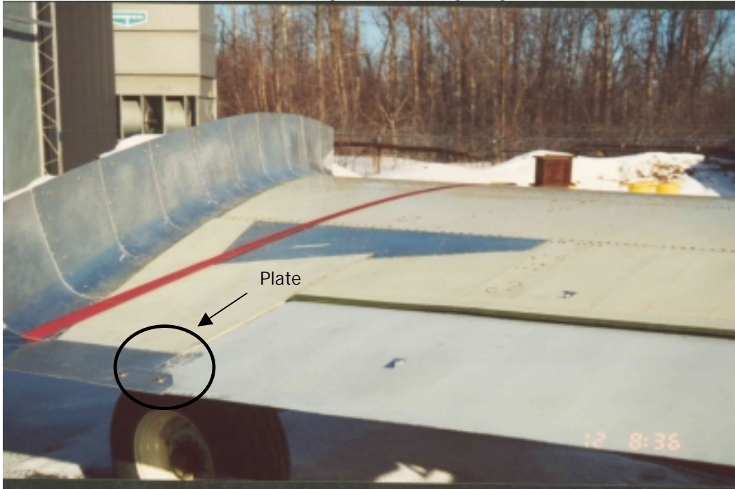
Photo 2.13 Simulated Fairing and Trailing Edge Plate
