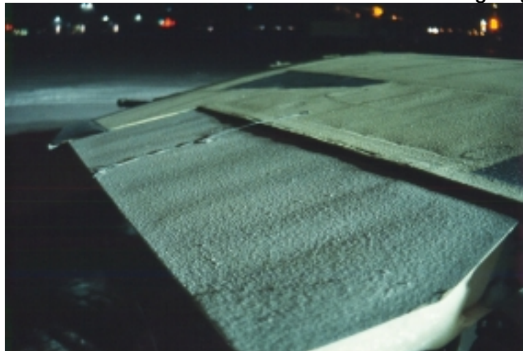
Photo 4.4 Snow Failure on the JetStar Trailing Edge
