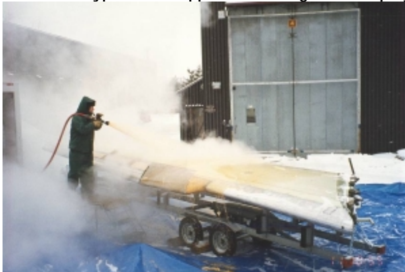
Photo 4.2 Type I Fluid Application Using Mobile Sprayer
