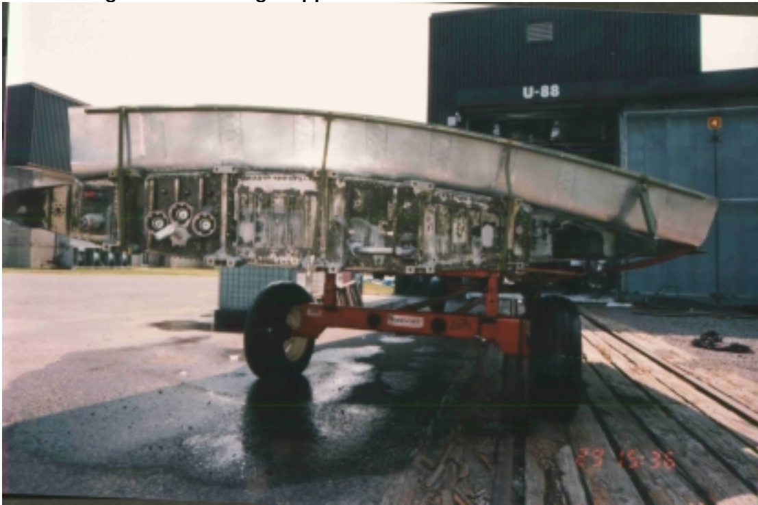
Photo 2.10 Wing Root Showing Capped Fuel Lines and Sealed Fuel Tanks
