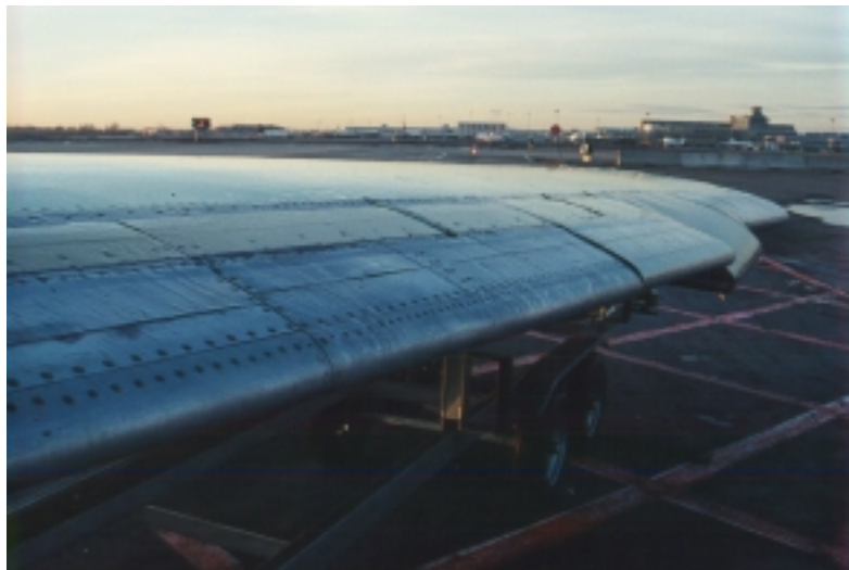
Photo 4.6 Snow Accumulation on the JetStar Trailing Edge
