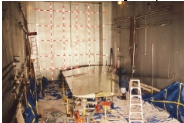
Photo 4.8 Freezing Rain on JetStar Wing Prior to Forced Air Deicing
