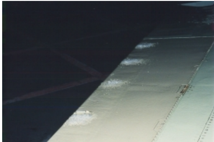
Photo 4.6 Snow Accumulation on the JetStar Trailing Edge
