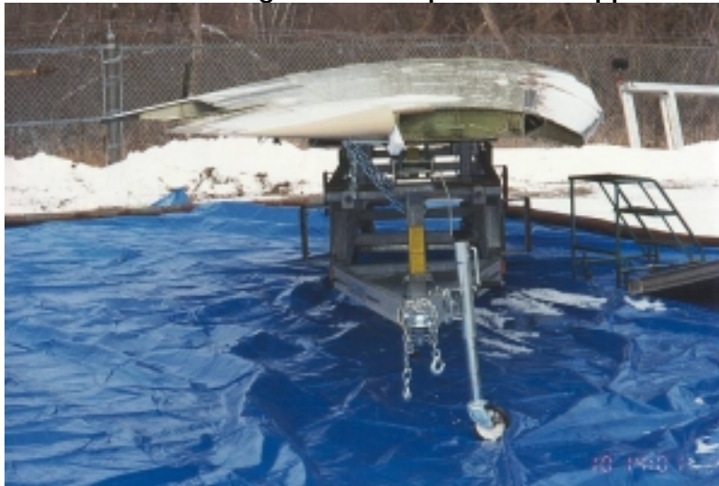
Photo 4.1 JetStar Wing Test Set-Up for Fluid Application Tests
