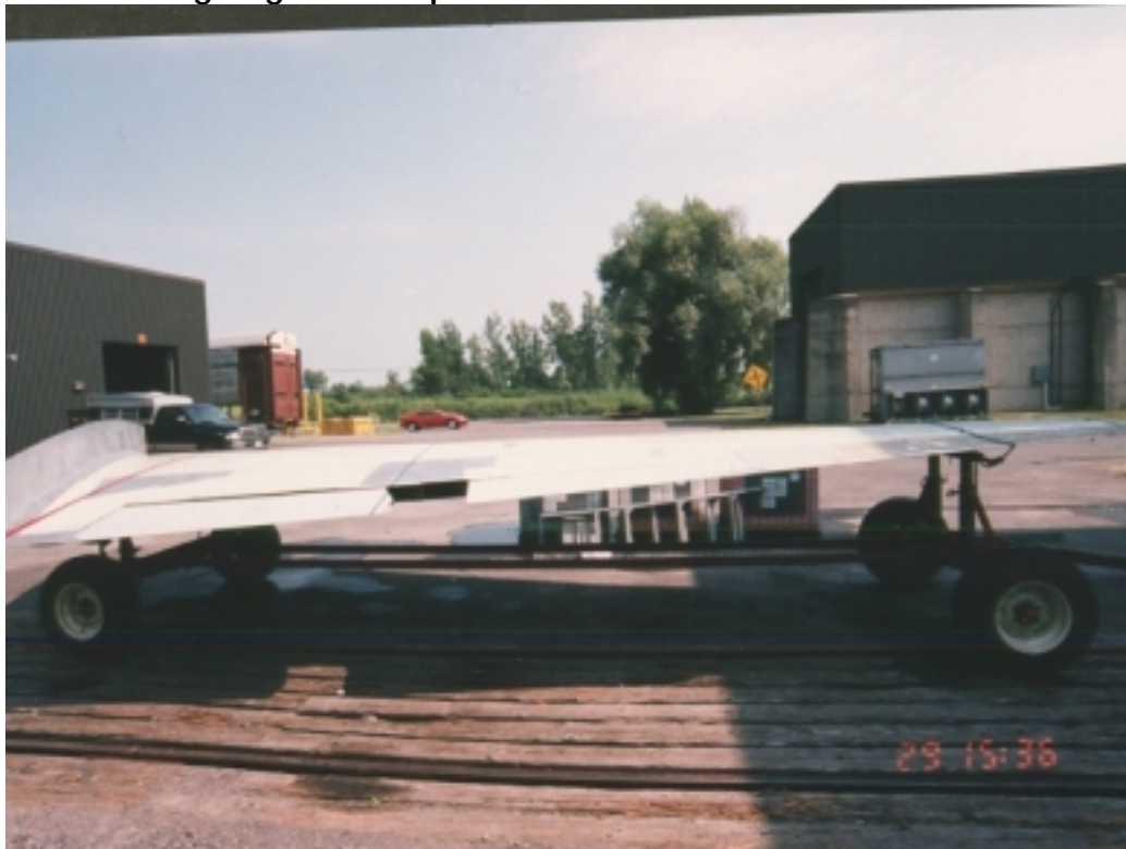
Photo 2.14 View of Trailing Edge and Gap Left from Removal of the External Fuel Tank
