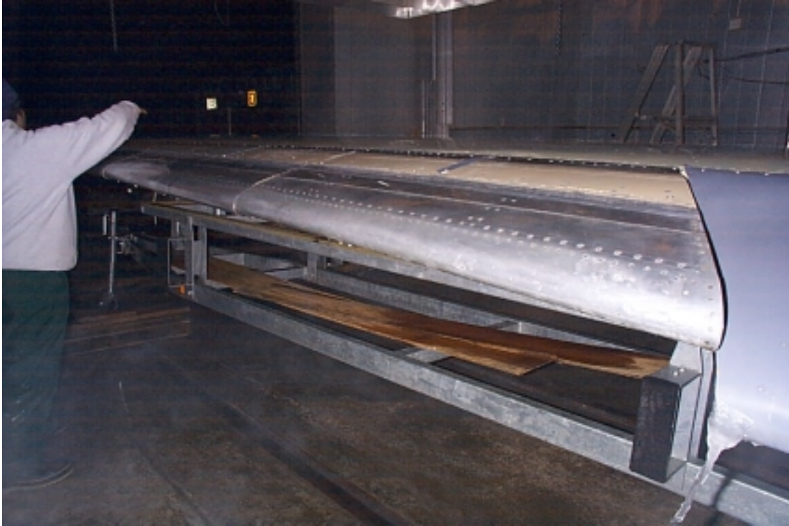
Photo 2.9 Polished Leading Edge of JetStar Wing
