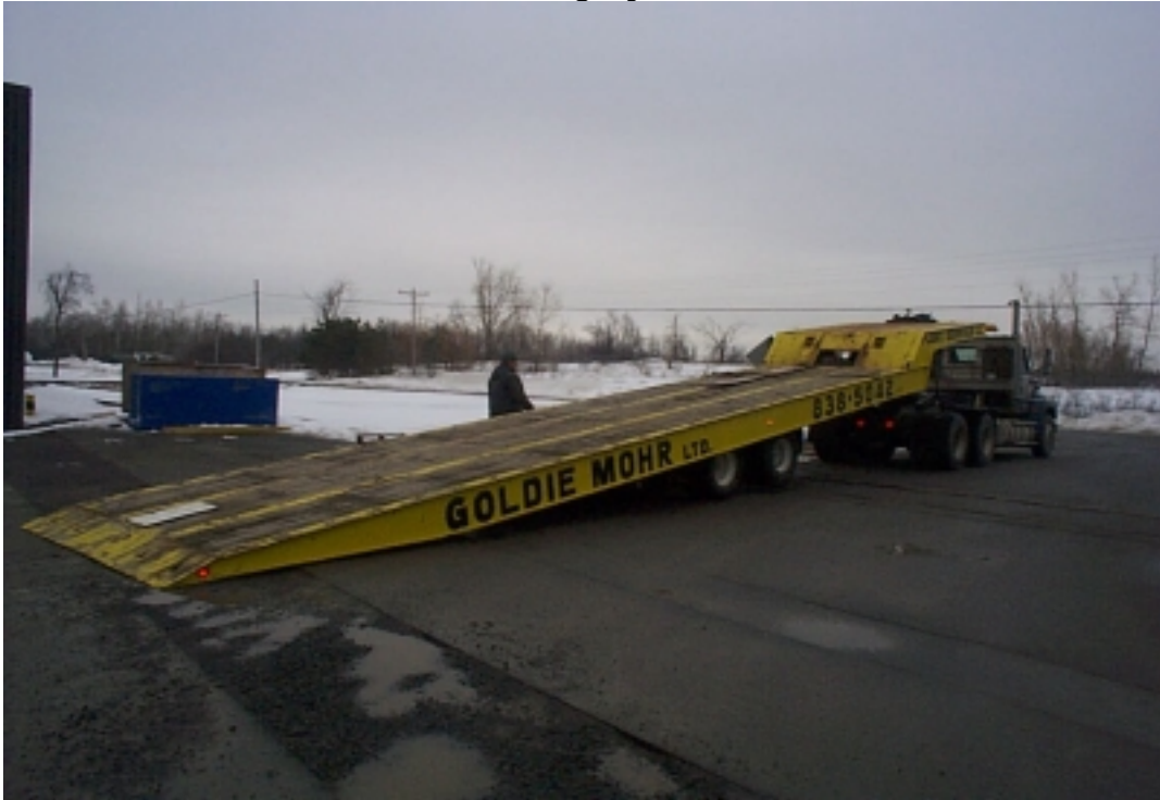
Photo 2.17 Flatbed Truck Moveable Ramp Used to Transport JetStar Wing and Wing Mounting System
