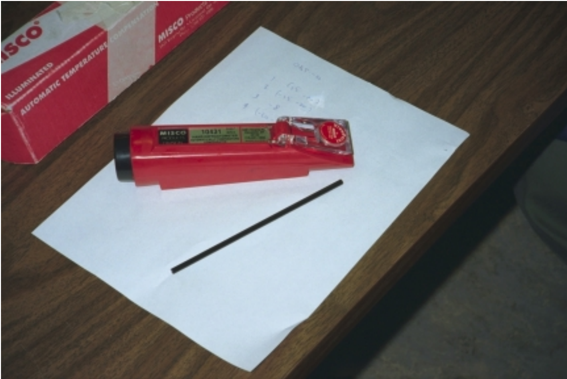
Photo 2.13 Misco Refractometer Used to Measure Freeze Point
