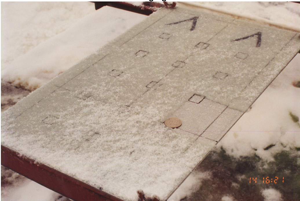
Photo B-2 Snow-bridging Failure
