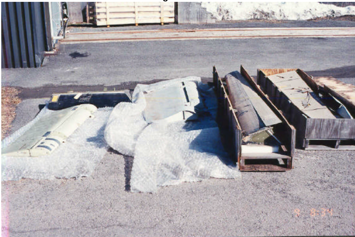
Photo 2.4 JetStar Wing Control Surfaces
