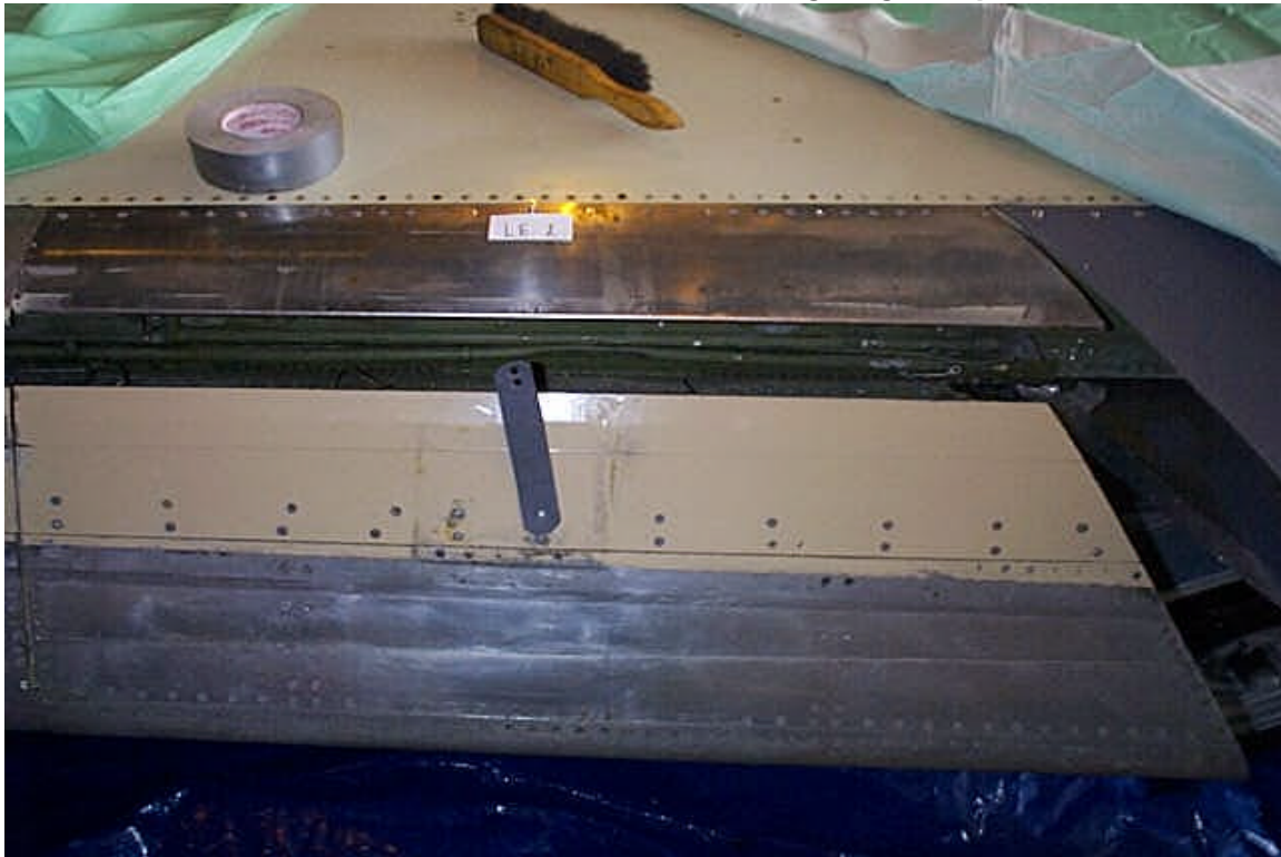
Photo 2.7 Bracket Used to Secure Leading Edge Flap
