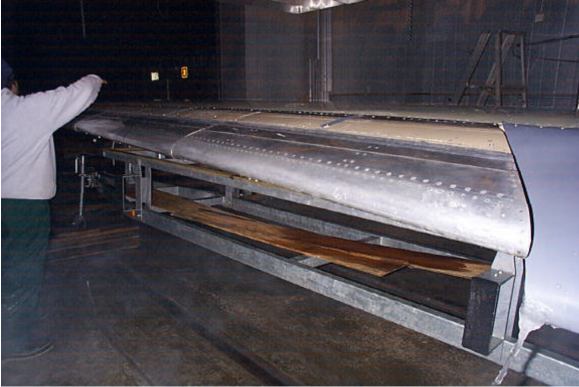
Photo 2.9 Polished Leading Edge of JetStar Wing
