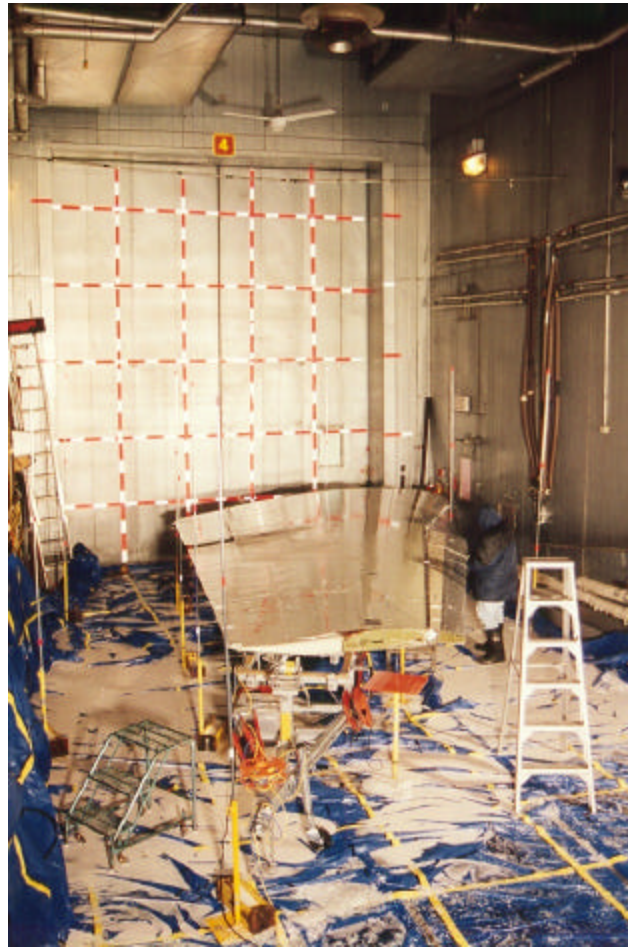
Photo 2.6 Device to Measure Force of Air Stream
