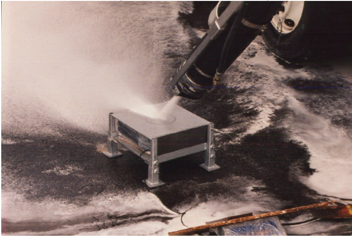
Photo 2.7 Measuring Air Stream Force at Close Range
