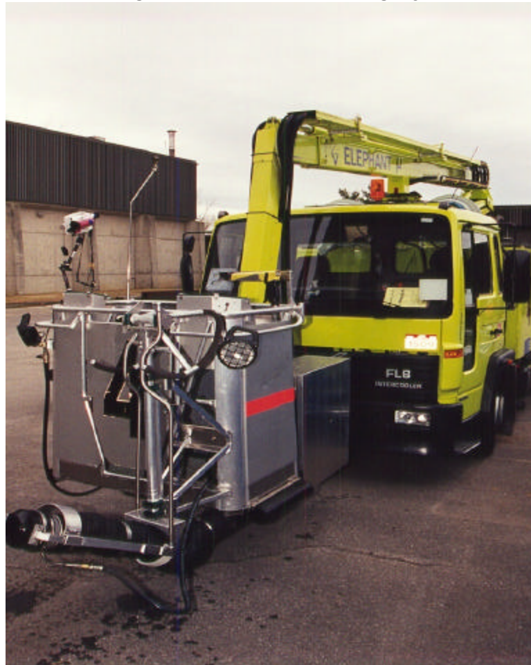
Photo 2.18 Forced Air System Installed on Bucket
