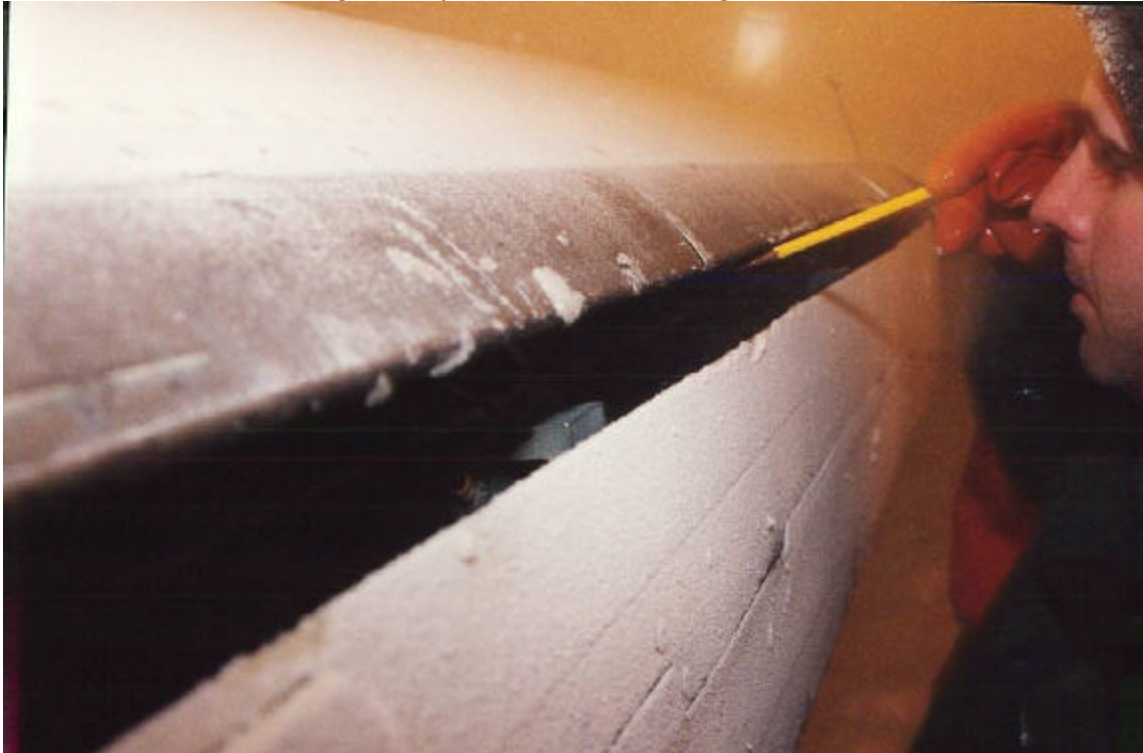
Photo 4.6 Slush Residue in Leading Edge Slat Cavity Following Air/Injected Fluid Deicing of Wet Snow
