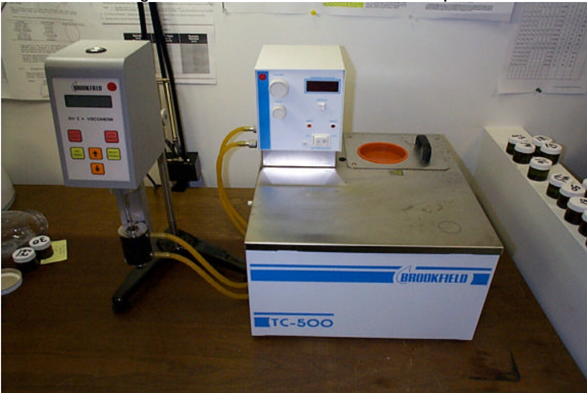
Photo 2.16 Brookfield Digital Viscometer Model DV-I+ and Temperature Bath
