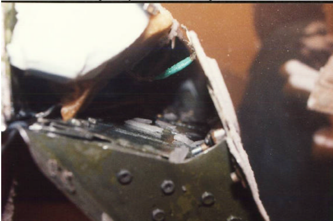
Photo 4.6 Slush Residue in Leading Edge Slat Cavity Following Air/Injected Fluid Deicing of Wet Snow
