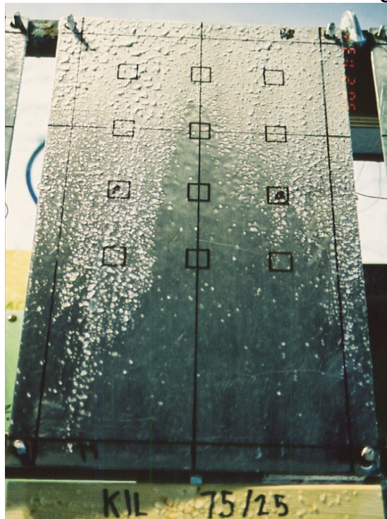
Photo 3.2 Intra-Laboratory Natural Snow Tests Kilfrost ABC-S 75/25 Fluid Five Minutes Following Plate Failure
