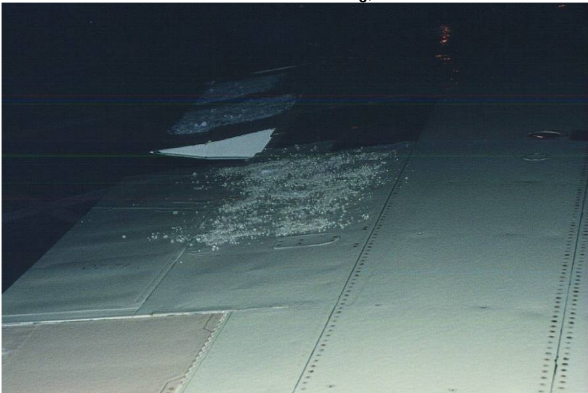
Photo 3.9 Granular Snow Patch on Main Wing, 10+ mm Thick
