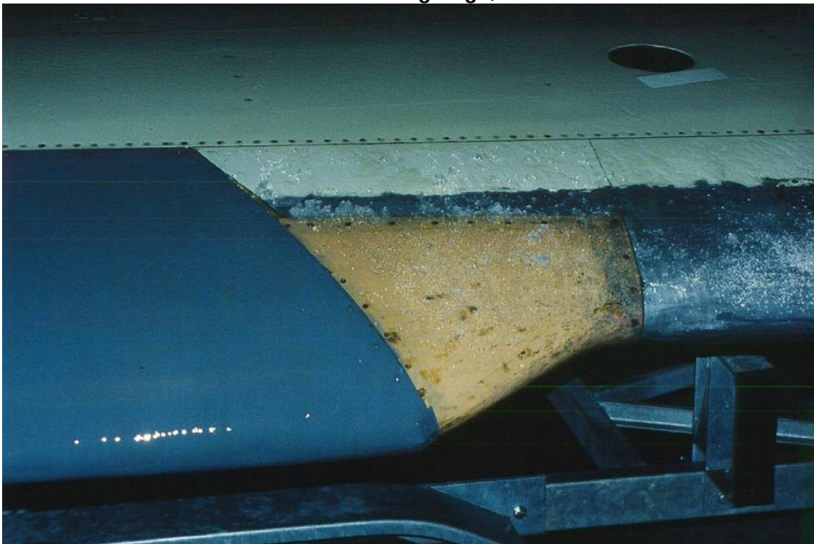
Photo 3.13 Granular Snow on Leading Edge, 10+ mm Thick
