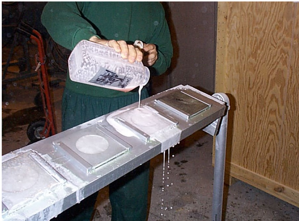
Photo 4.2 Fluid Foam Test
