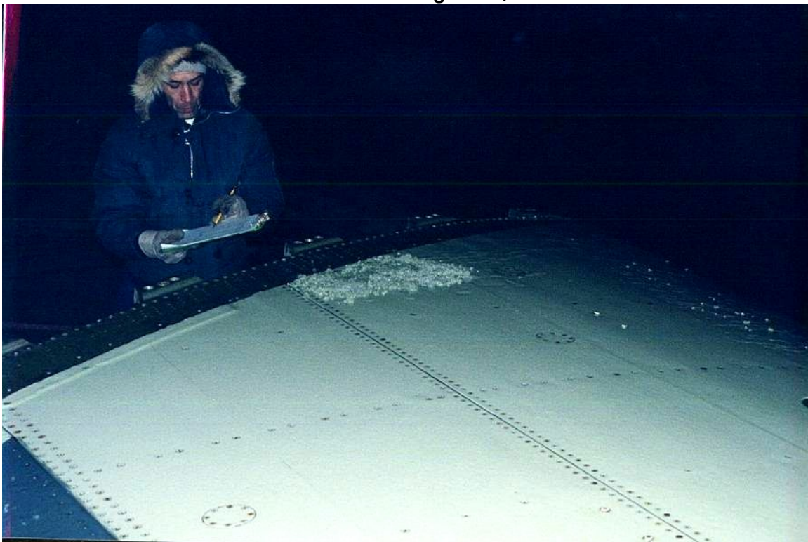
Photo 3.7 Granular Snow Patch at Wing Root, 10+ mm Thick
