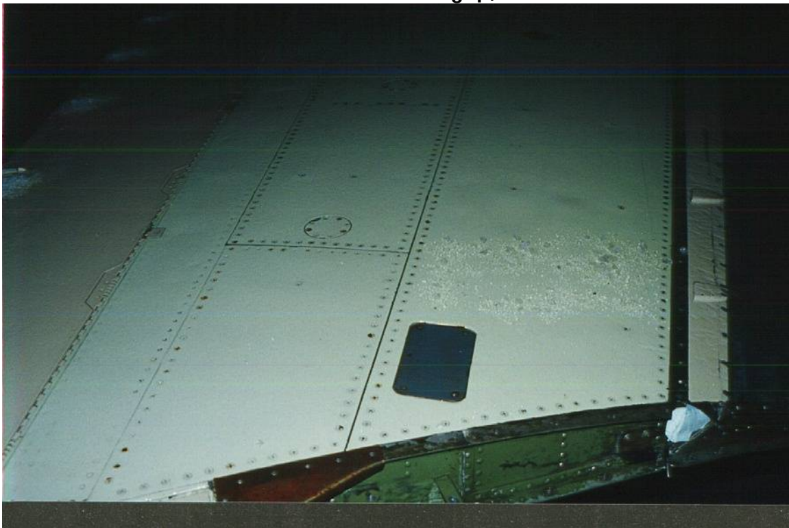
Photo 3.11 Granular Snow Patch Near Wingtip, 10+ mm Thick
