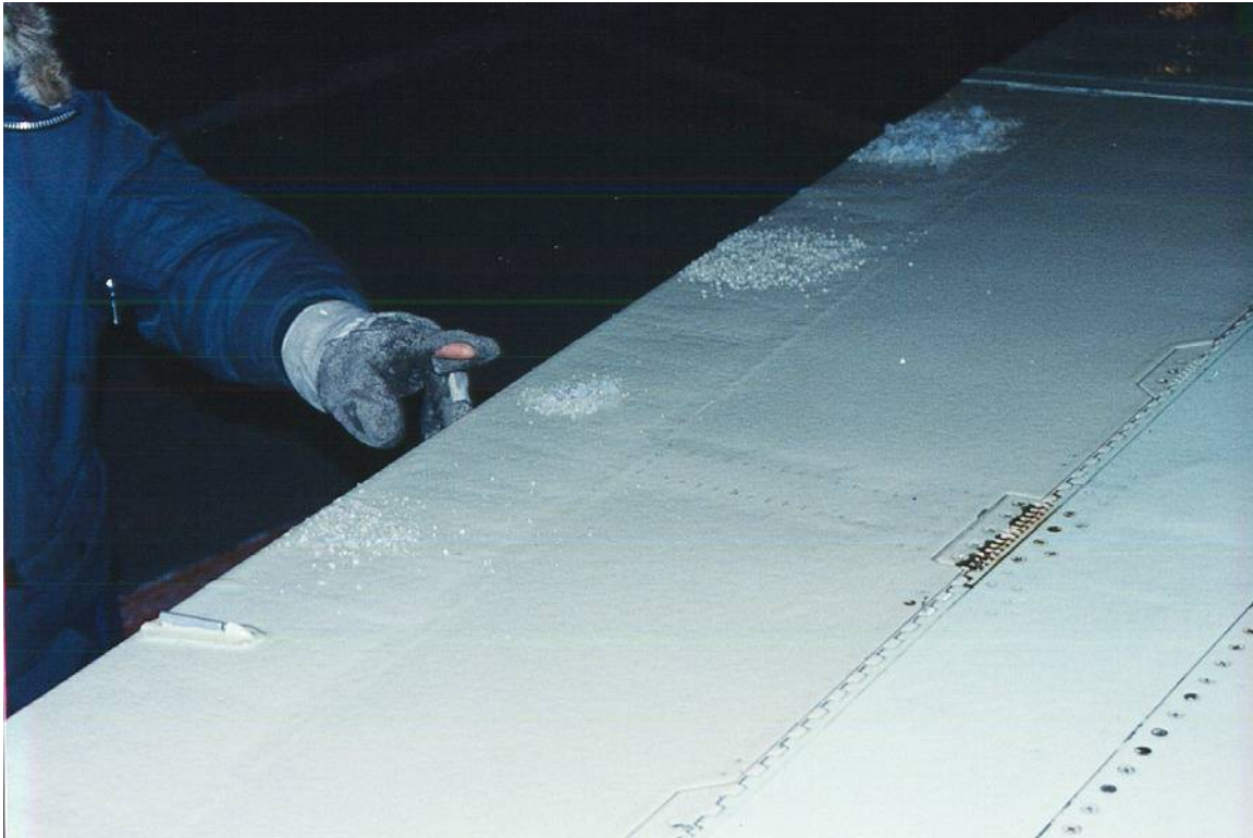
Photo 3.6 Granular Snow Patches on Aileron
