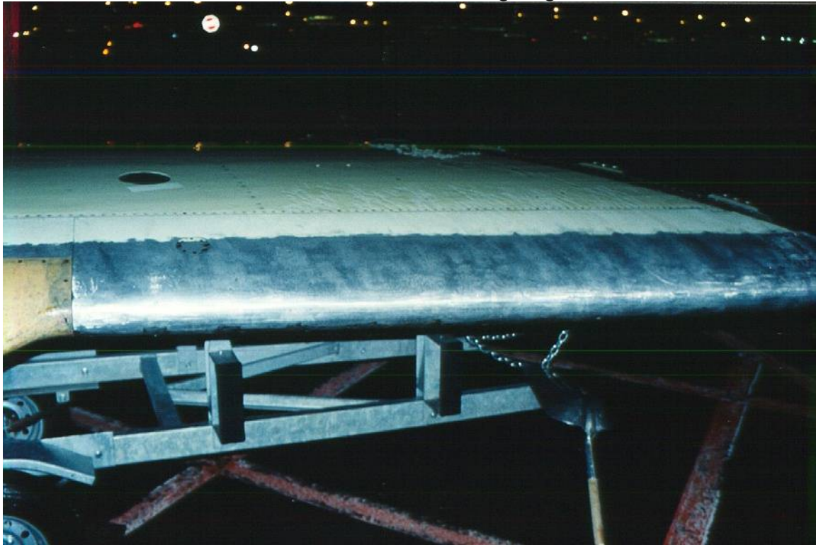
Photo 3.16 Thin Ice Film on Leading Edge
