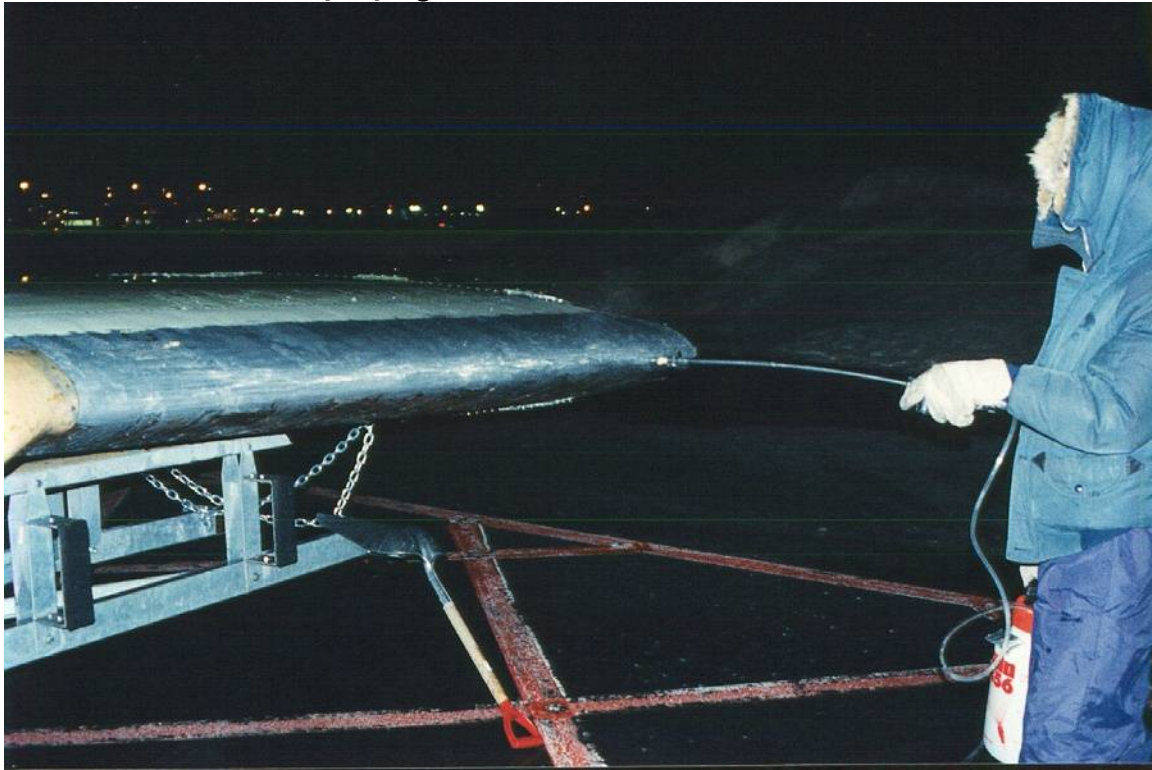
Photo 2.7 Spraying Water Mist to Form Ice Film
