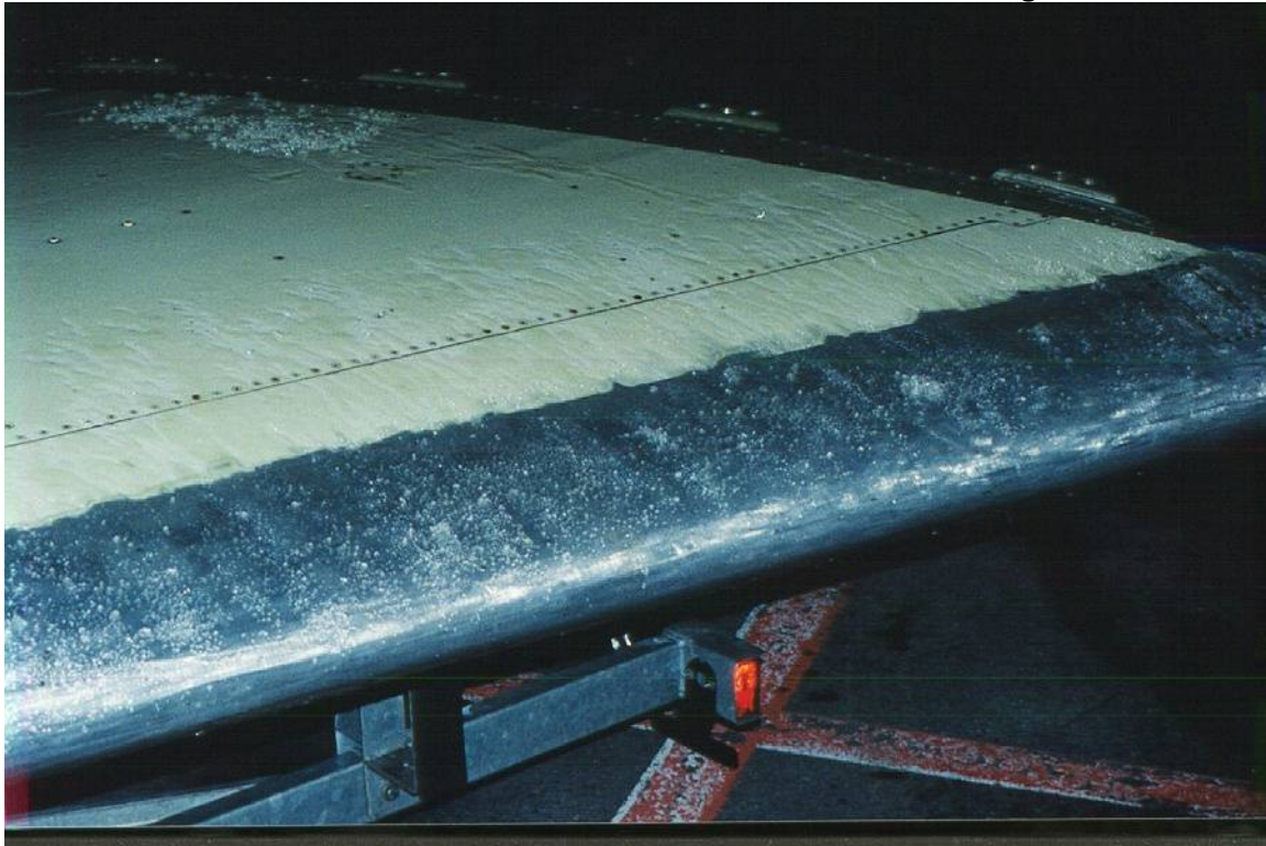
Photo 3.14 Remnants of Granular Snow Patch on Main Wing
