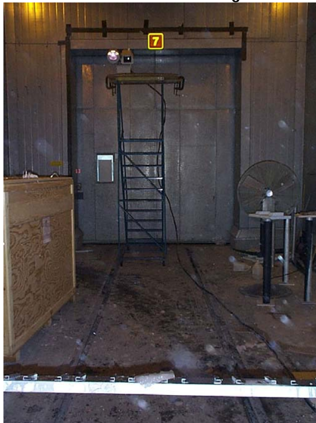
Photo 2.10 Sensor Mounted on Rolling Stair
