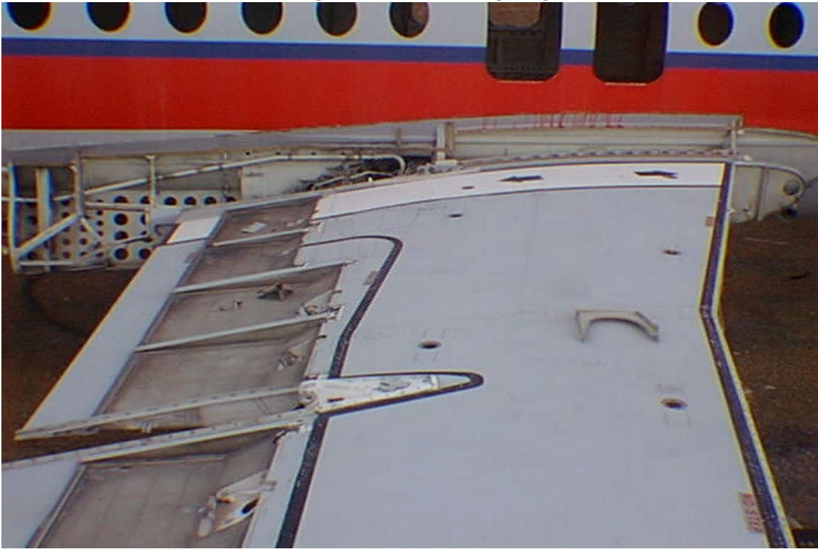
Photo 3.1 Fokker F-28 Starboard Wing Without Leading Edge and Control Surfaces
