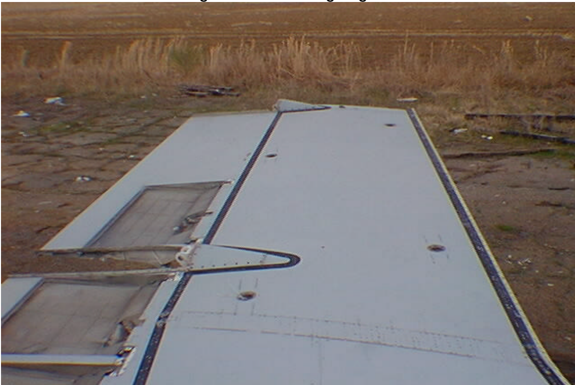
Photo 3.2 Fokker F-28 Port Wing Without Leading Edge and Control Surfaces
