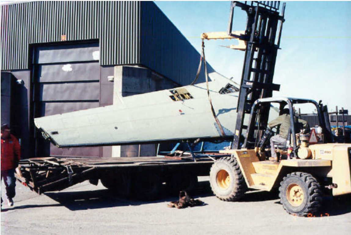
Photo 3.7 Removal of the Wing from the Transportation Vehicle
