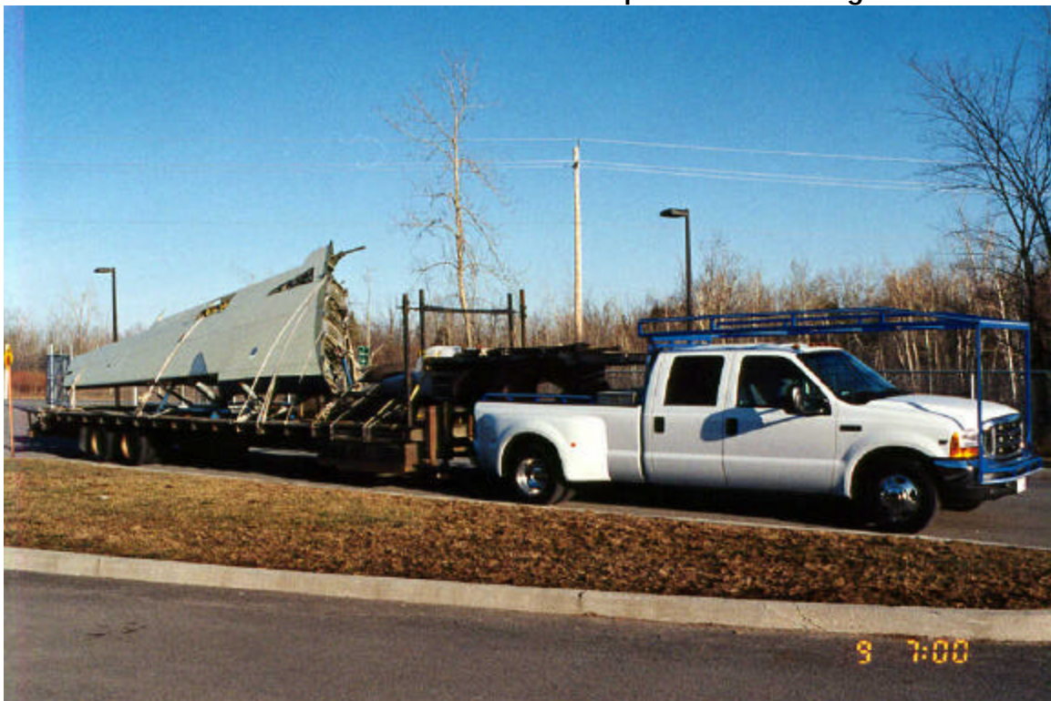
Photo 3.4 Truck and Trailer Used to Transport Jetstar Wing
