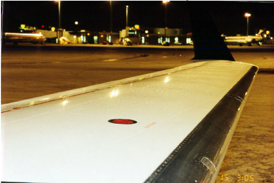
Photo 4.9 Frost Accumulation on the Port Wing (ID# 3)
