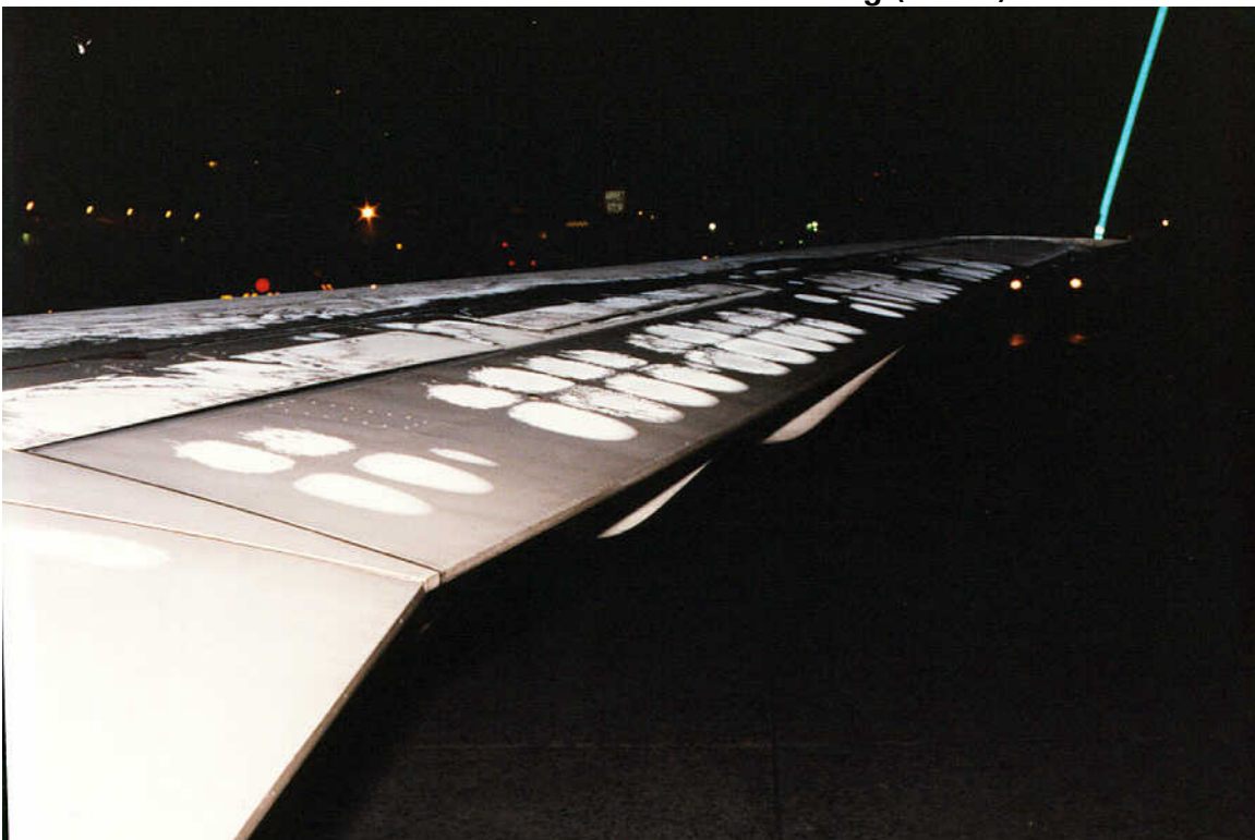
Photo 4.2 Frost Accumulation on Starboard Wing (ID# 1)
