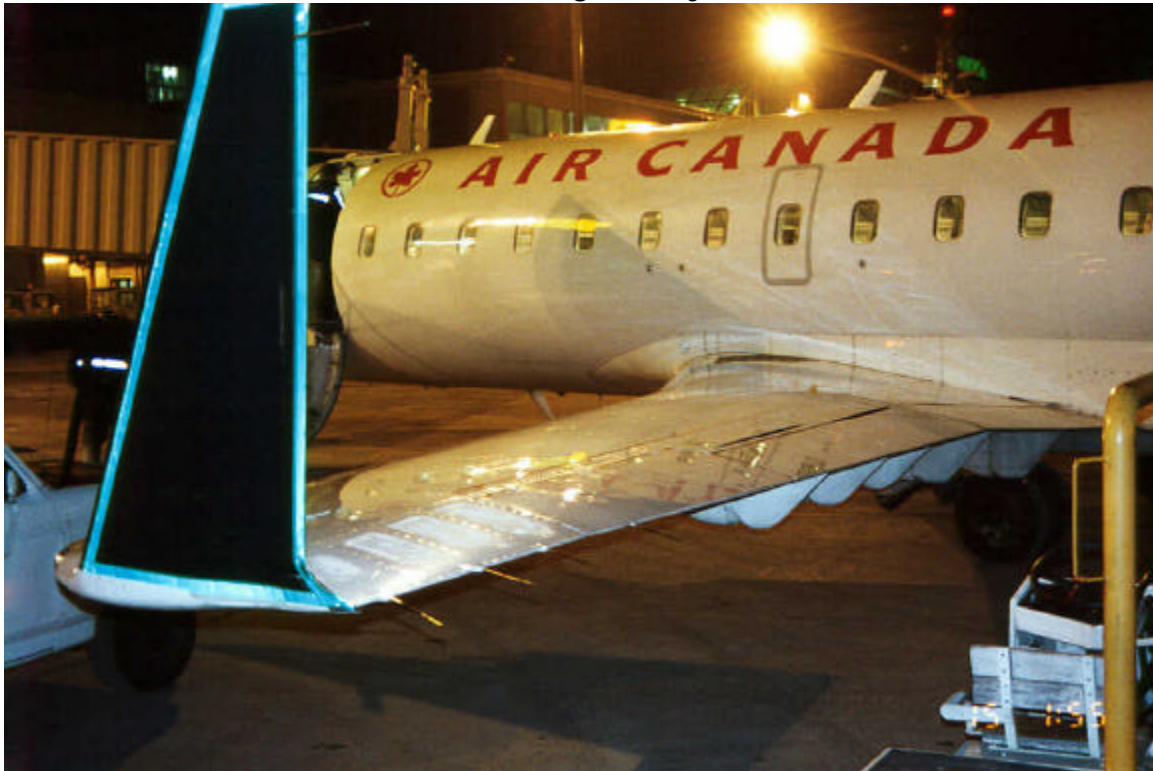
Photo 4.7 Frost Accumulation on Port Wing Shortly After Arrival of Aircraft
