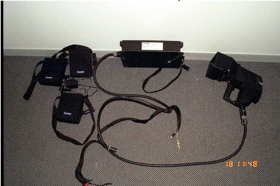
Photo 2.6 Hand-Held Ice Detection Sensor by RVSI ID-1H
