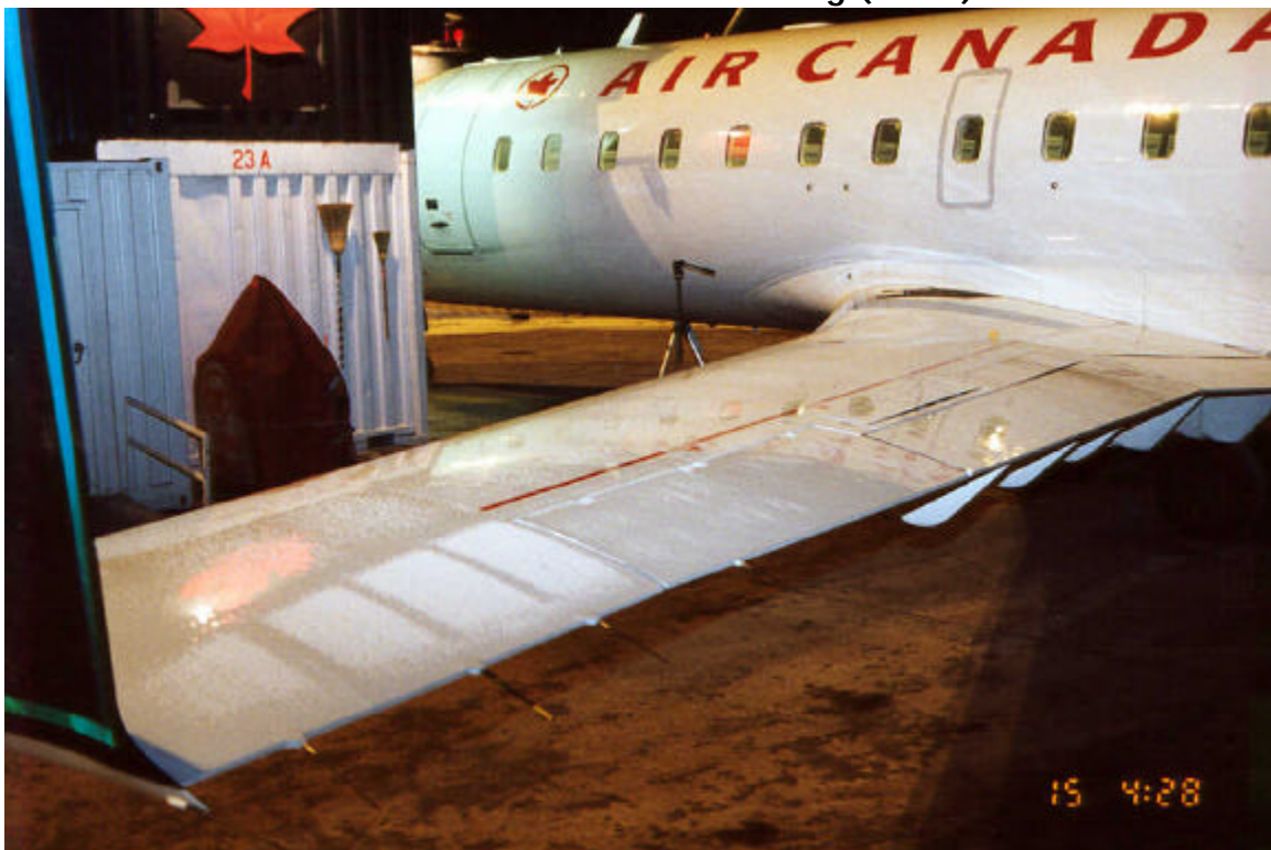
Photo 4.8 Frost Accumulation on Port Wing (ID# 3)
