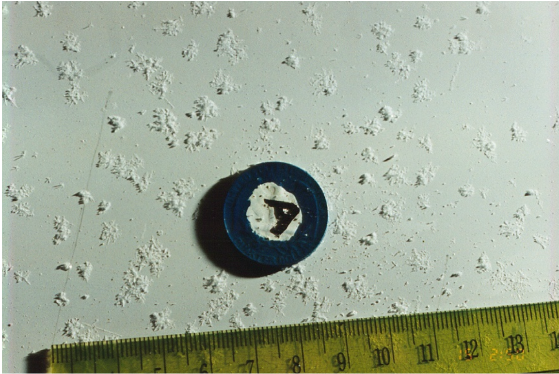
Figure 3.4 Plan Photo of Frost Formation on RJ Aileron
