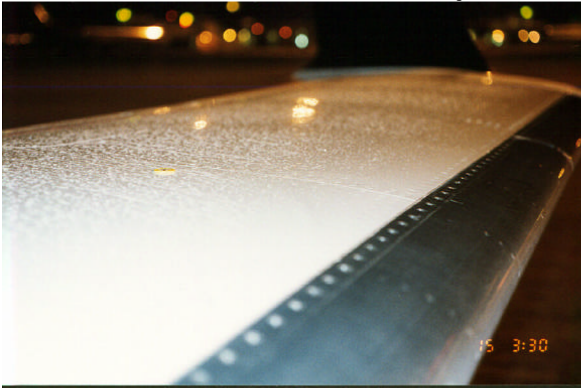
Photo 4.17 Overall Photo of the Frost Formation on the Mid-Wing (ID# 3)
