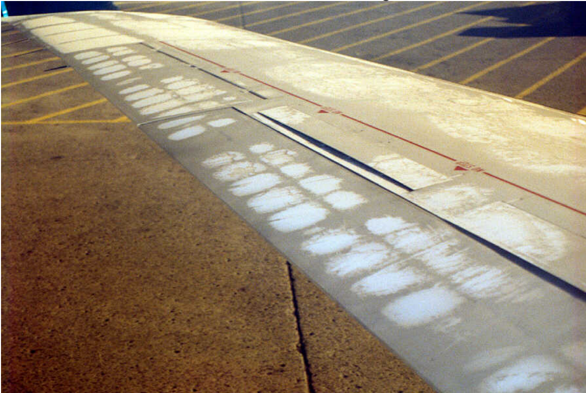
Photo 4.1 Frost Accumulation on Port Wing (ID# 1)
