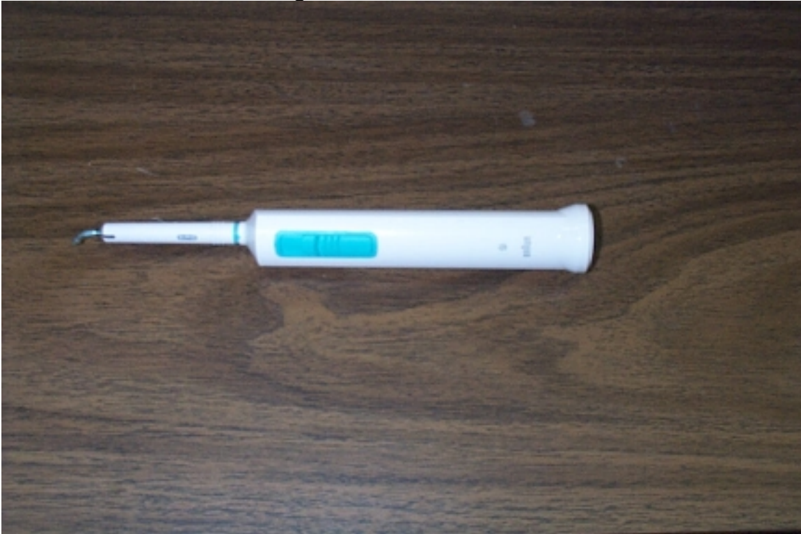
Photo 2.6 Dental Flossing Device Used to Test Adhesion
