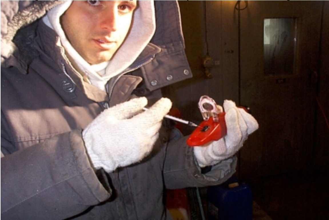
Photo 2.5 Collecting Fluid Samples with Syringe
