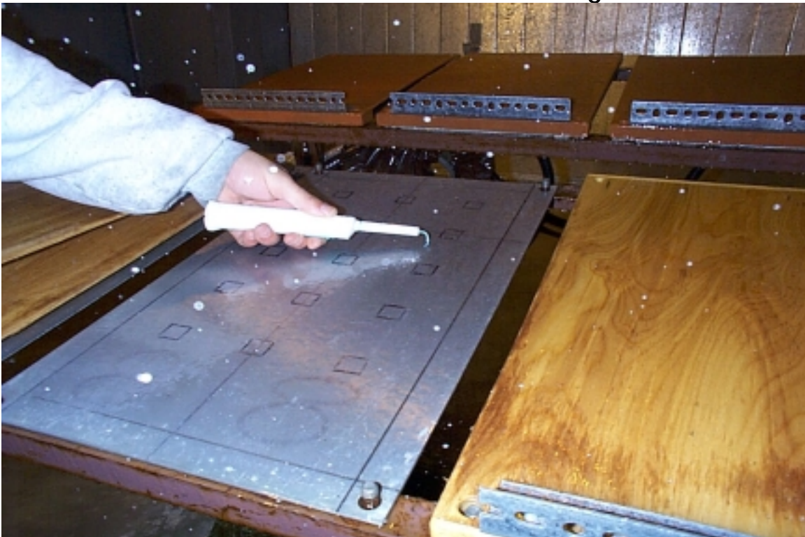
Photo 2.7 Adhesion Tests Performed with Flossing Device
