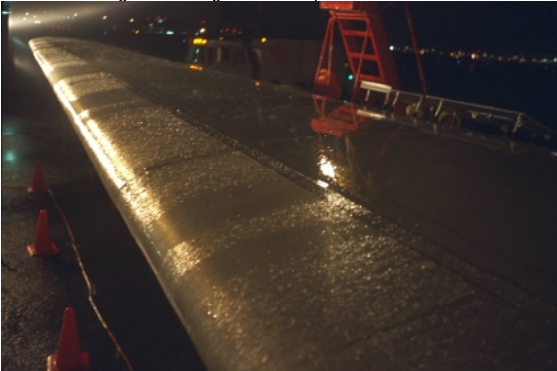
Photo 4.15 TYPE IV FLUID FAILURE ON A DC-9 WING Light Freezing Rain, Temperature = -1^{\circ}\text{C}
