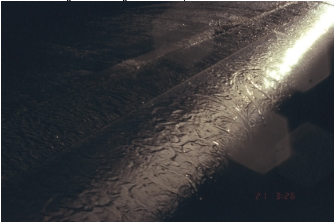
Photo 4.17 TYPE I FLUID FAILURE ON A DC-9 WING Light Freezing Rain, Temperature = -1.5^{\circ}\text{C}
