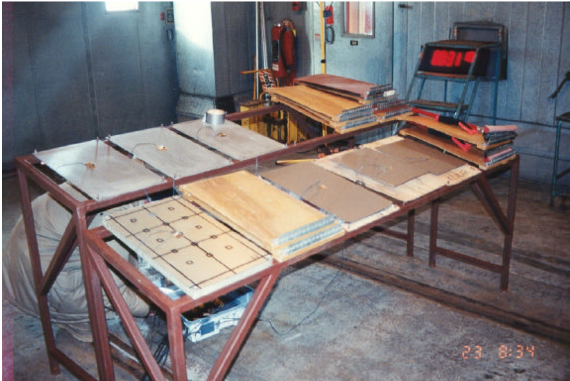
Photo 3.4 Thermistor Probes on Aluminum Plates
