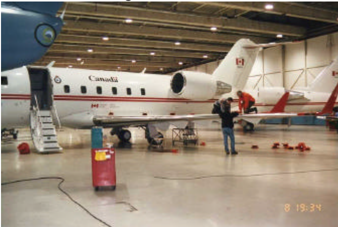
Photo 2.3 Installing Thermistor Probes
