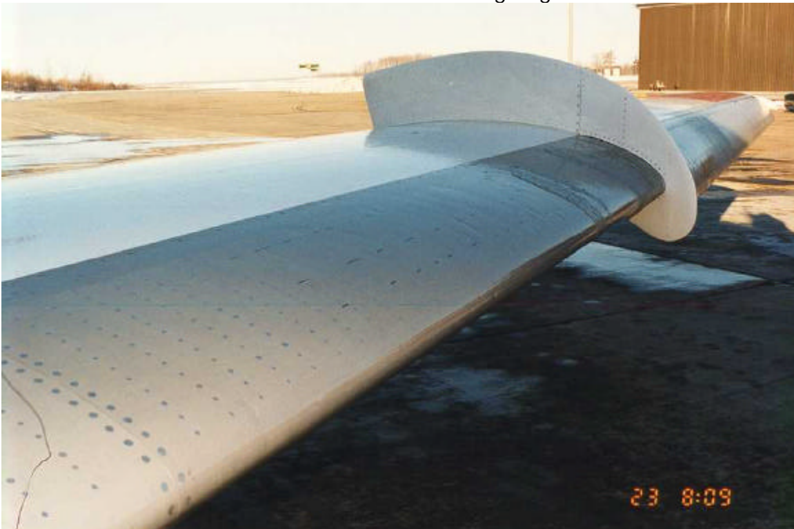
Ice Patches on the Leading Edge
