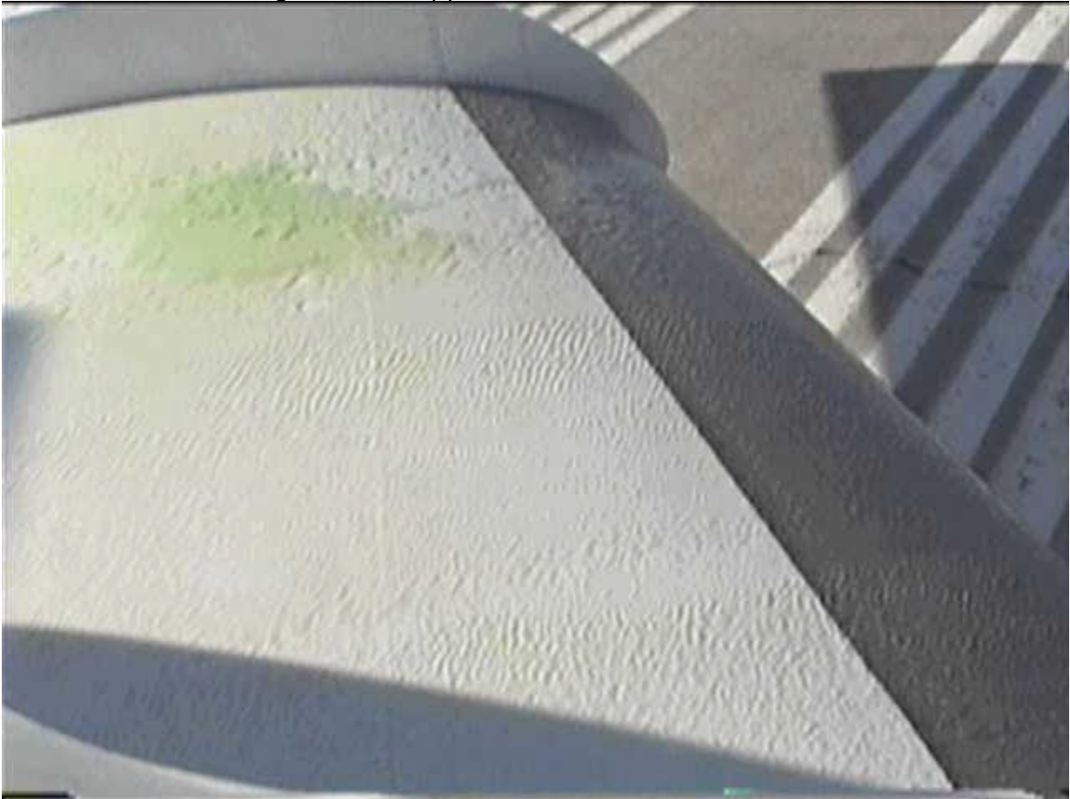
Wing Surface Appearance at End of Taxi Phase
