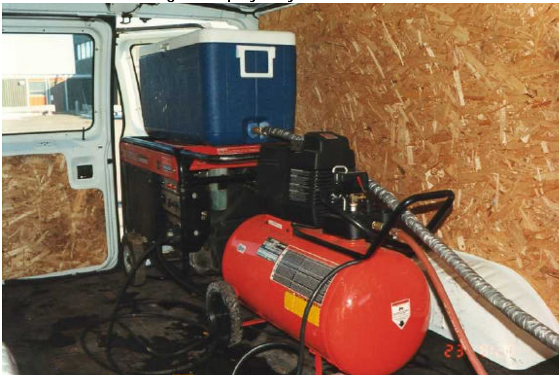
Photo 2.10 Freezing Rain Sprayer System Installed in Van
