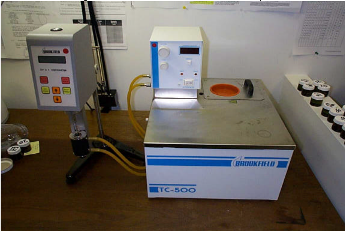
Photo 2.14 Brookfield Digital Viscometer Model DV-I+ and Temperature Bath
