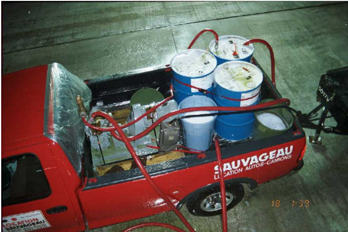
Photo 2.5 Mobile Type IV Fluid Sprayer Unit
