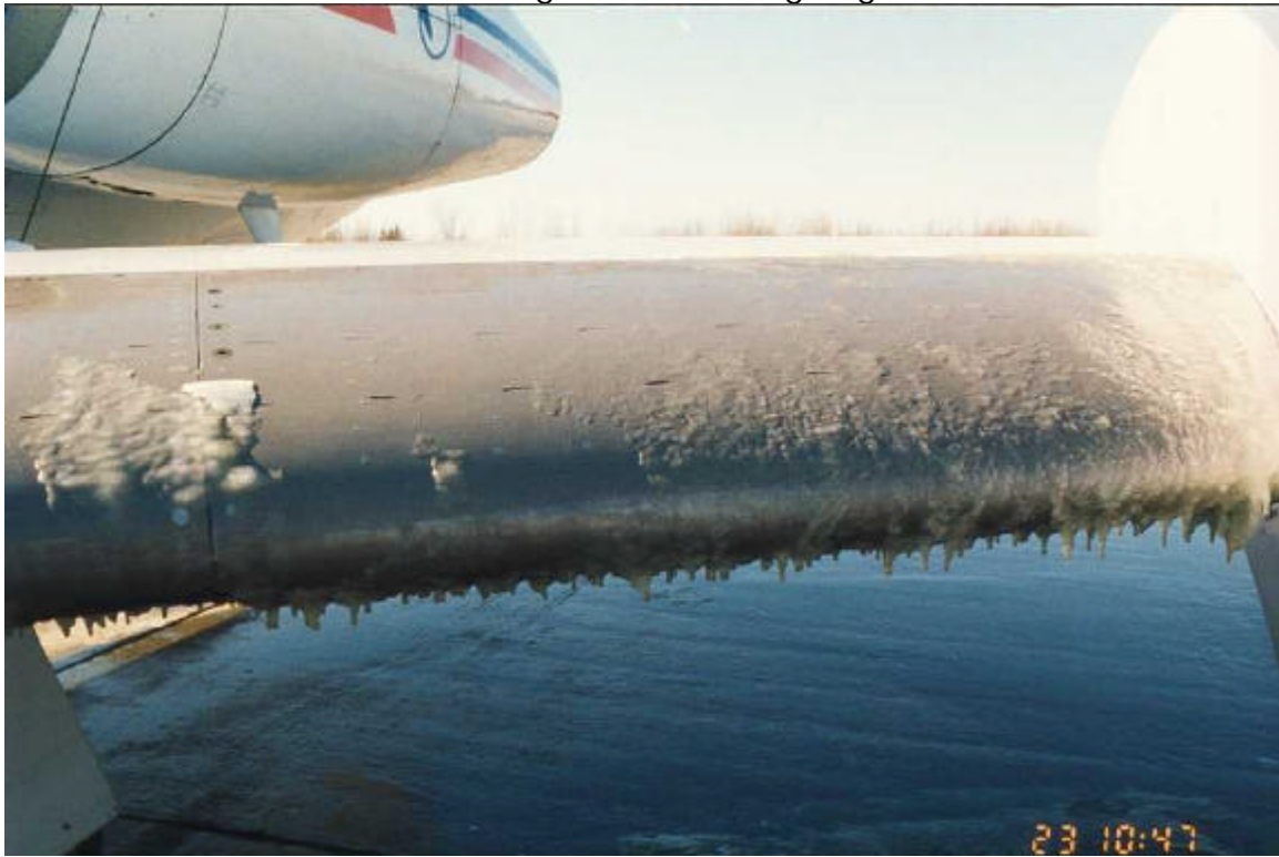
Remaining Ice on Leading Edge
