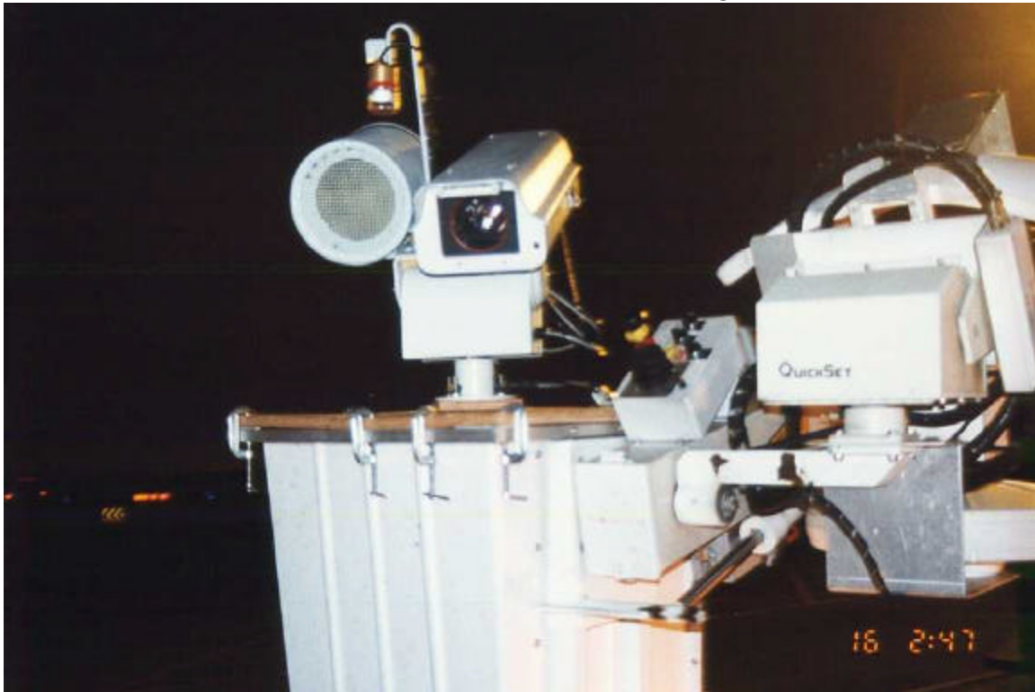
Photo 2.15 Ice Detection Camera Mounting
