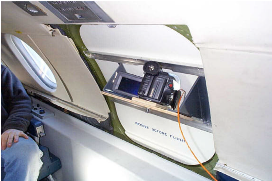
Photo 2.18 Video Camera Installation
