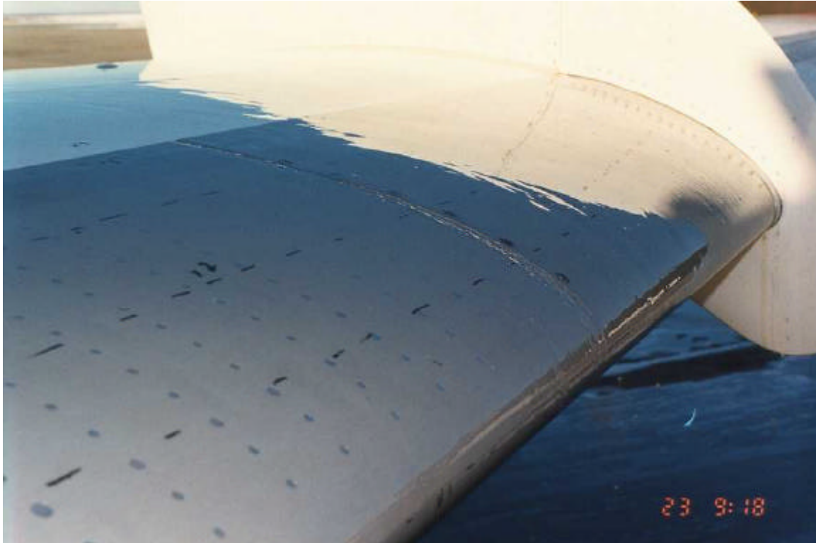
Ice at Seam on Leading Edge
