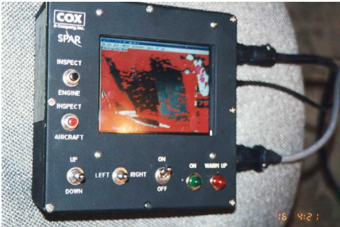
Photo 2.16 Ice Detection Camera Control Unit
