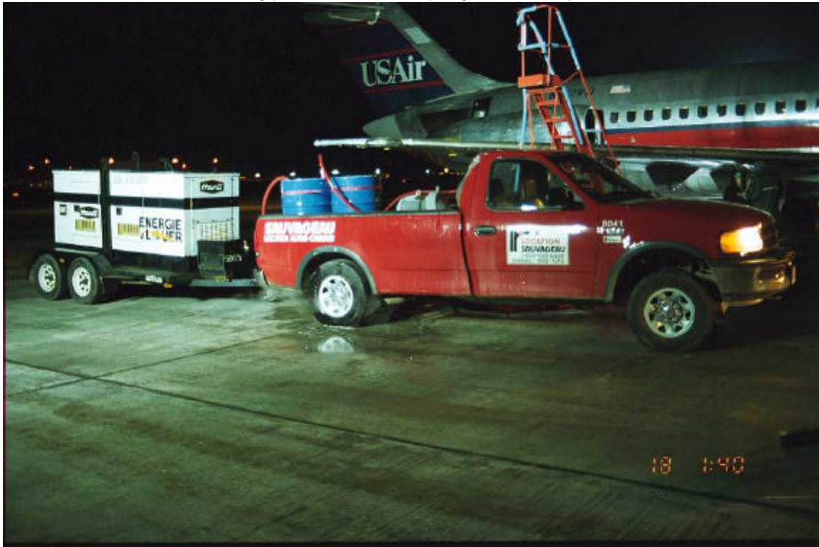
Photo 2.7 Type IV Mobile Sprayer Set-Up
