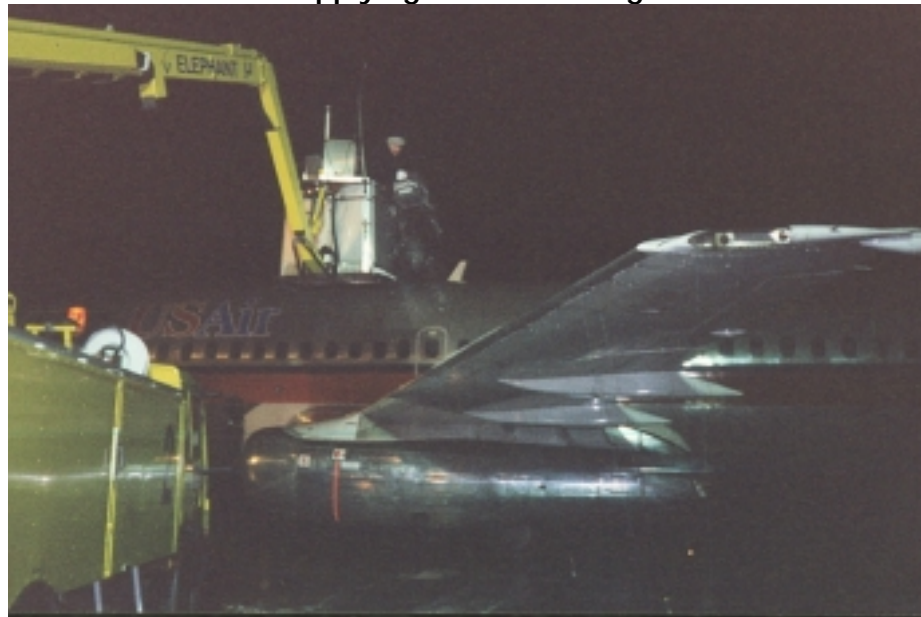
Photo 2.24 Applying Snow to Wing
