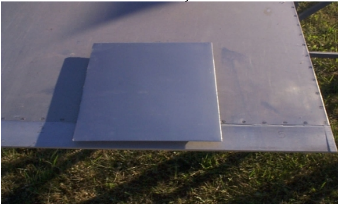
Photo 2.18 Carbon Fibre on Honeycomb Surface
