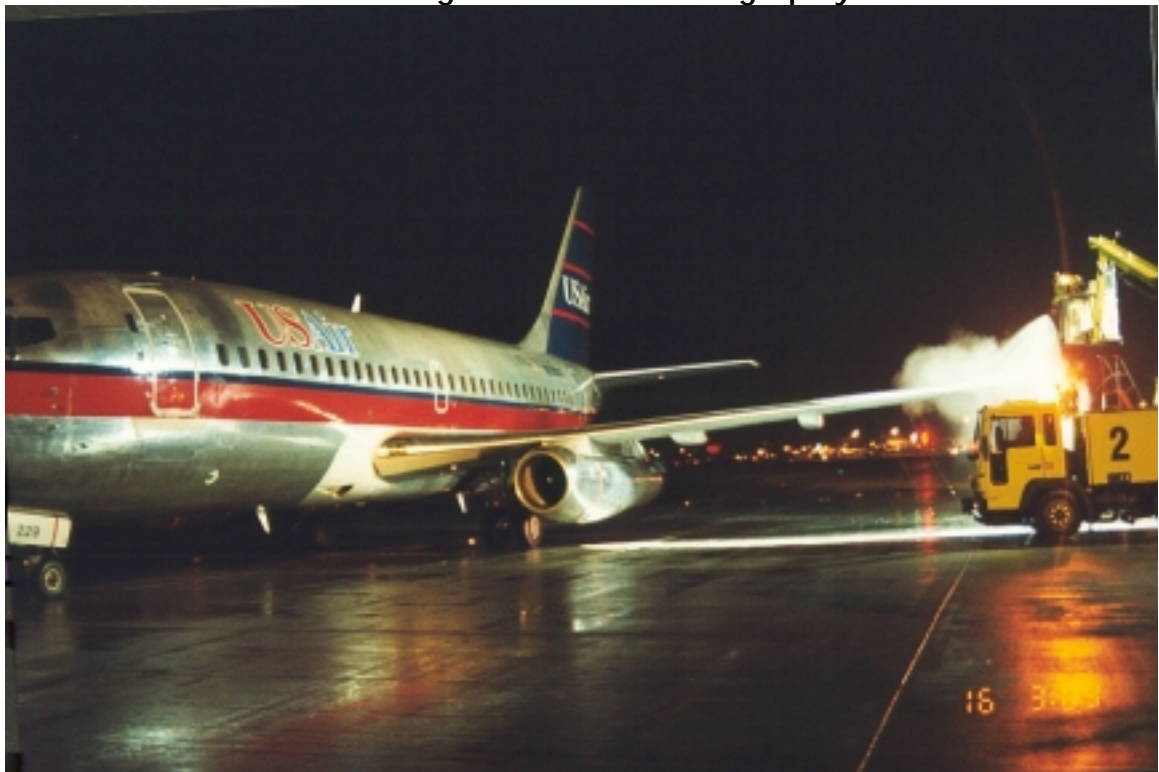
Photo 2.26 Removing Snow with De-icing Spray
