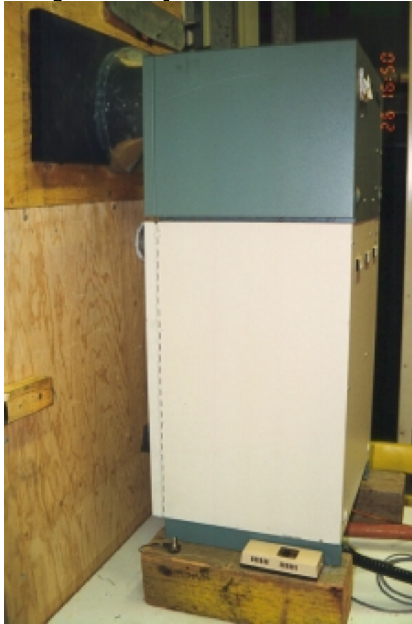
Photo 2.23 High Humidity via Steam Generator
