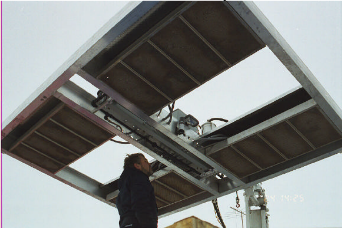
Photo 2.1 Underside of Heater Array
