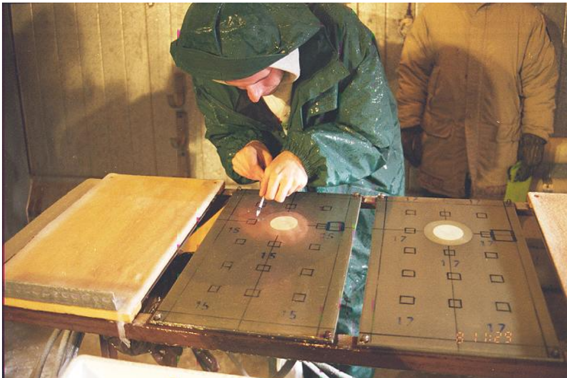
Photo 2.4 Collecting Fluid Samples with Syringe
