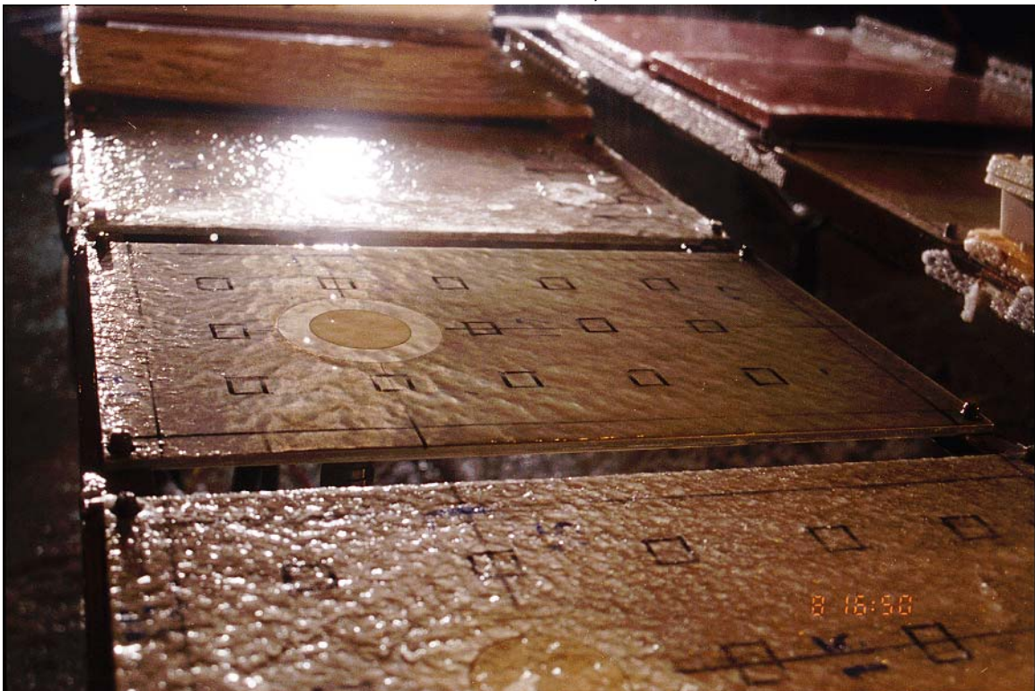
Photo C11.2 - 1 st Failure, t = 13 min
