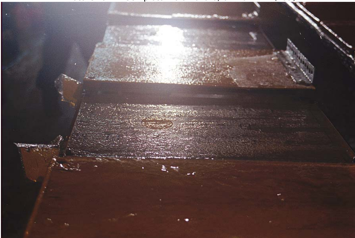
Photo C20.4 - Complete Fluid Failure, t = 64 min (Est.)
