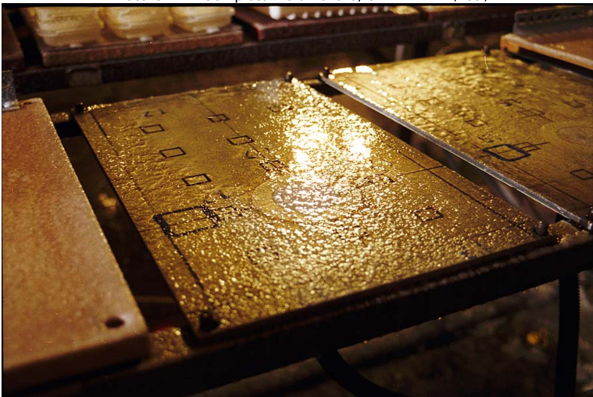
Photo C2.4 - Complete Fluid Failure, t = 44 min (Est.)
