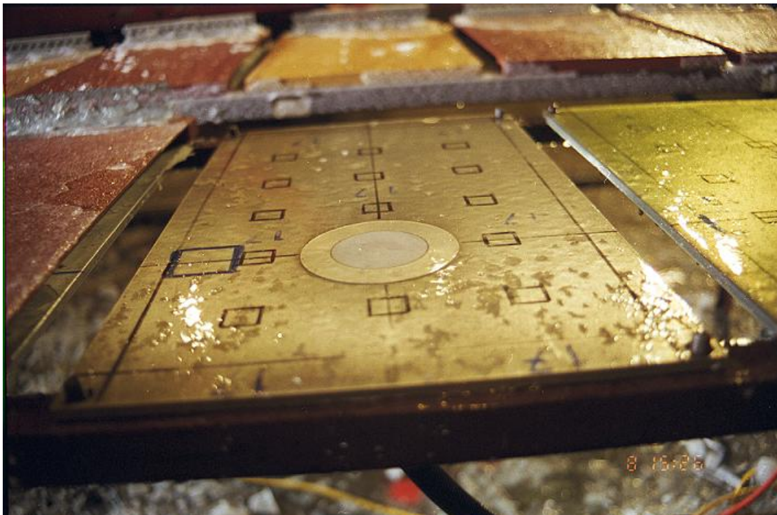
Photo 4.4 Streaks of Solidified Precipitation
