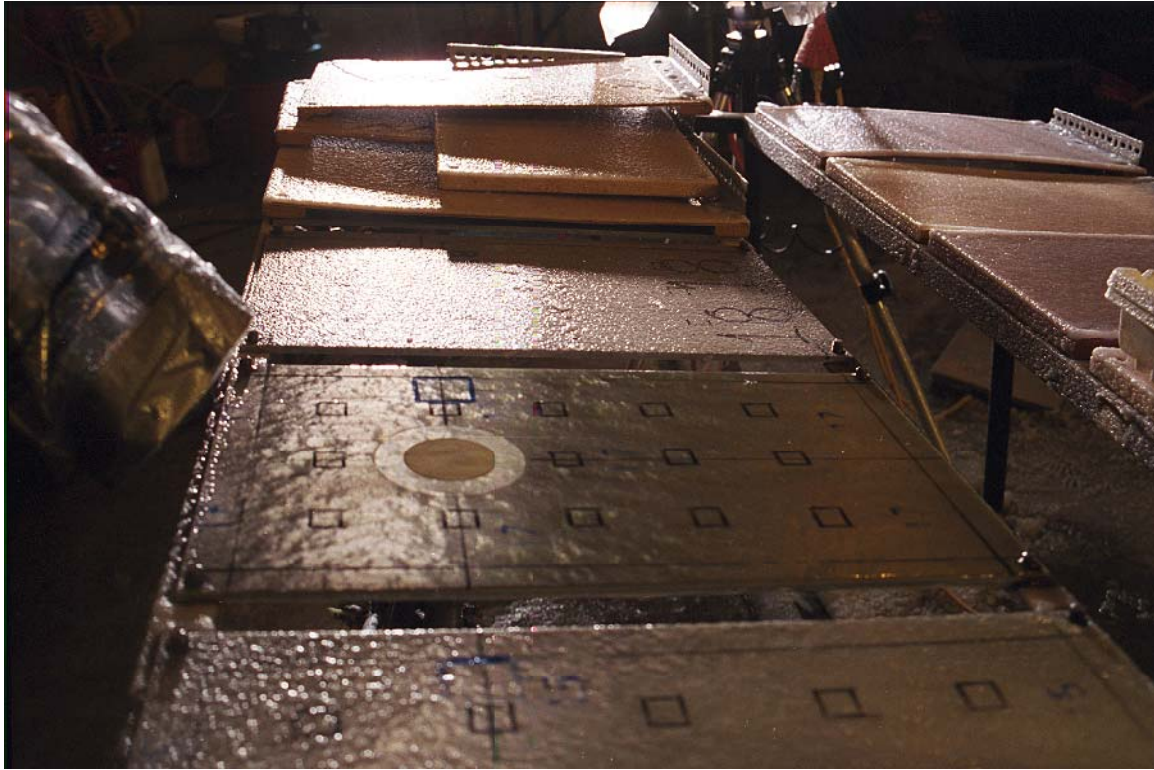
Photo 4.9 Fingers of Plate-like Ice Particles
