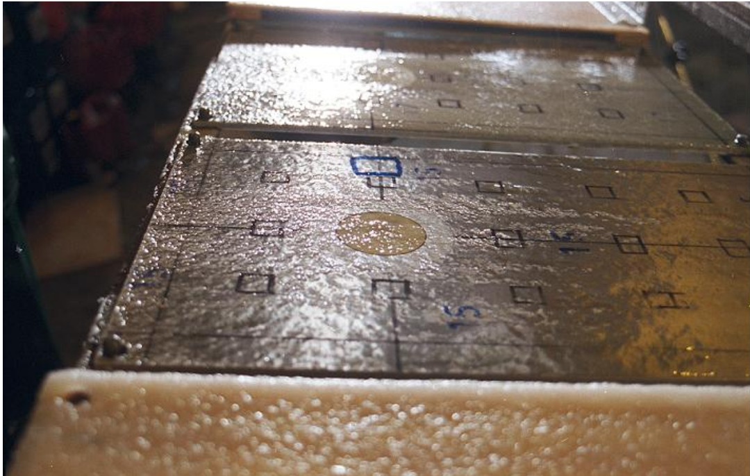
Photo 3.4 PHOTOS OF COMPLETE FAILURE - ID # 1 Complete Fluid Failure, t = 66 min (Est,)
