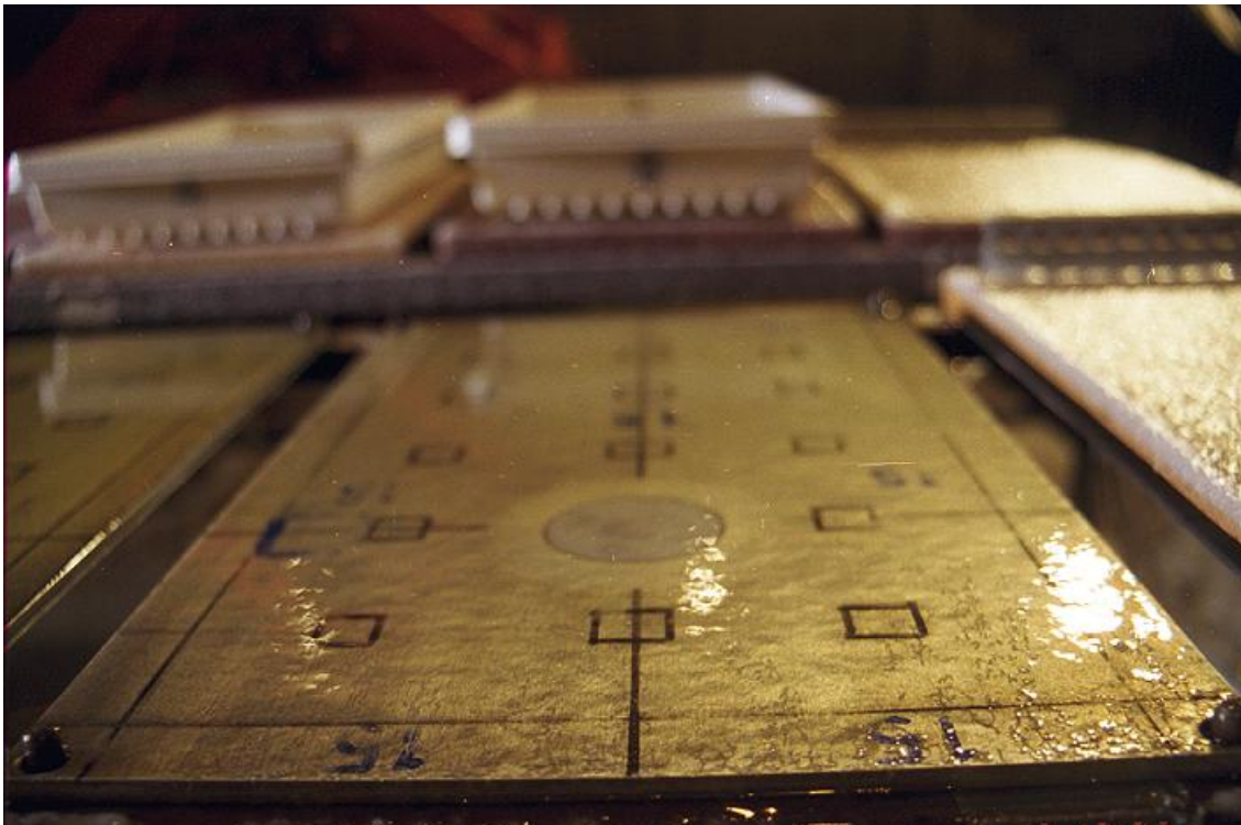
Photo 4.8 Dots and Streaks of Solidified Precipitation
