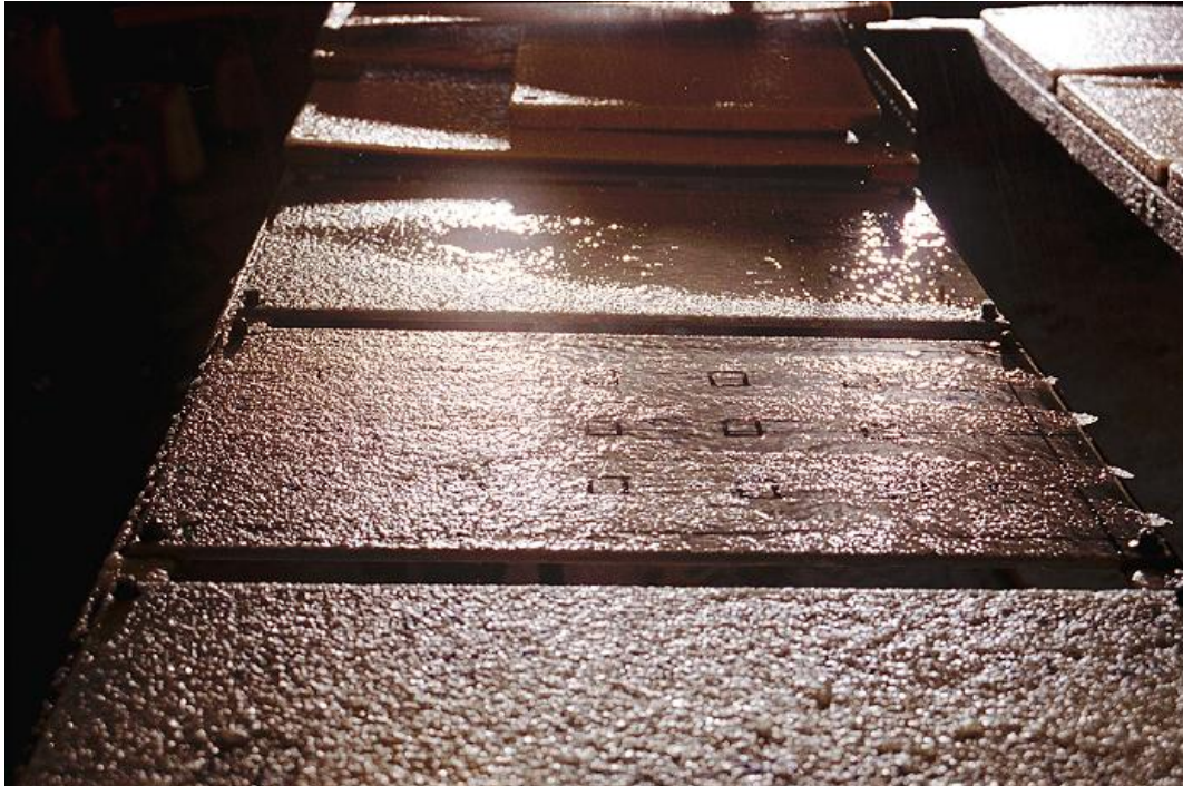
Photo 4.18 TYPE IV FLUID FAILURE – FREEZING DRIZZLE Temperature = -10^{\circ}\text{C} , Precip. Rate = 10\text{ g/dm}^2/\text{h}
