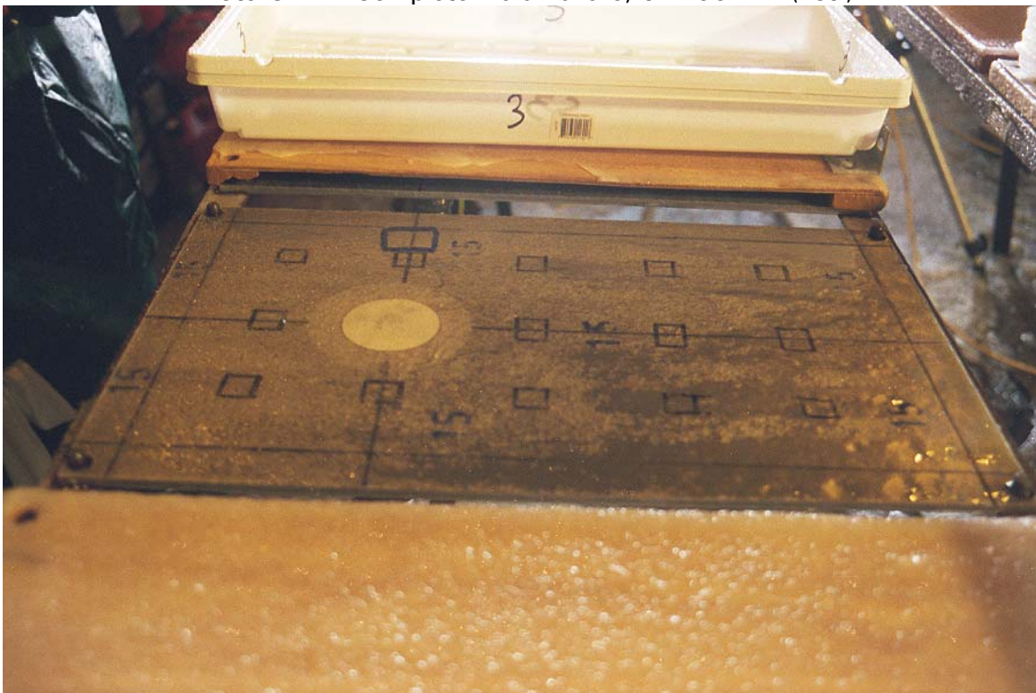
Photo C1.4 - Complete Fluid Failure, t = 66 min (Est.)
