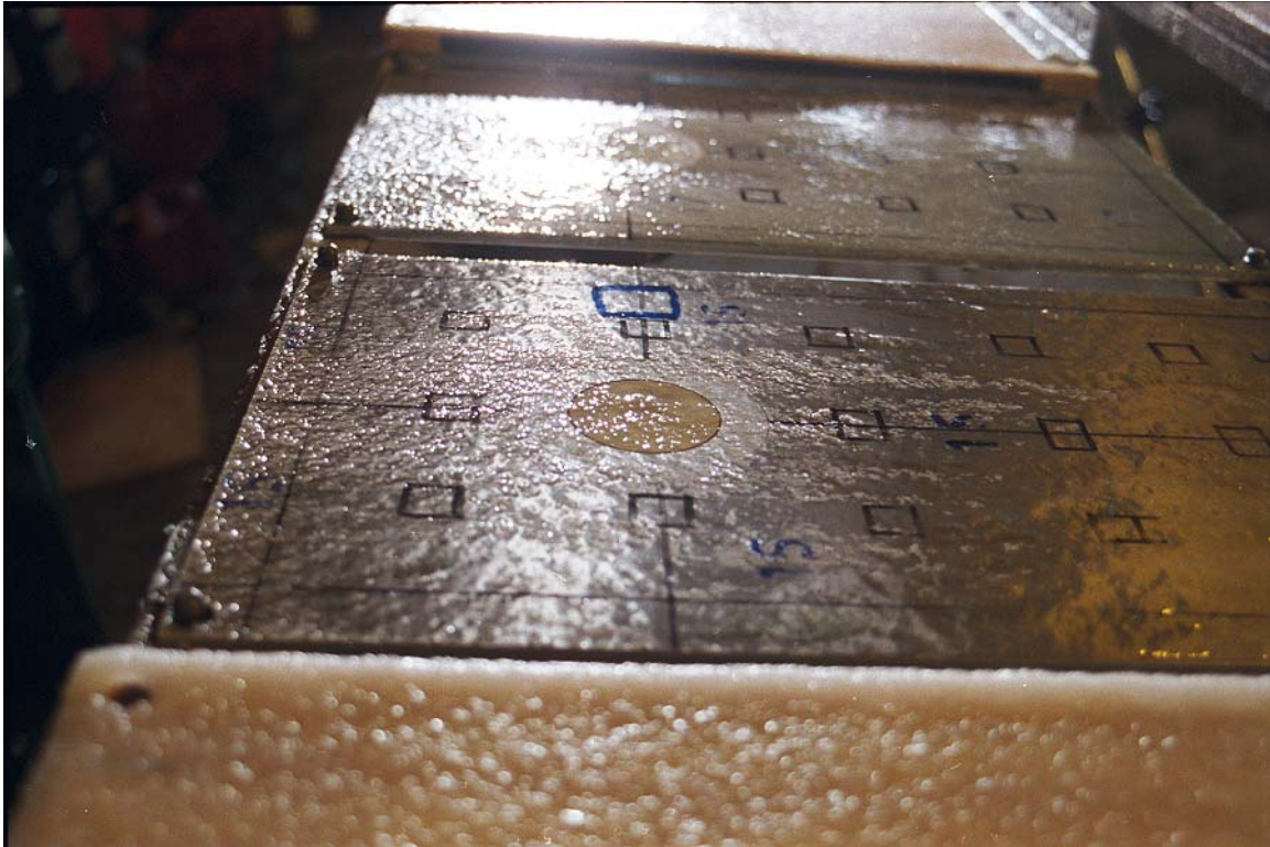
Photo C1.3 - Standard Failure (1/3 or 5 th Crosshair), t = 50 min (Est.)
