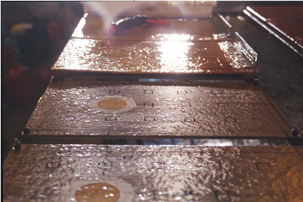
Photo C15.4 - Complete Fluid Failure, t = 18 min
