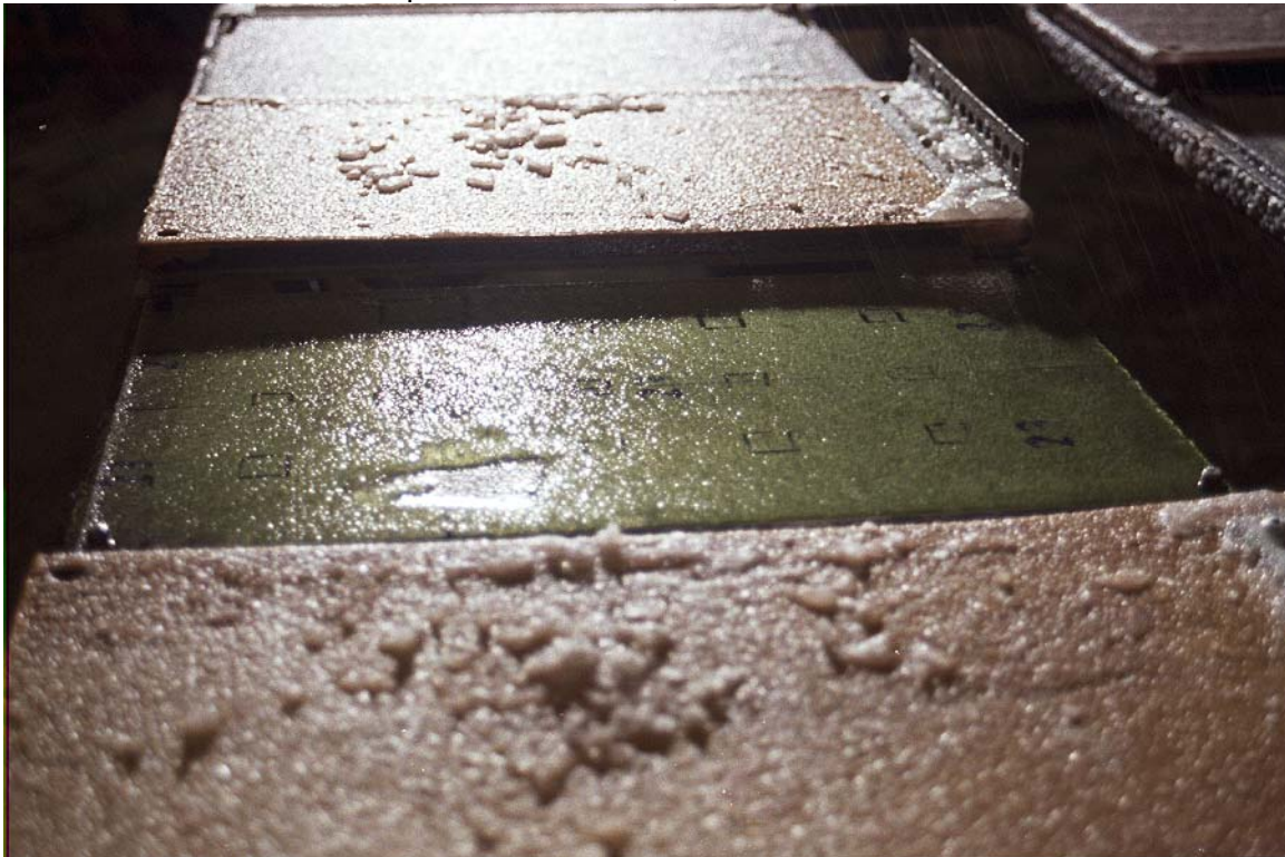
Complete Fluid Failure, t = 79 min (Est.)
