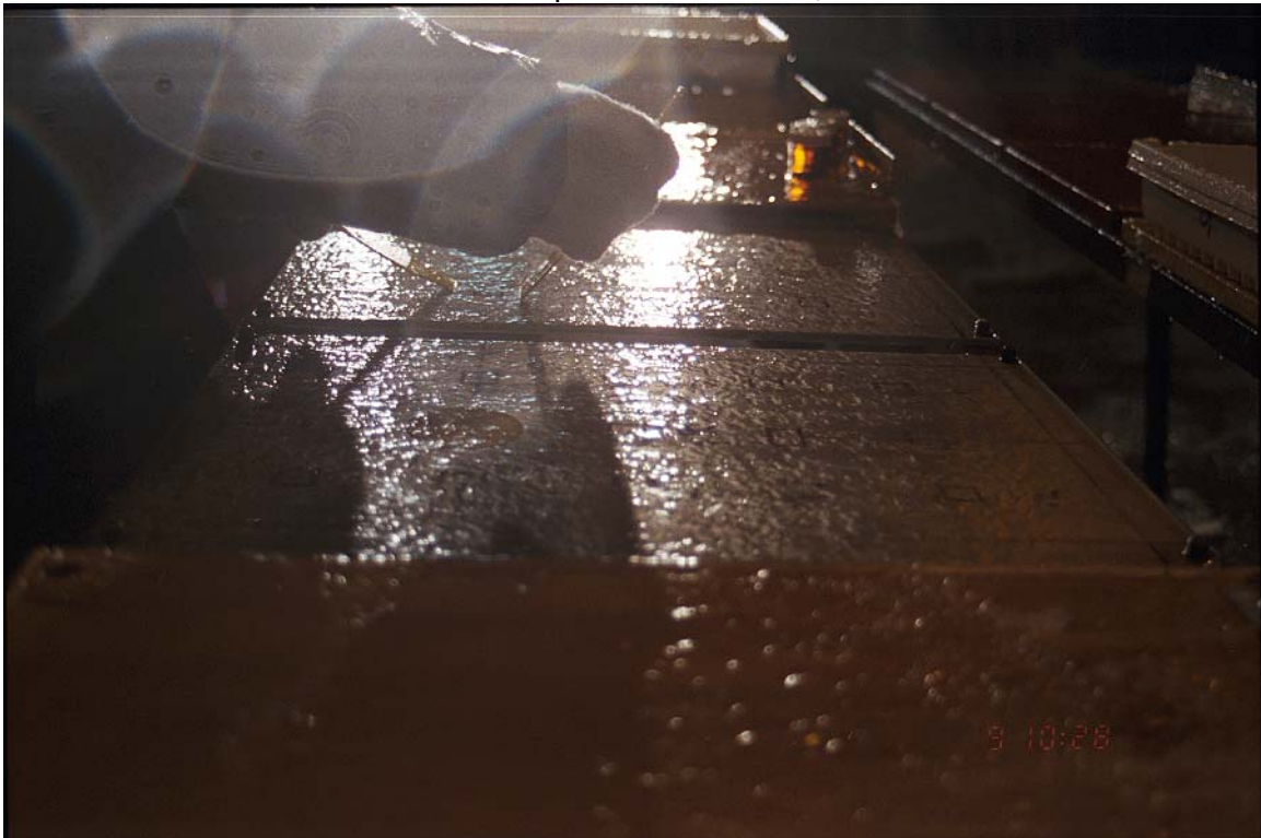
Photo C16.4 - Complete Fluid Failure, t = 25 min
