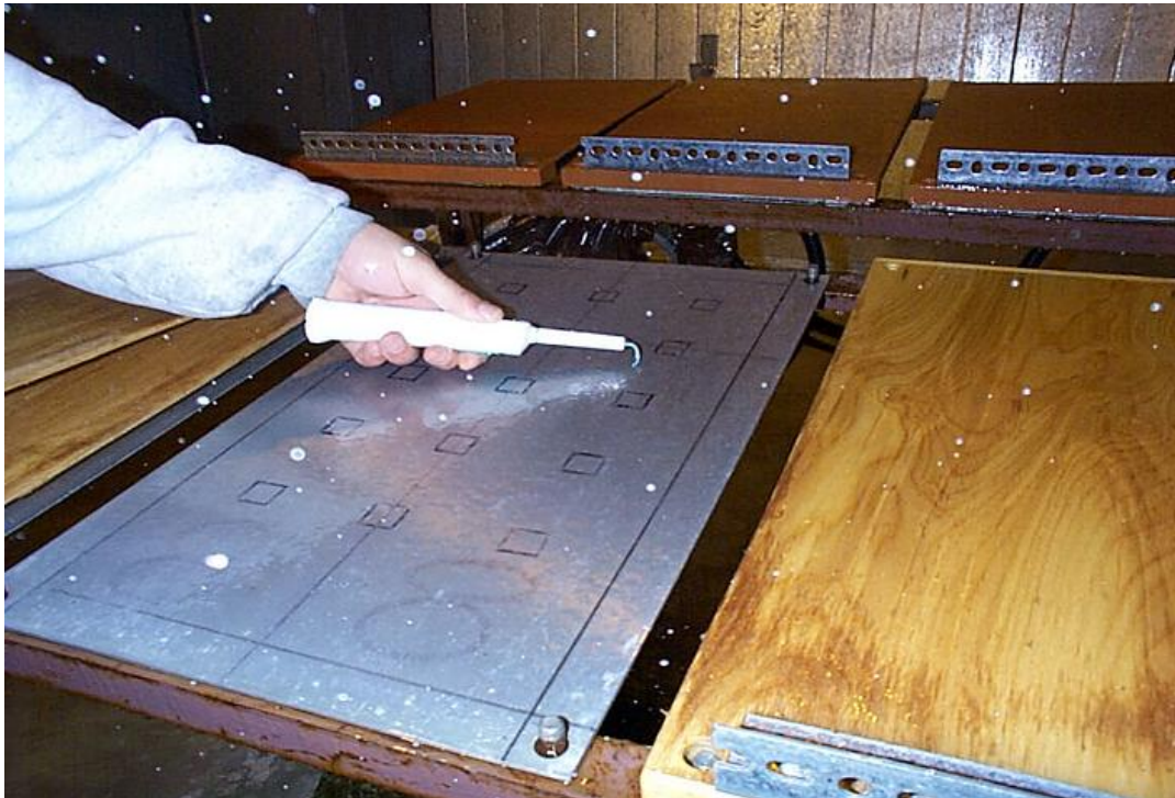
Photo 2.6 Testing Adherence with Flossing Device
