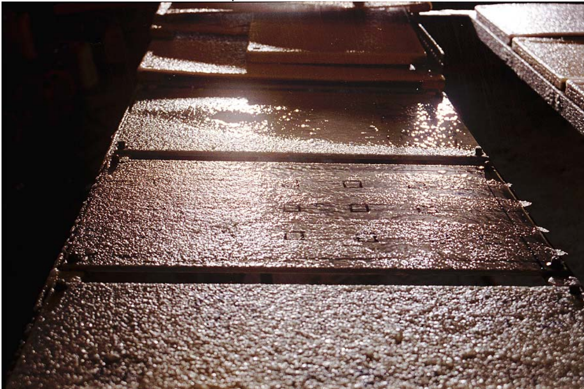
Photo C4.4 - Complete Fluid Failure, t = 81 min (Est.)
