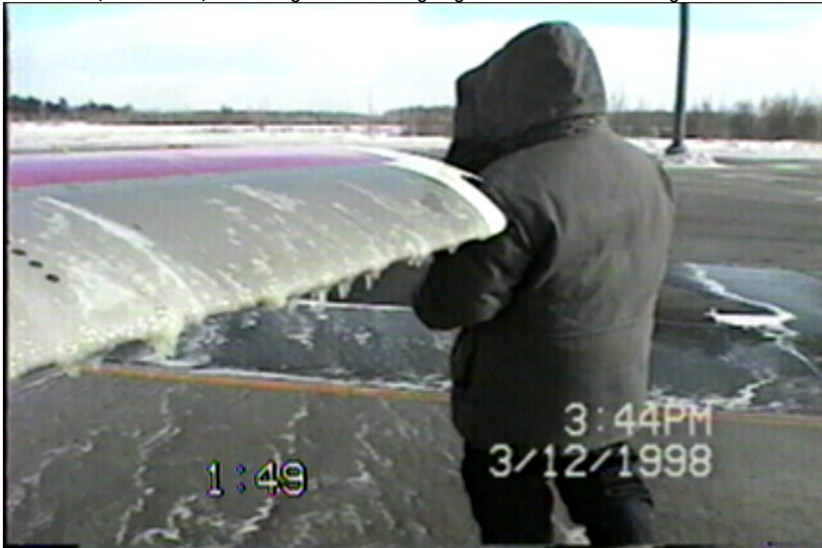
Run 3 (33% Failure) Remaining Ice on Leading Edge Outer Chord - Following Takeoff Run
