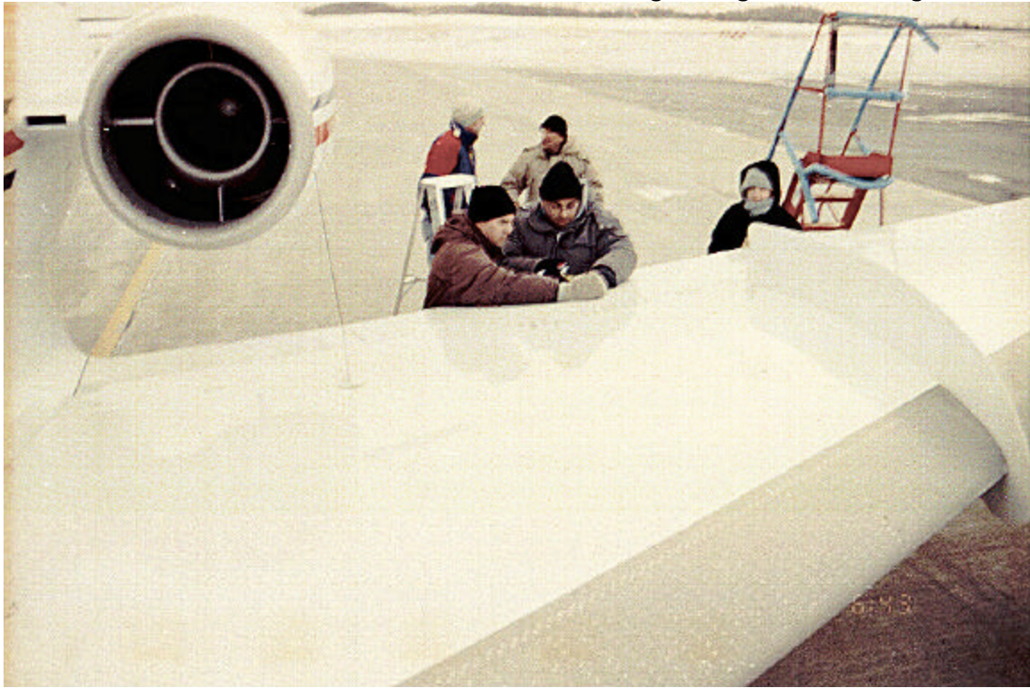
Photo 2.5 NRC Falcon 20D Fluid Thickness Measuring (Wing Fence at Right)
