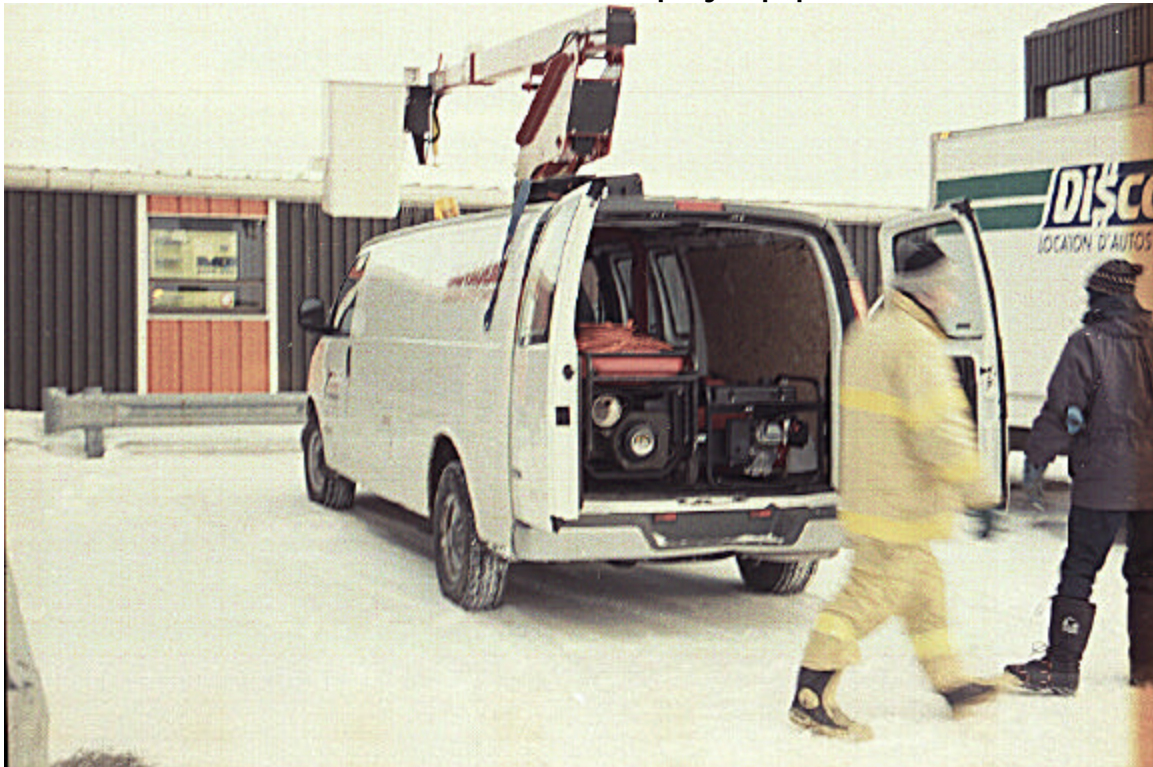
Photo 2.6 Boom Truck with Water Spray Equipment
