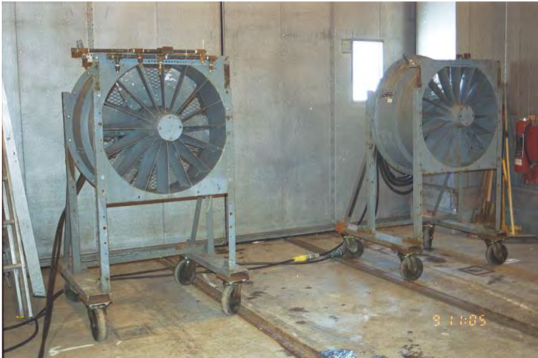
Photo 2.10 Fans Used to Generate Winds
