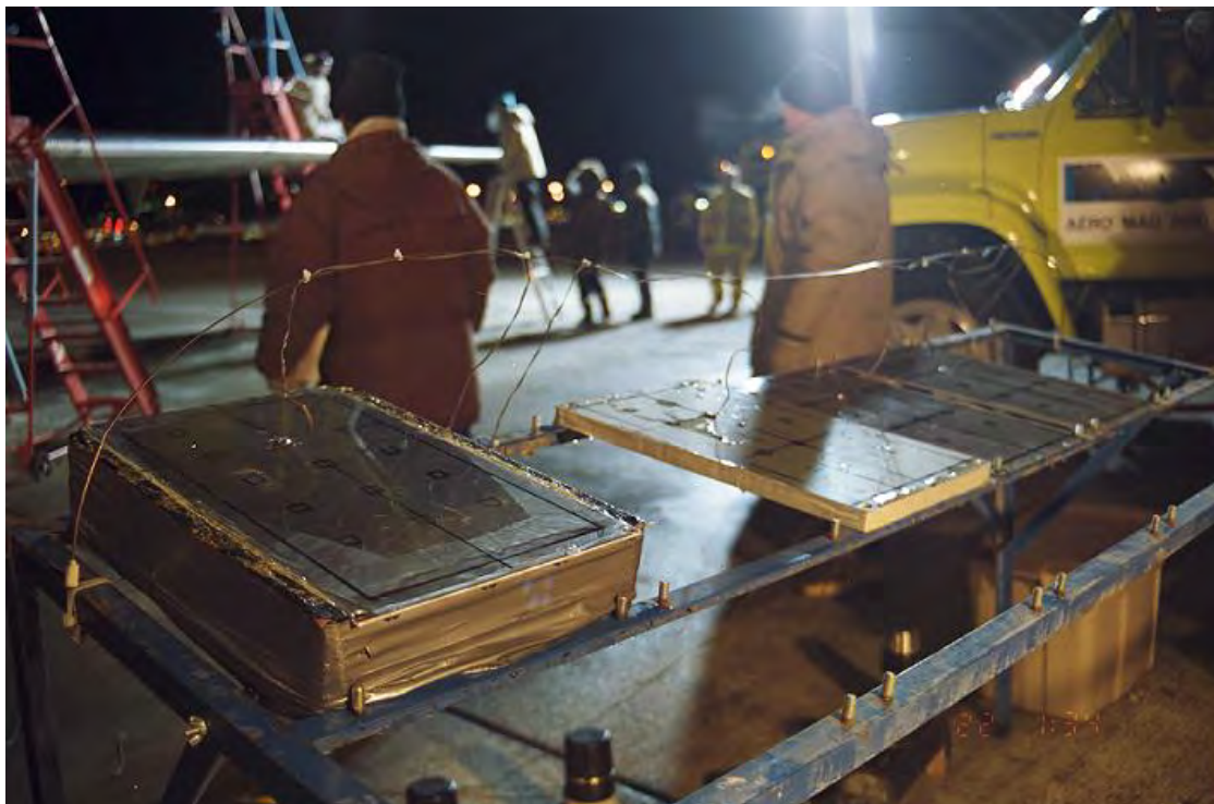
Photo 2.4 Typical Installation of Thermistor Probes on Cold-Soaked Boxes
