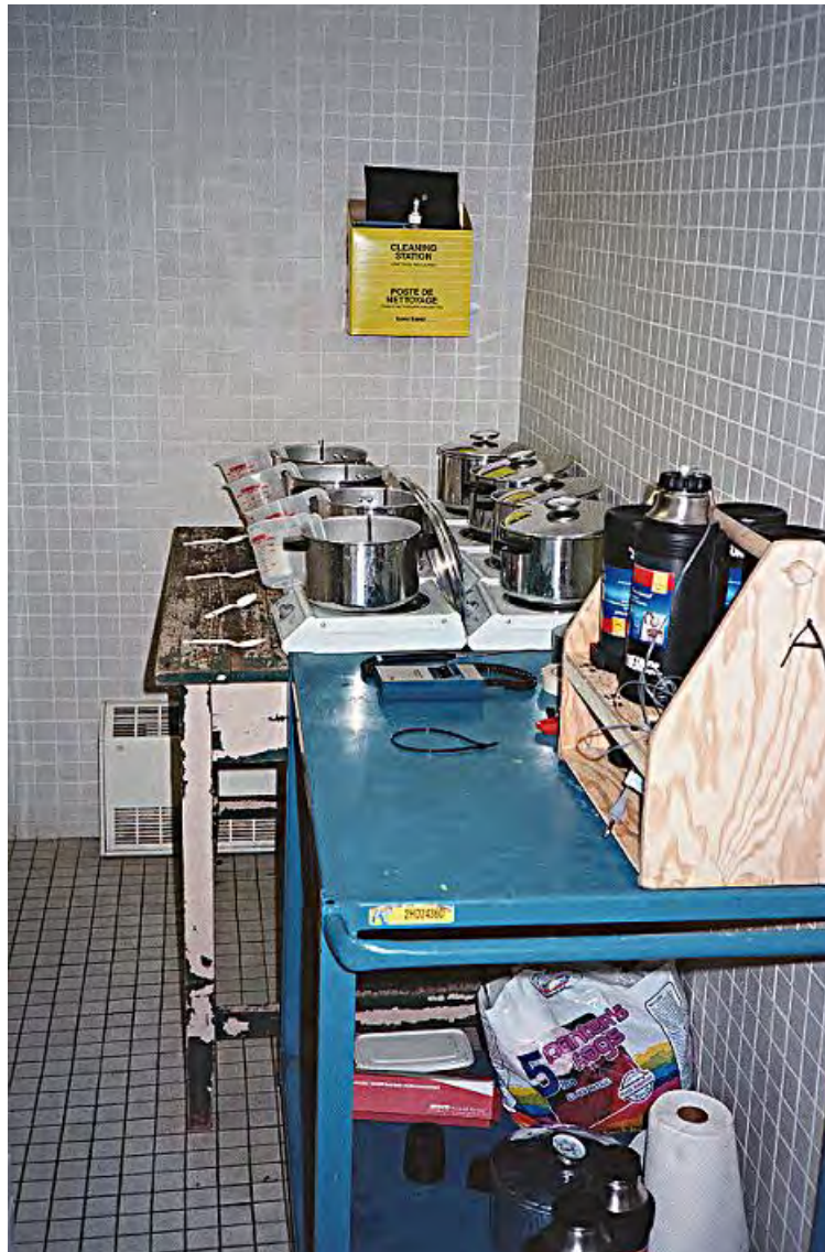
Photo 2.6 Apparatus for Heating Fluids and Transporting Fluids to Test Stand
