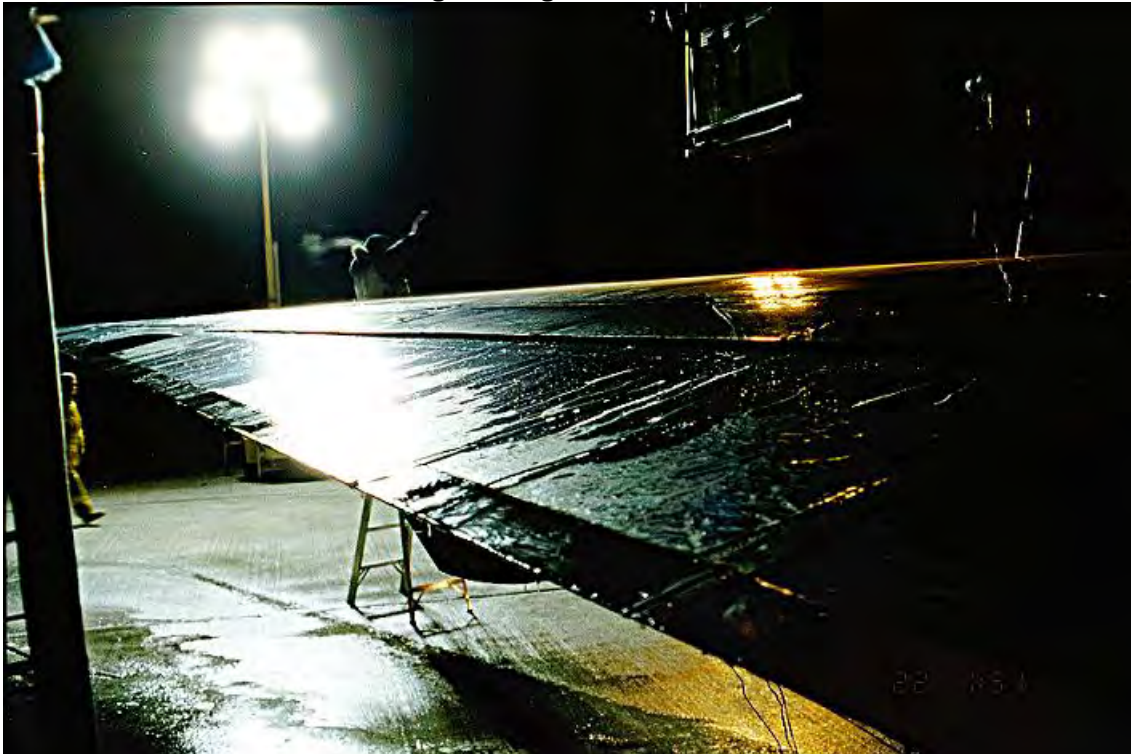
Photo 4.1 Freezing on Flight Control Panels
