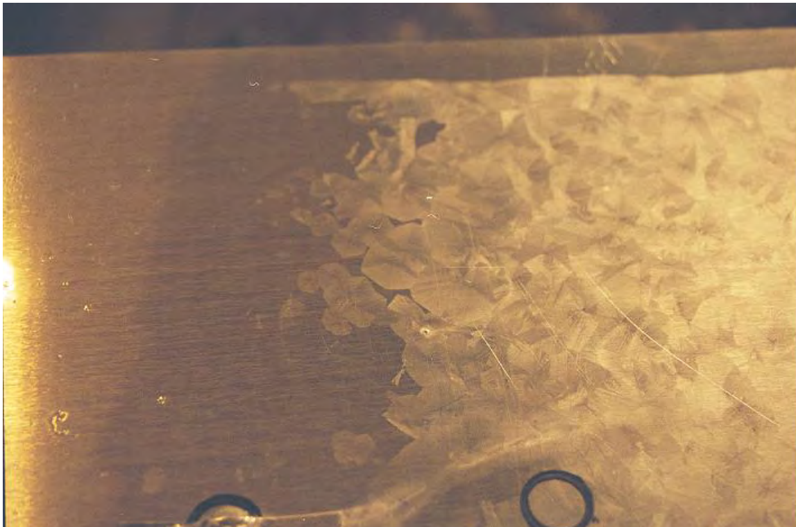
Photo 4.5 Second View of Flash Freezing (Type I)
