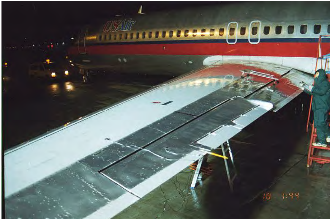
Photo 2.4 Typical Installation of Thermistor Probes on Cold-Soaked Boxes
