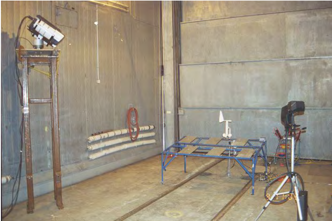
Photo 2.10 Fans Used to Generate Winds
