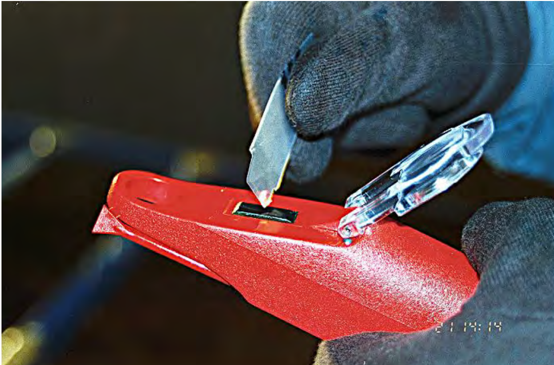
Photo 2.14 Fluid Sample Being Placed on Brixometer
