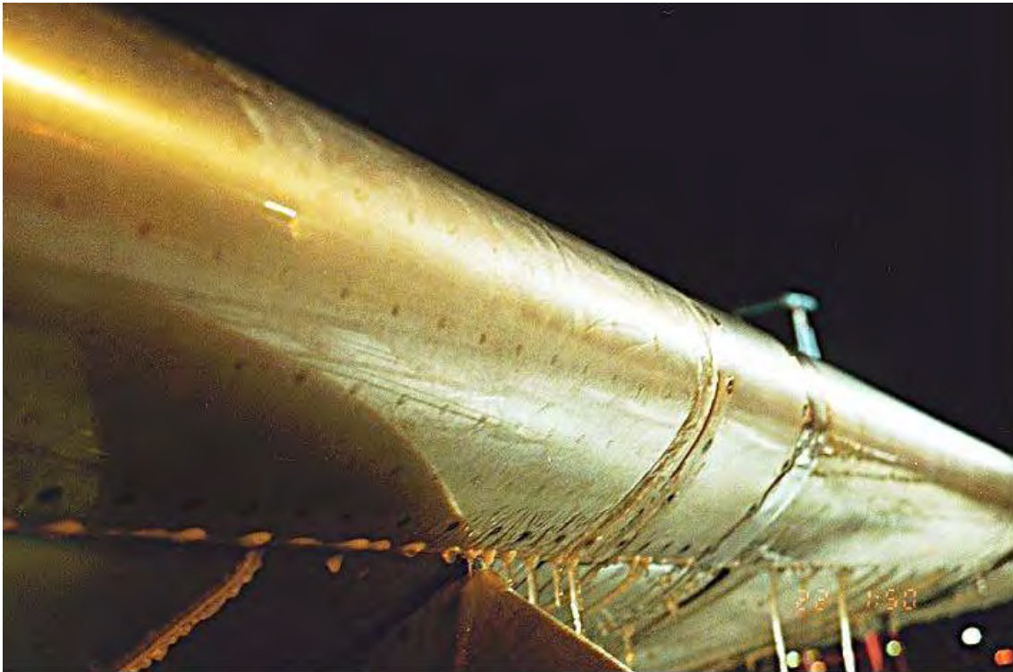
Photo 4.2 Drip Ice at Rear of Leading Edge Slat
