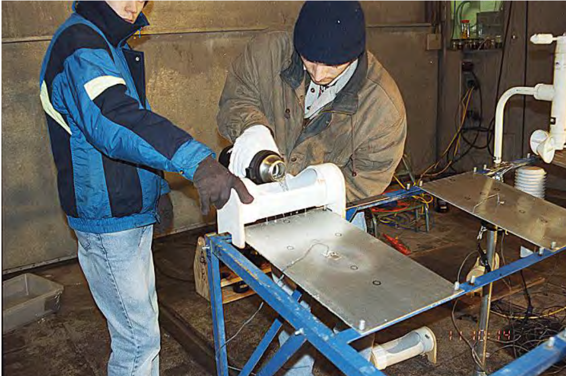
Photo 2.7 Applying Fluid to Test Plate
