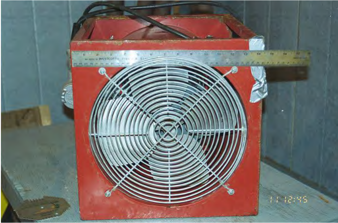
Photo 2.18 Smaller Fan Used for Wind - Initial Evaluation of Wind Effect
