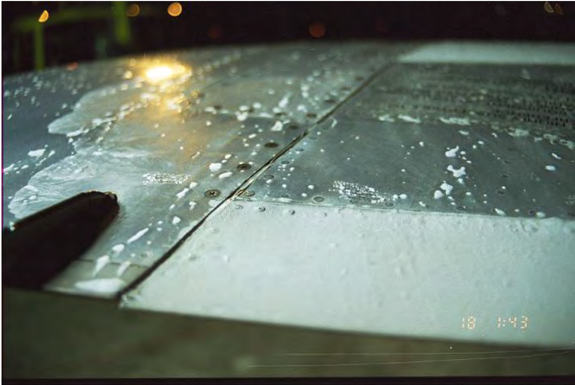
Photo 4.3 Freezing of Thin Film Outboard of Aileron
