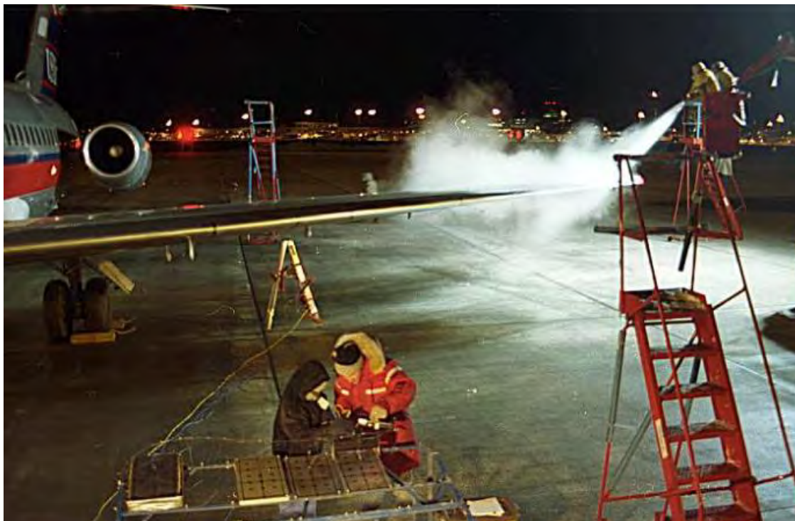
Photo 2.2 Spray Application from Deicing Vehicle and Position of Flat Plate Test Stand
