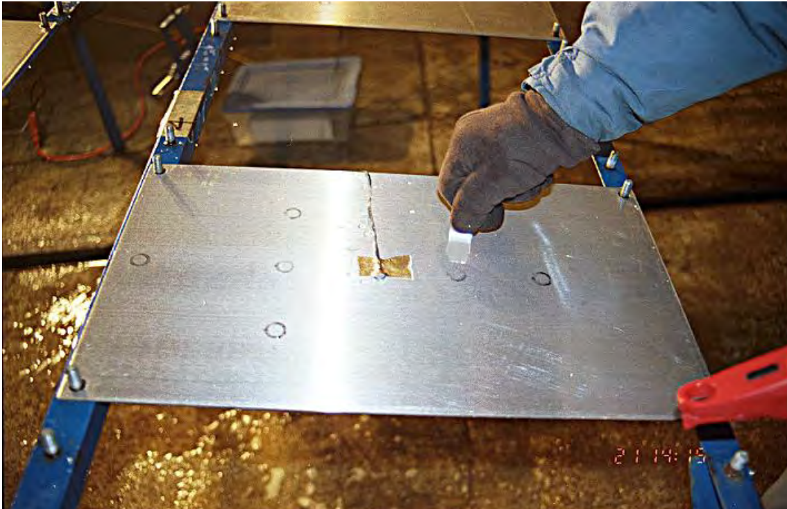
Photo 2.12 Collecting Fluid Sample for Testing Concentration
