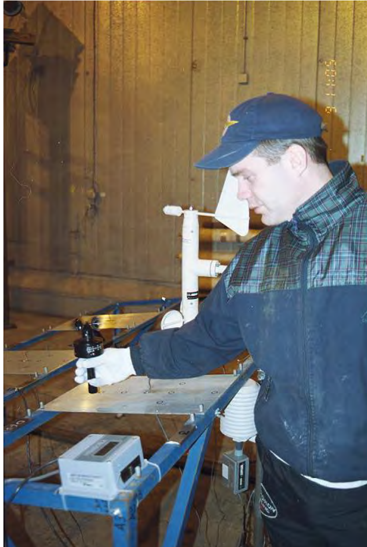
Photo 2.11 Measuring Wind Speed with Hand-held Anemometer and Vaisala RH Meter
