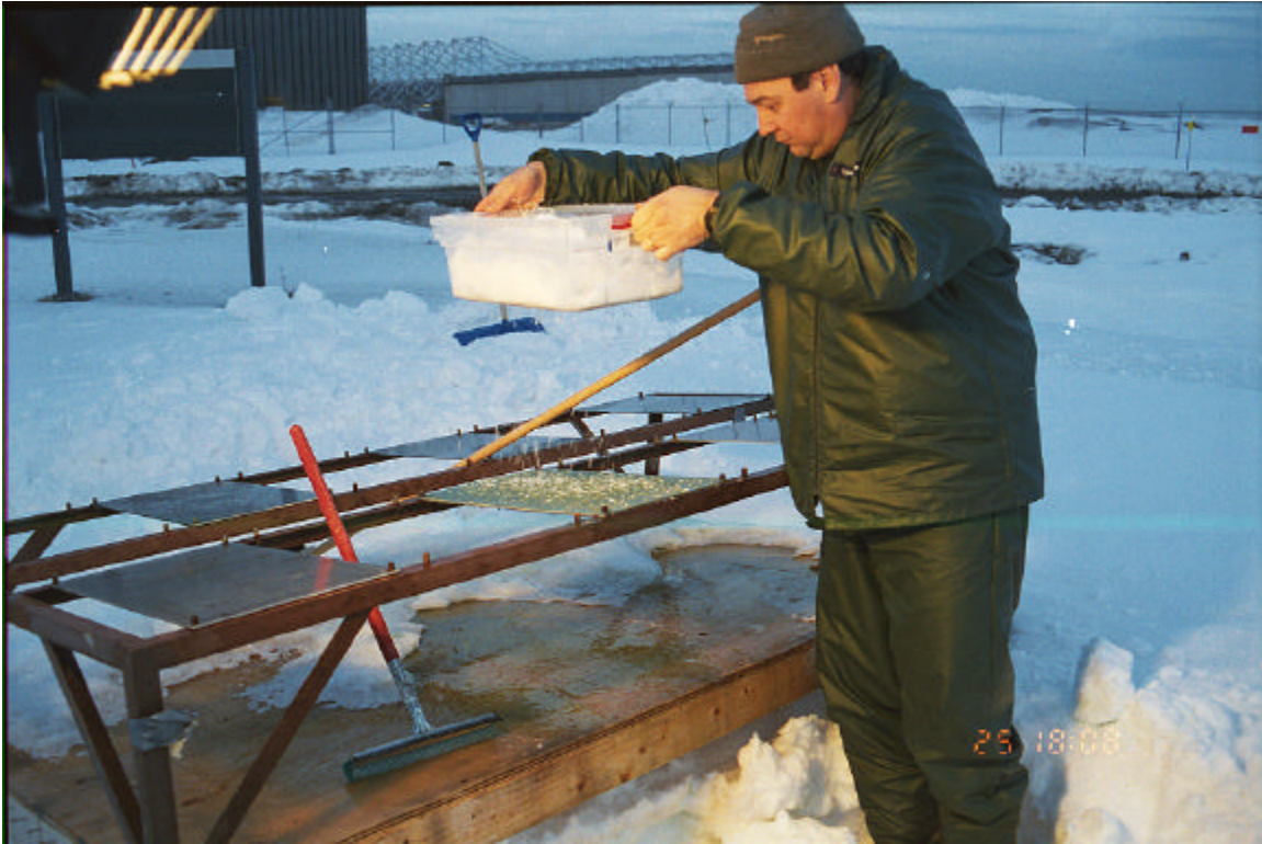
Photo 4.1 Sieve Used to Contaminate Plates
