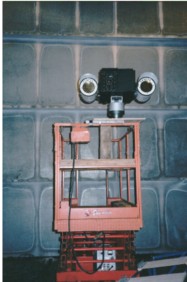
Photo 2.14 Sensor Installation on Scissor Lift
