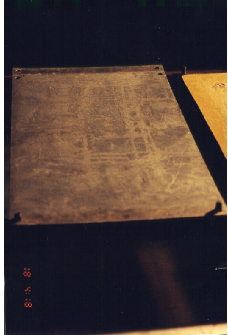
1.6 mm (1/16") Aluminium Plate Following Frost Deposition Test
