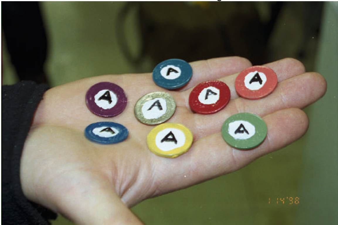
Photo 2.8 Painted Coins Used in Documentation of Roughness of a Failed Fluid
