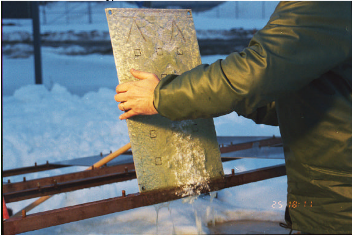
Type IV Failure (at Plate Rotation)
