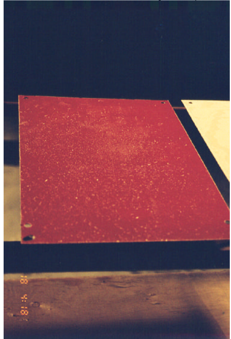
Red 1.6 mm (1/16") Aluminium Plate Following Frost Deposition Test
