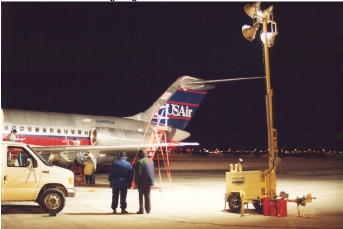
Photo 2.4 Mast Lighting Used for Aircraft Illumination
