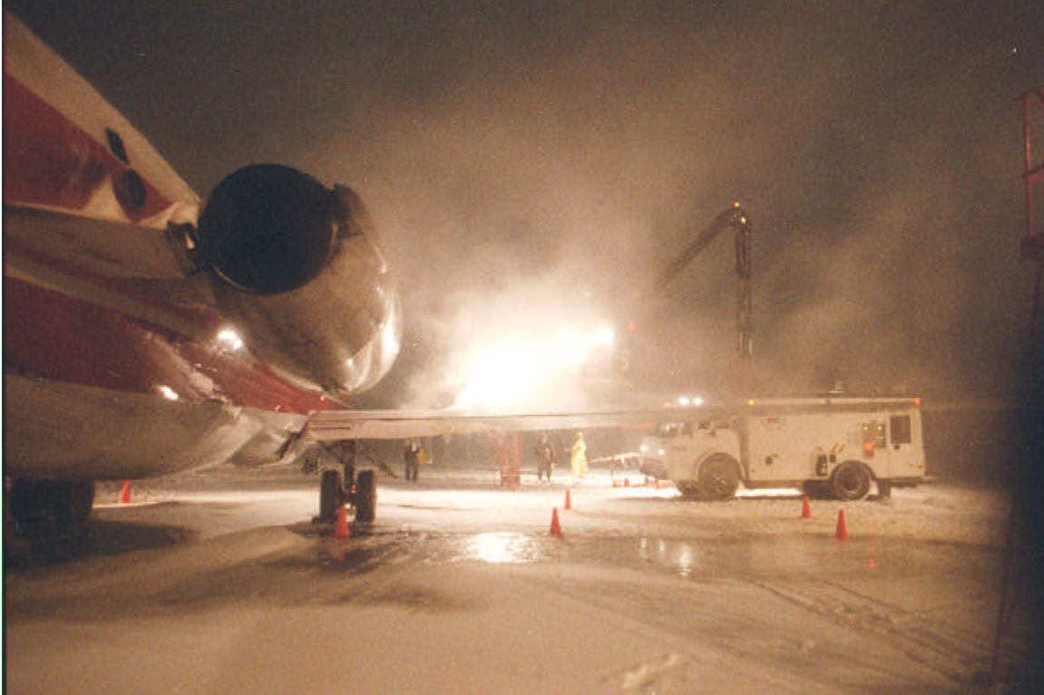
Photo 4.22 Hot Water Deicing
