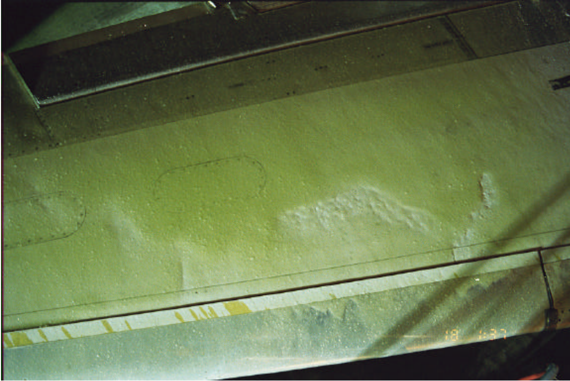
Photo 4.20 Type IV Ultra+ Applied Improperly with Mobile Sprayer
