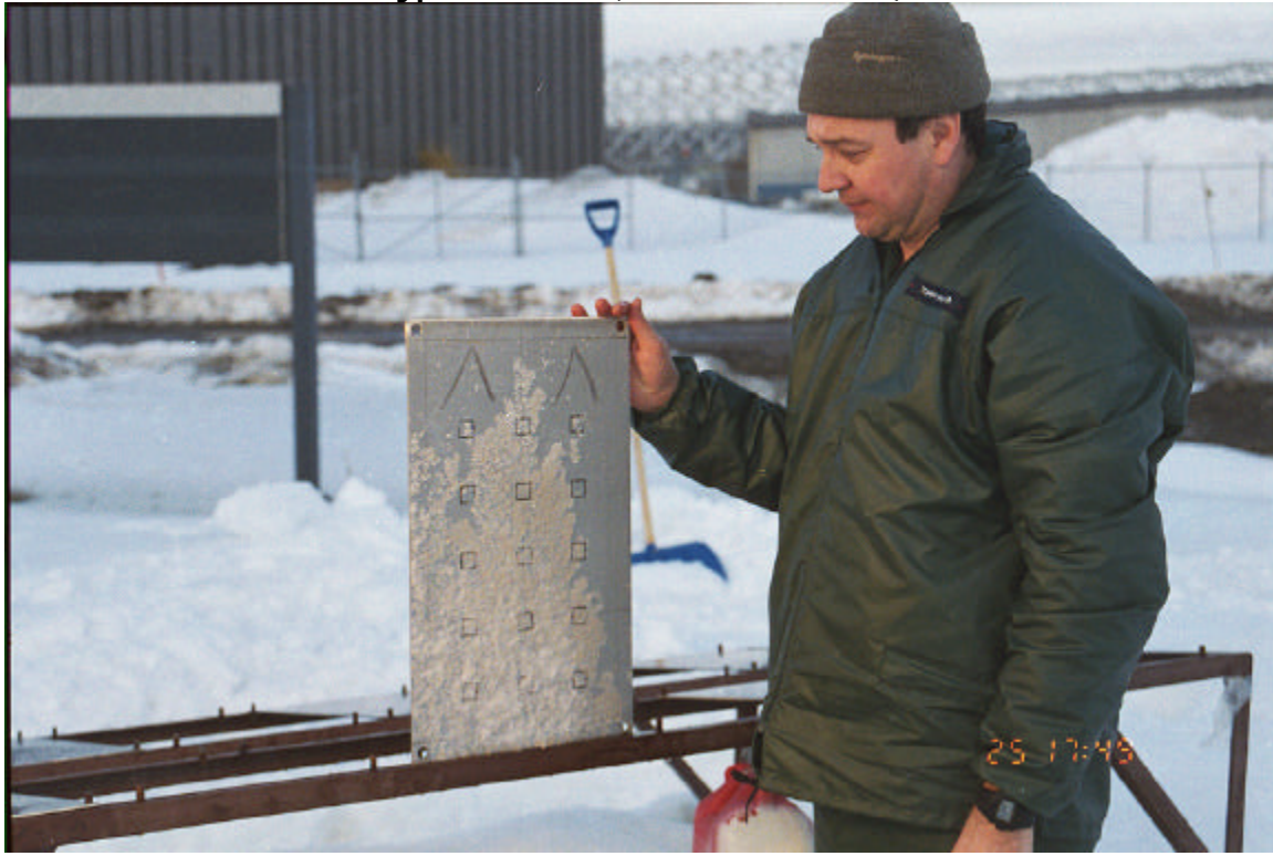
Type I Failure (7 minutes after Plate Rotation)
