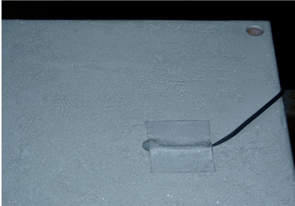
Photo 2.7: Thermistor on Frosted Surface at 15 cm Line
