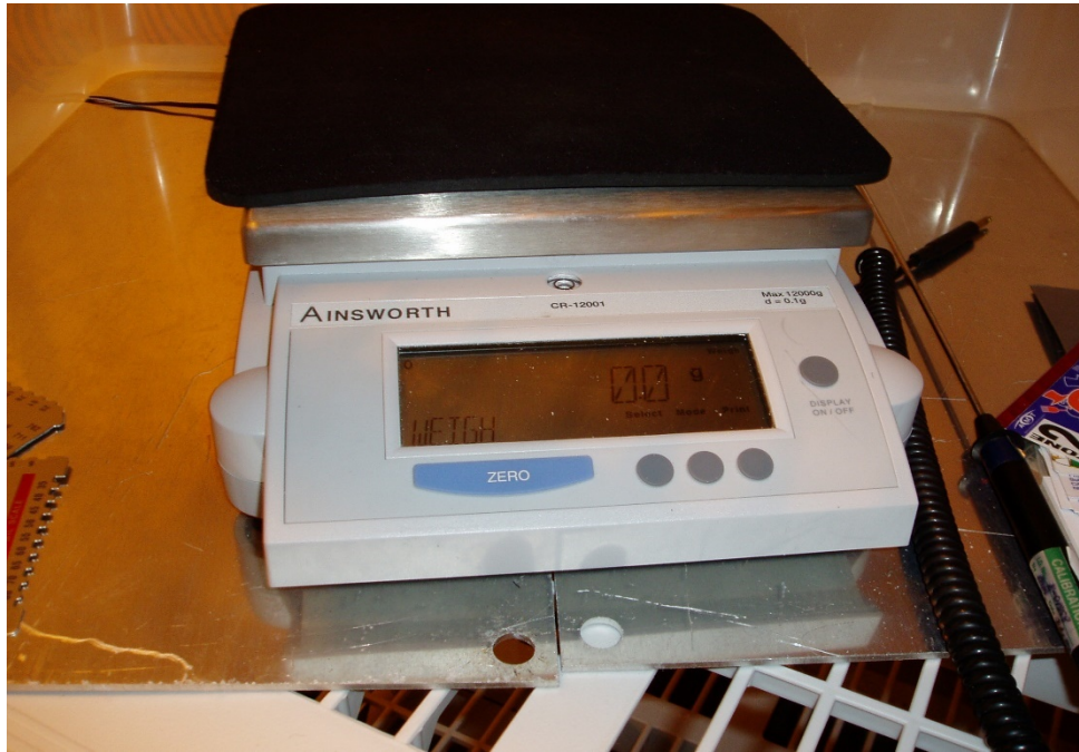
Photo 2.5: Weigh Scale Used to Measure Icing Intensity
