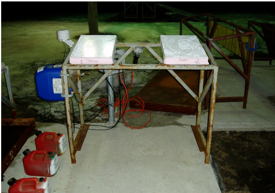
Photo 2.4: Test Stand with Icing Intensity Frosticator Plates
