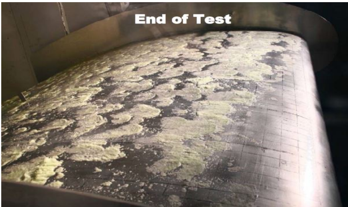
Photo 6.8: Crystalline Formation in Fluid at the End of Test
