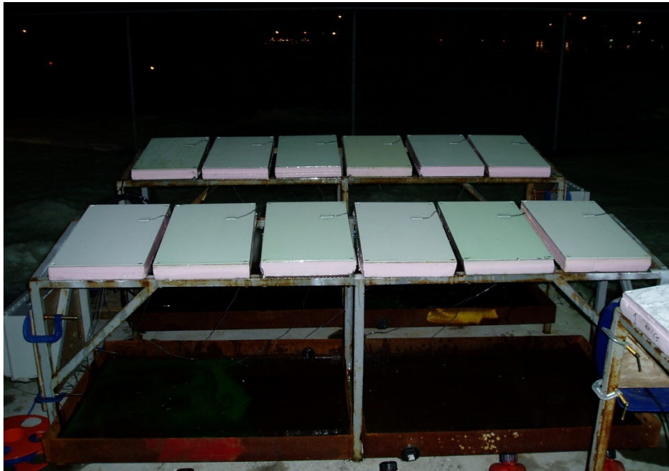
Photo 2.3: Test Stand with Insulated Frosticator Plates
