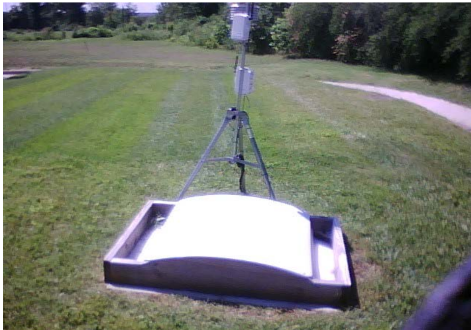
Photo 3.2: UPS Representative Aircraft Wing Surface
