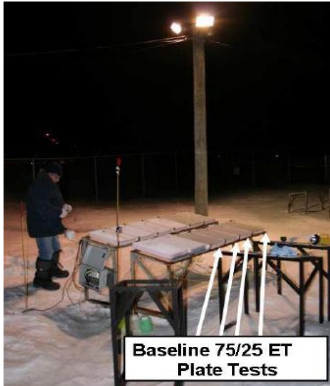
Photo 6.3: White Painted Insulated Flat Plate Setup at APS Test Facility
