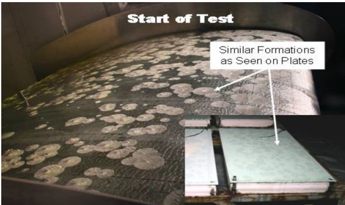
Photo 6.6: Crystalline Formation in Fluid at Start of High Speed Test Run
