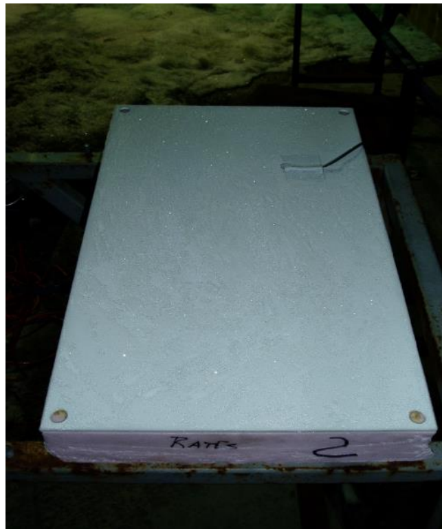
Photo 2.2: Frost Plate with Insulated Backing
