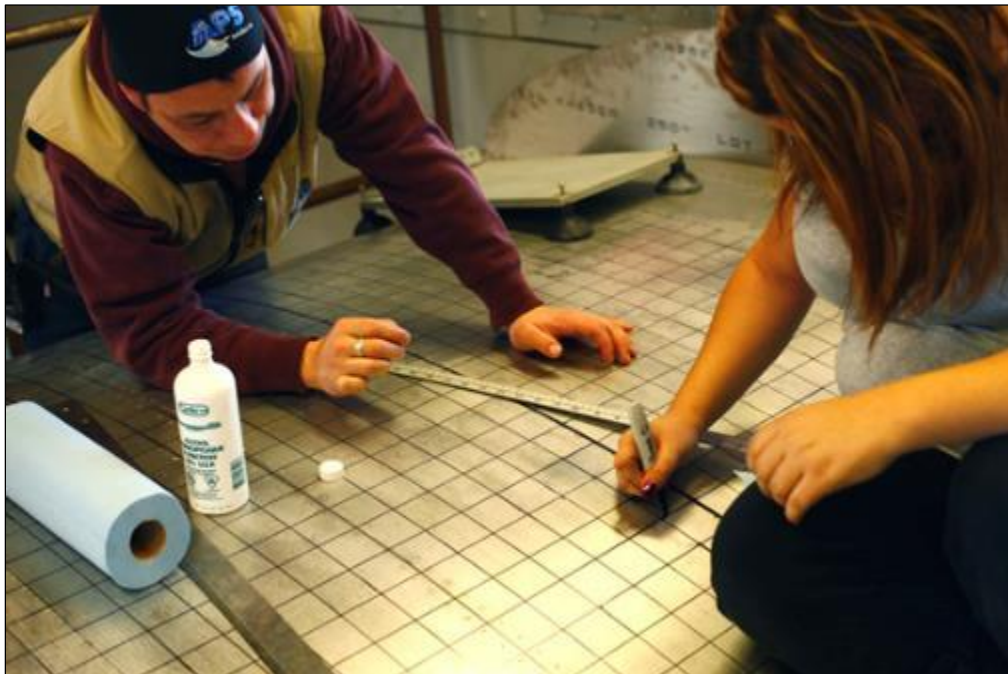
Photo 2.4: Grid Markings on NASA LS(1)-0417 Wing Section
