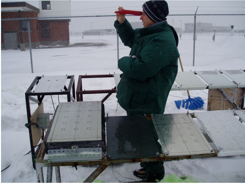
Photo 3.7: Using Brixometer to Measure Fluid Brix
