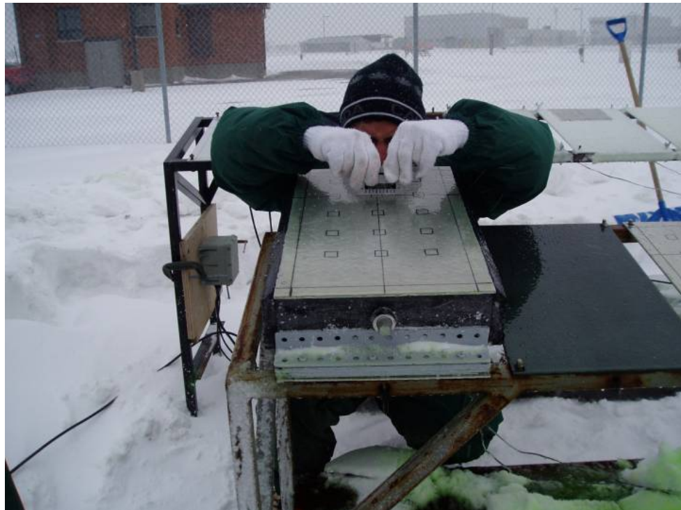
Photo 3.8: Fluid Thickness Measurement Using Wet Film Thickness Gauge
