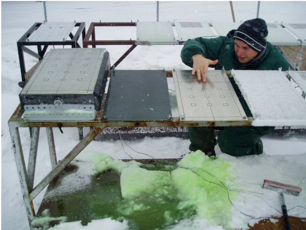
Photo 3.6: Obtaining Fluid Sample for Brix Measurement
