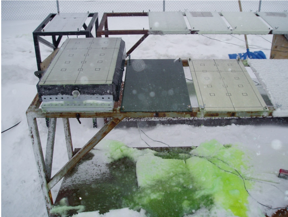
Photo 3.3: Comparative Endurance Time Testing Setup - Outdoors
