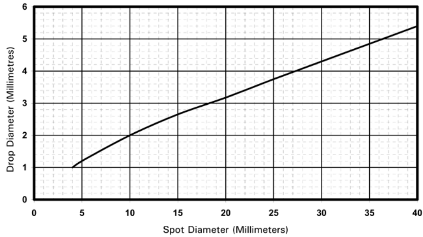
CONVERSION OF SPOT DIAMETER TO DROP DIAMETER WHATMAN # 1 FILTER PAPER
