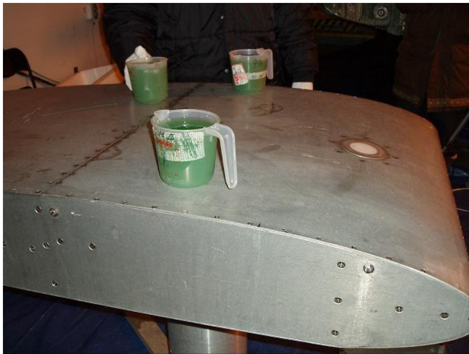
Photo 2.8: Fluid Application to Airfoil
