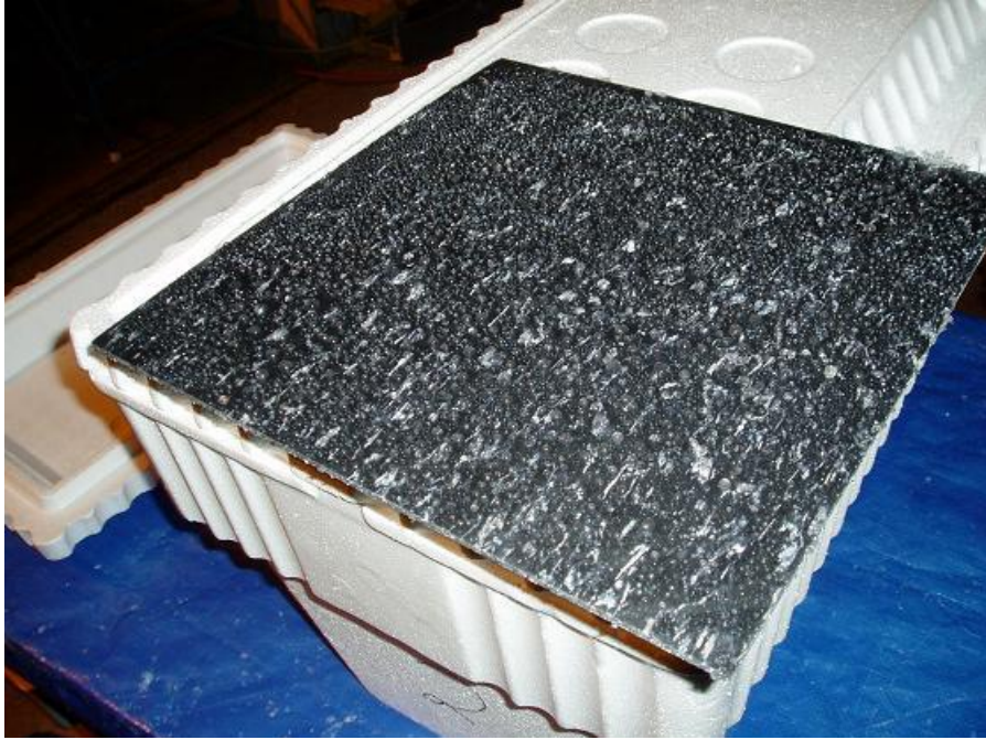
Photo 2.9: Composite Tile Surface Used to Produce Ice Pellets
