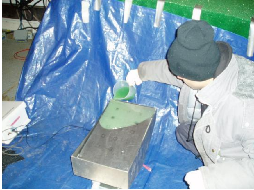
Photo 2.3: Fluid Application to Standard Aluminum Test Plate in NCAR Bucket
