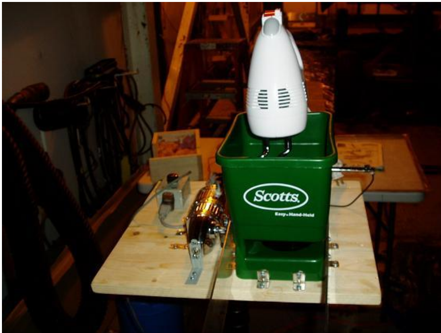
Photo 2.4: Ice Pellet Pitcher Used to Simulate Ice Pellet Precipitation Conditions
