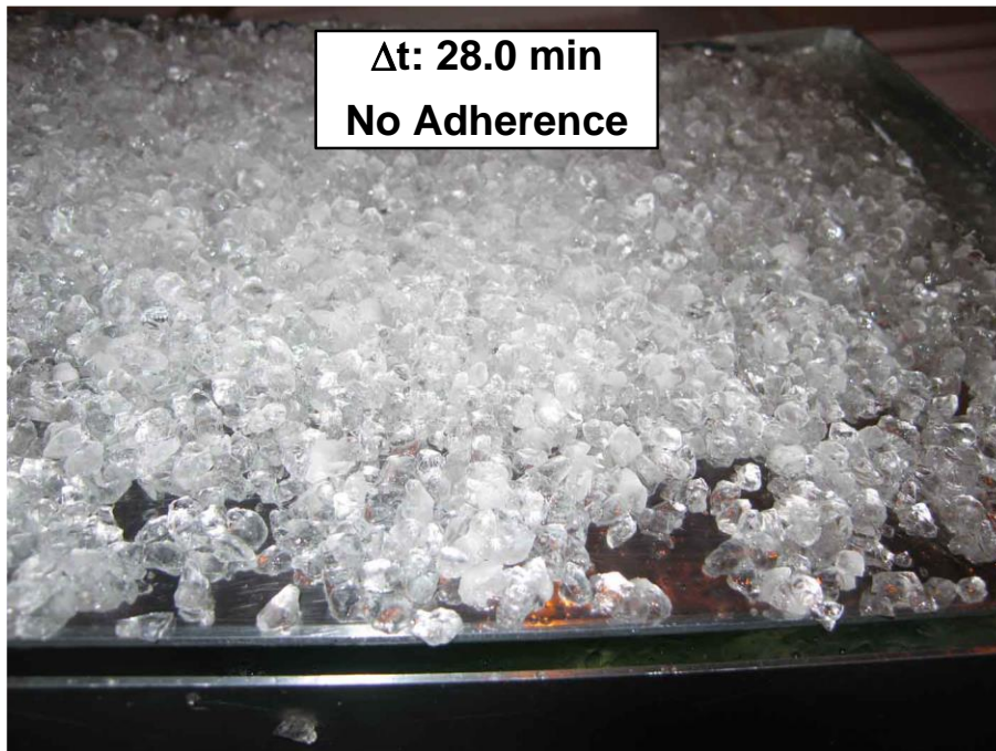
Photo 9.14: Adherence Test #10 – Photo 8 Type IV PG 50/50 Applied at 60°C, IP (4-5.8 mm, \approx 25 \text{ g/dm}^2/\text{h} ), -3°C
