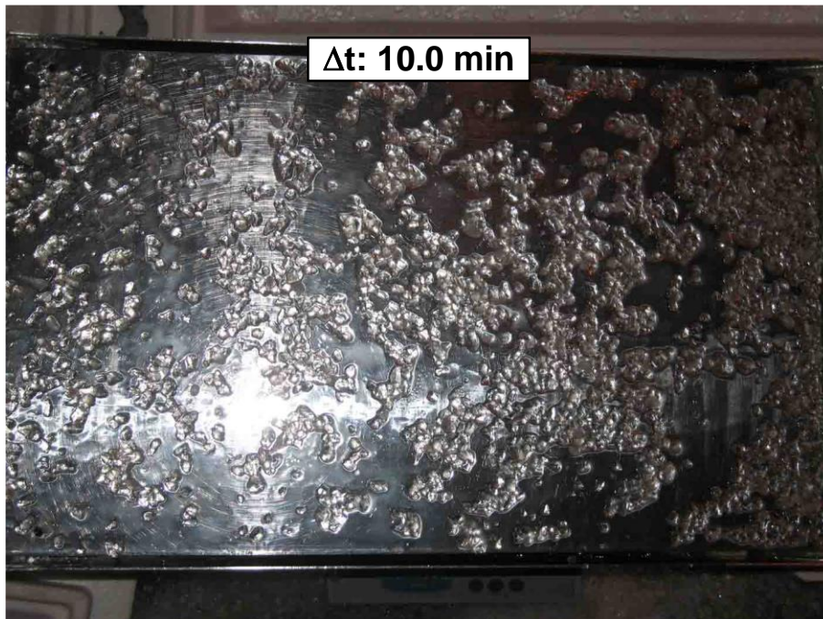
Photo 9.10: Adherence Test #10 – Photo 4 Type IV PG 50/50 Applied at 60°C, IP (4-5.8 mm, \approx 25 \text{ g/dm}^2/\text{h} ), -3°C
