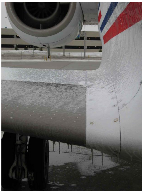
Photo 7.2: View of Falcon 20 Wing Section with Adhered Ice Pellets and Freezing Rain – Photo 2
