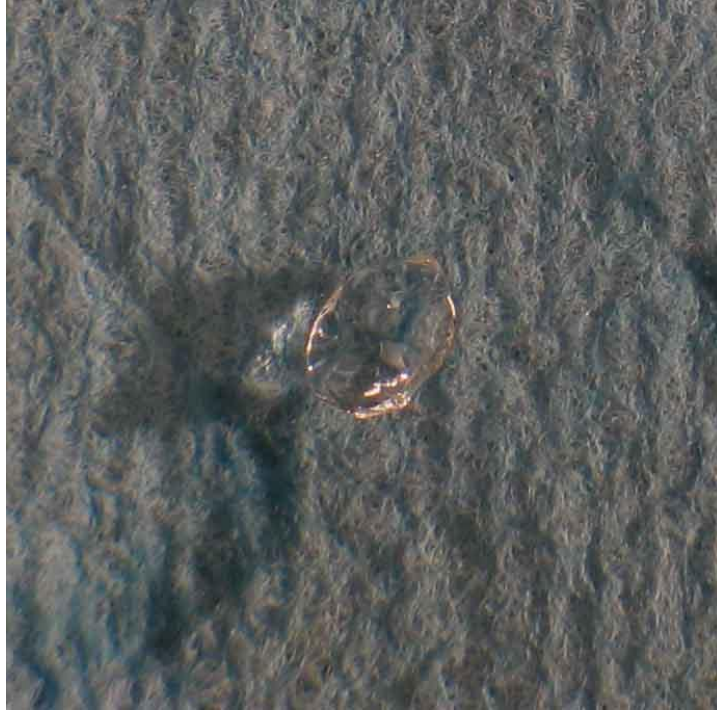
Photo 4.5: Crushed Ice Pellet after Being Submerged for 16 Minutes in Aircraft Deicing Fluid
