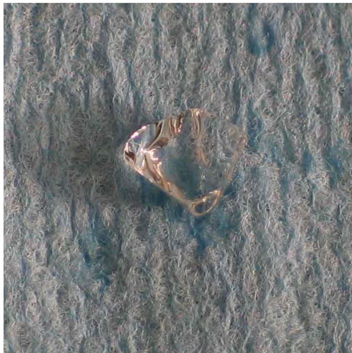
Photo 4.4: Crushed Ice Pellet After being Submerged for 8 Minutes in Aircraft Deicing Fluid
