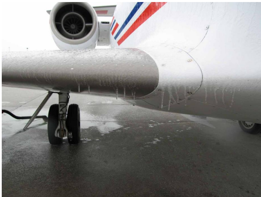
Photo 7.1: View of Falcon 20 Wing Section with Adhered Ice Pellets and Freezing Rain – Photo 1
