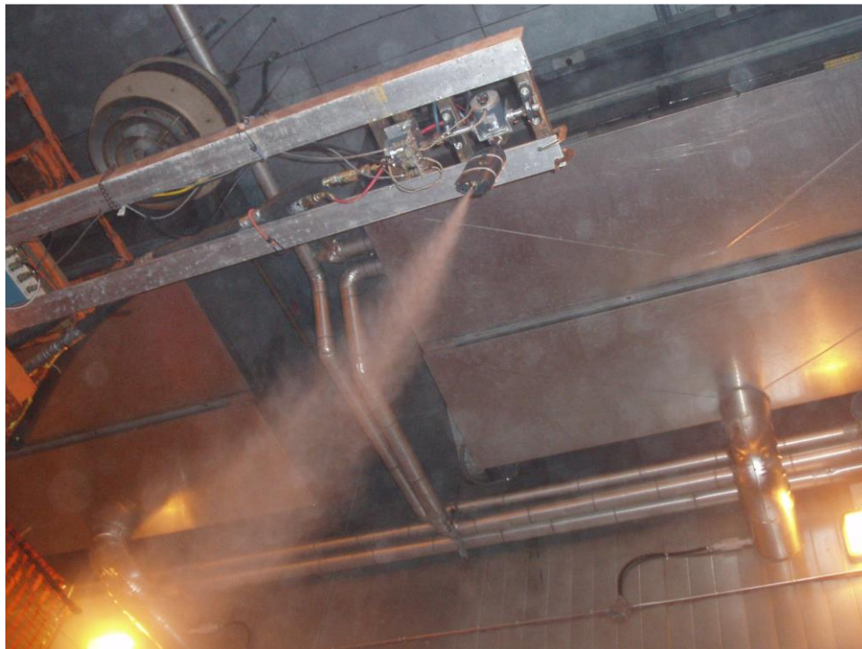
Photo 2.2: Sprayer Assembly Used to Produce Fine Droplets
