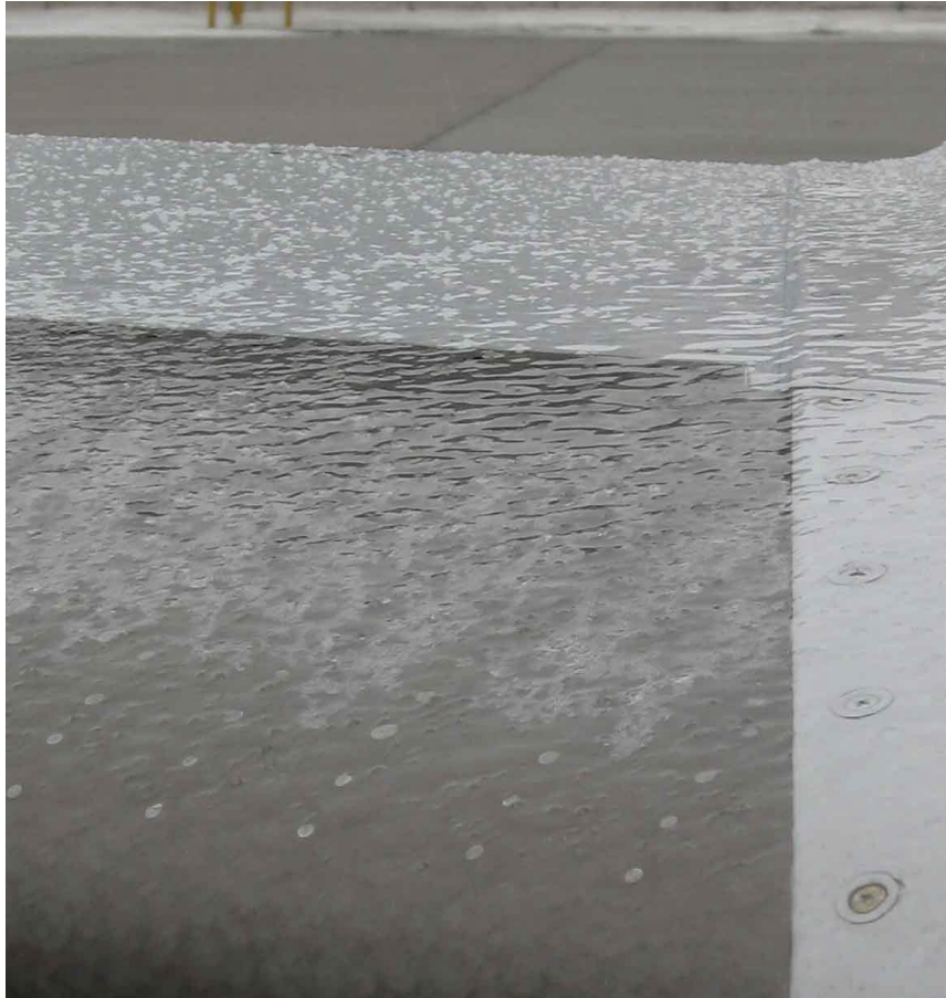
Photo 7.3: Close-up View of Rough Surface Caused by Adhered Ice Pellets and Freezing Rain on Falcon 20 Wing Section – Photo 2
