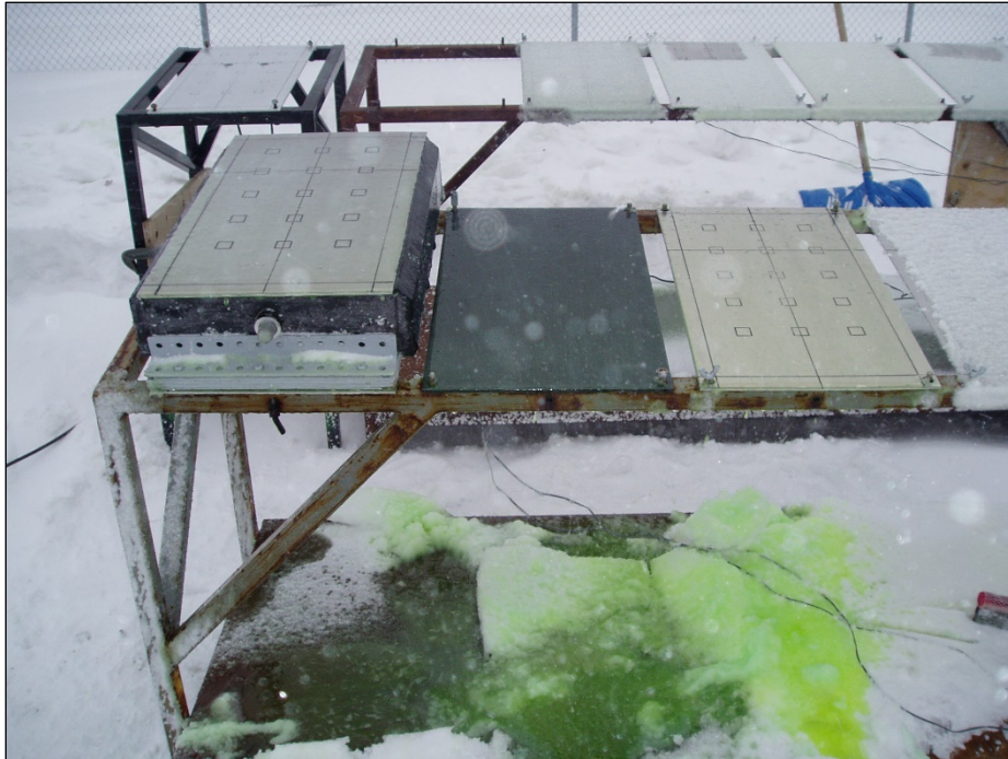
Photo 2.3: Comparative Endurance Time Testing Setup – Outdoors
