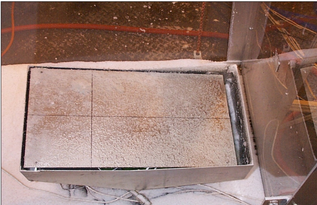
Photo 4.2: Artificial Snow Testing – Adhesion Failure
