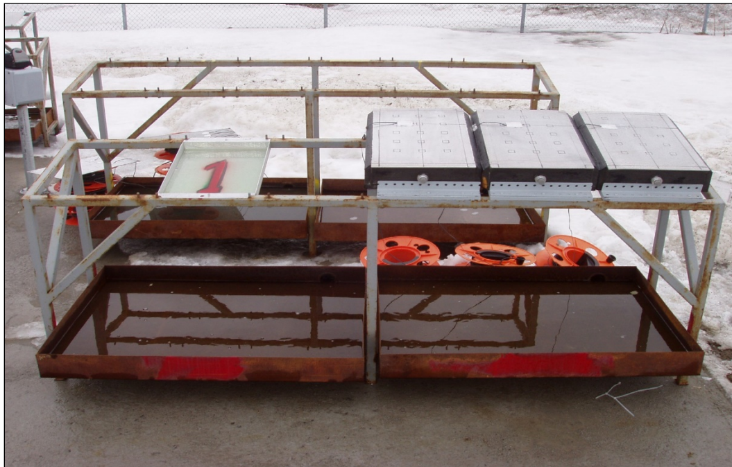
Photo 2.2: APS Test Site – Test Stand Used for Natural Snow Adhesion Tests
