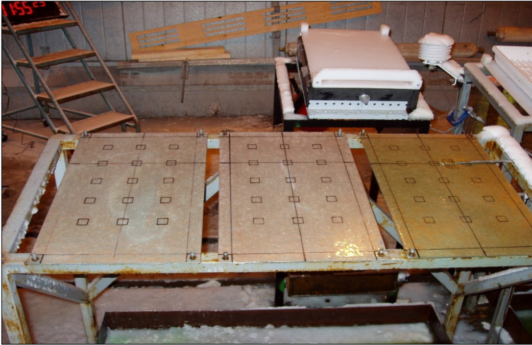
Photo 3.1: Test Stands Used for Freezing Precipitation Adhesion Tests
