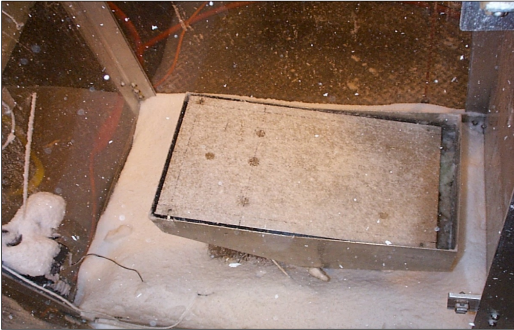
Photo 4.3: Artificial Snow Testing – Snow Build-Up on the Surface of the Plate
