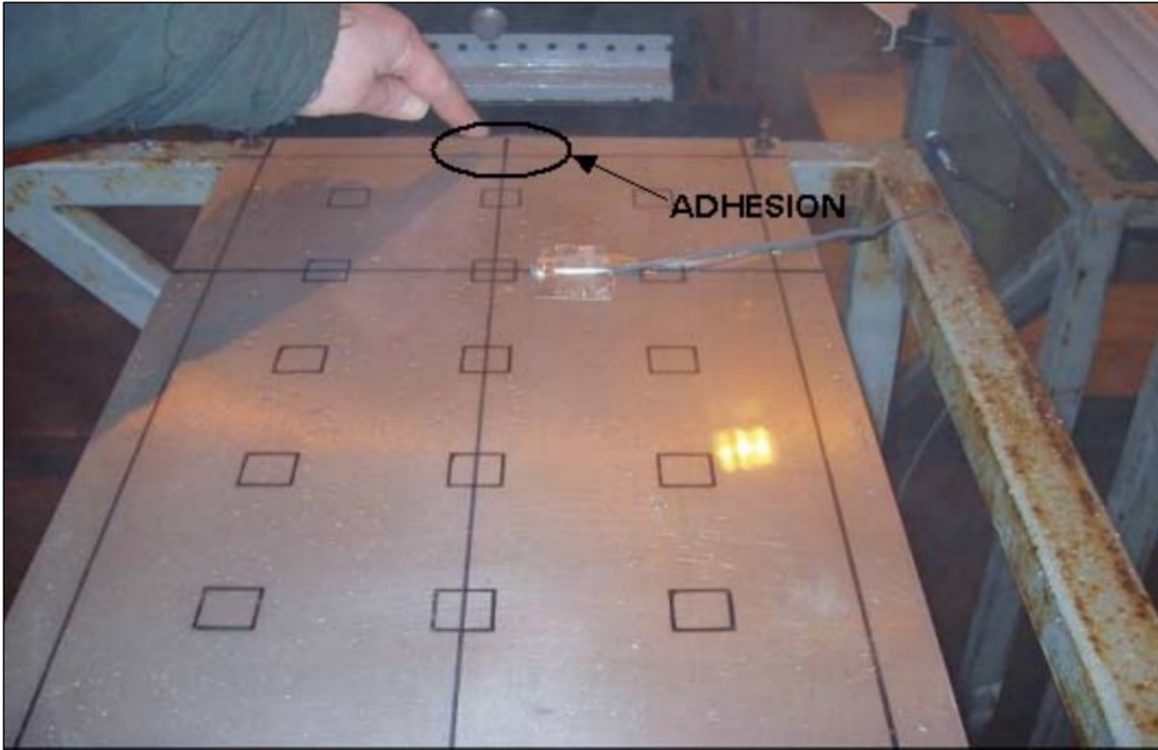
Photo 3.3: Onset of Adhesion Under Freezing Precipitation at NRC
