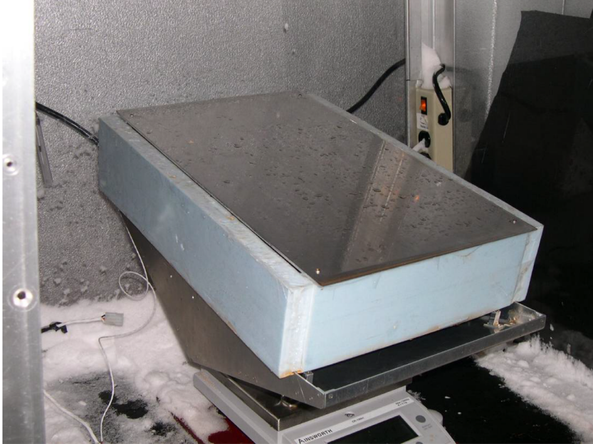
Photo 2.13: Standard Plate Setup for Type I Testing with Artificial Snowmaker
