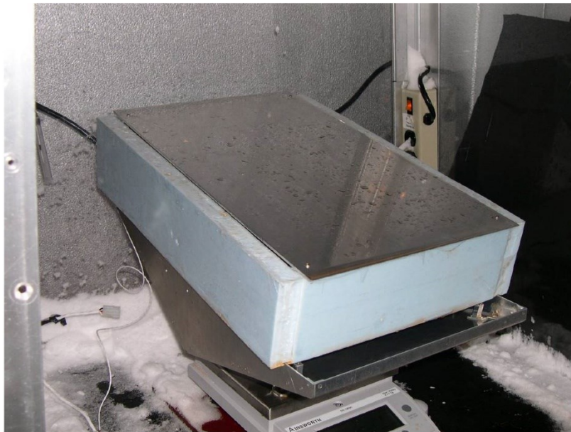
Photo 2.14: Standard Plate Setup for Type I Testing with Artificial Snowmaker
