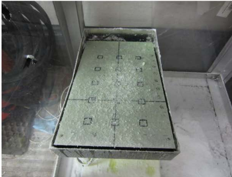
Photo 3.4: Standard Plate Setup for Testing with Artificial Snowmaker
