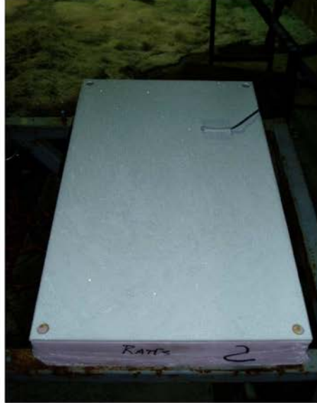
Photo 3.3: Frost Plate with Insulated Backing
