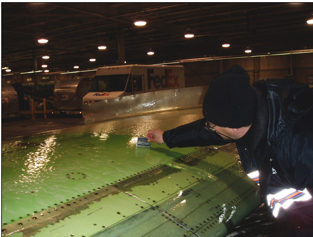
Photo 3.2: Measuring Fluid Thickness
