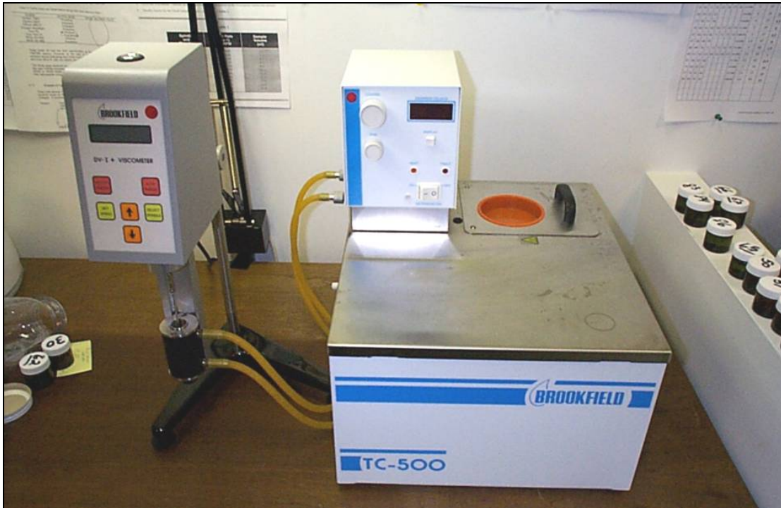
Photo 2.9: Brookfield LV DV-I+ Digital Viscometer
