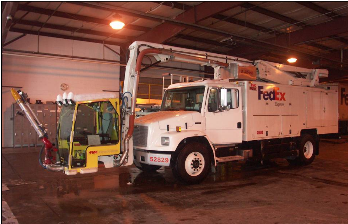
Photo 2.6: FMC LMD 2000 Deicing Truck
