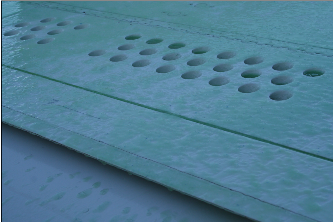
Photo 4.11: Residual Fluid on Trailing Edge after Run 8
