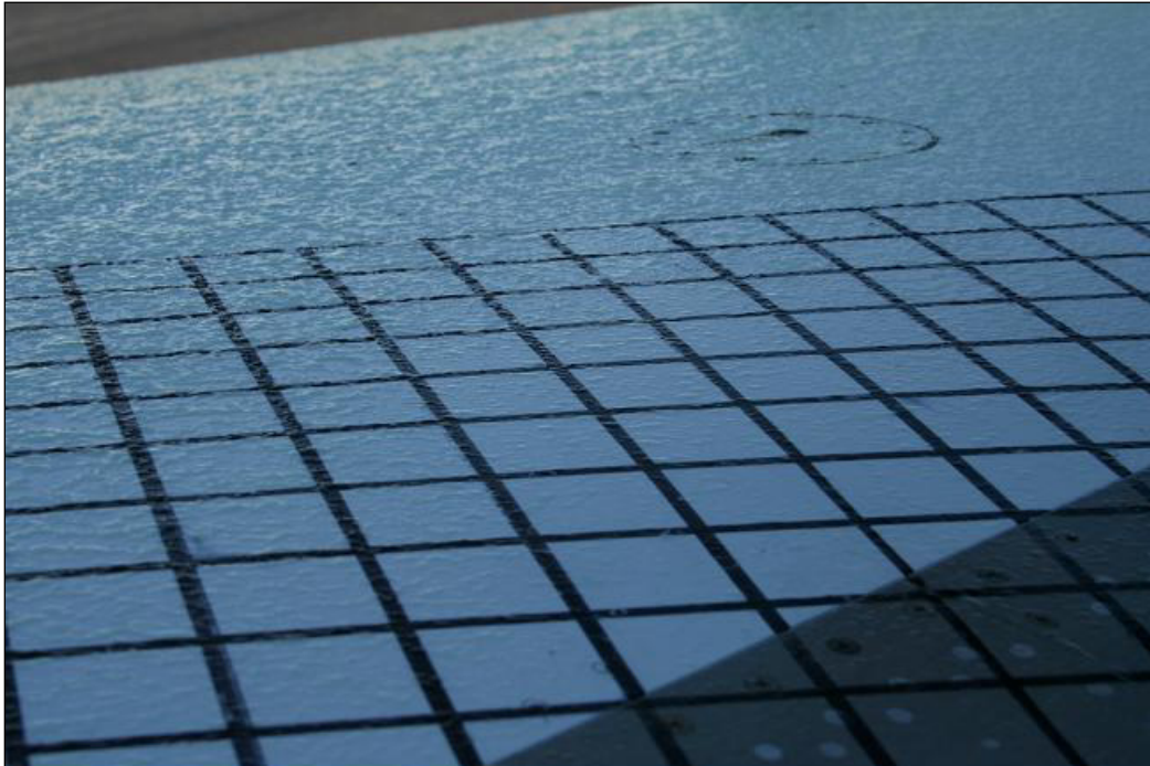
Photo 4.1: Typical Residual Fluid Left After Runs 1 to 7
