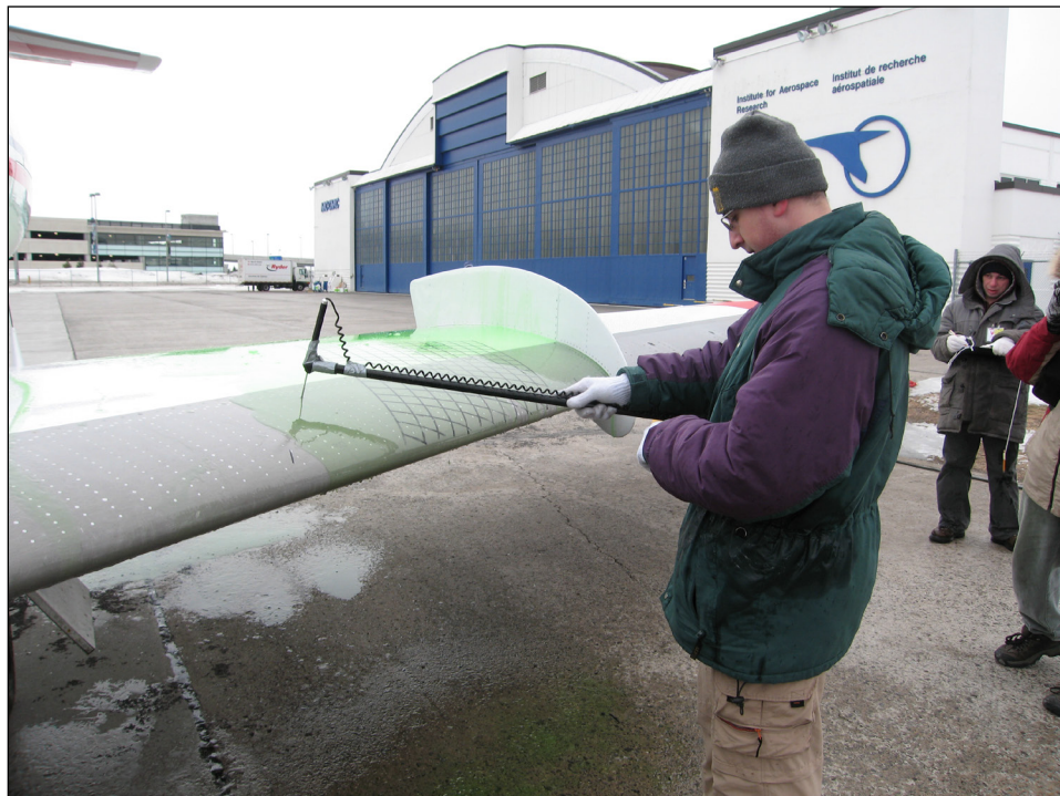
Photo 2.12: Wing Surface Temperature Measurement
