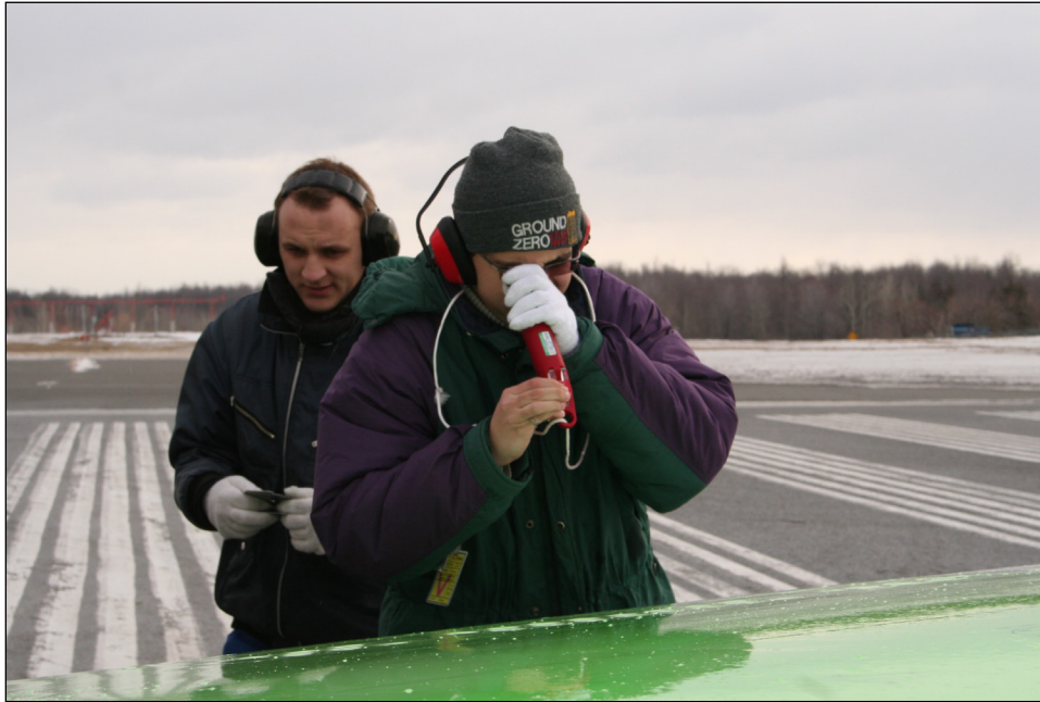
Photo 2.11: Fluid Freezing Point Measurement Using Hand-held Refractometer
