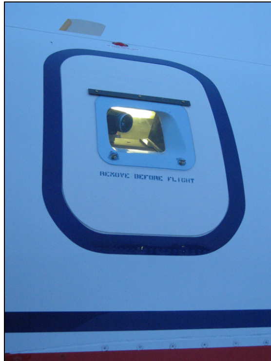
Photo 2.13: Temporary Structure Fitted with Camera-Mounting Capability
