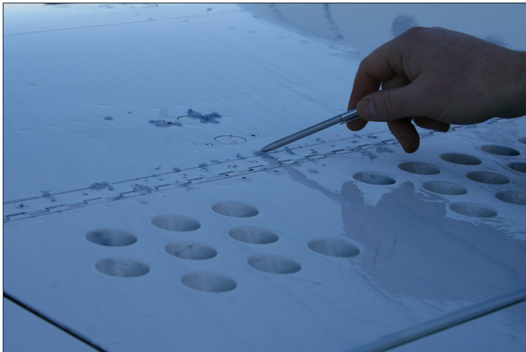
Photo 4.12: Residual Fluid and Ice Pellets Adhering to the Trailing Edge After Run 9
