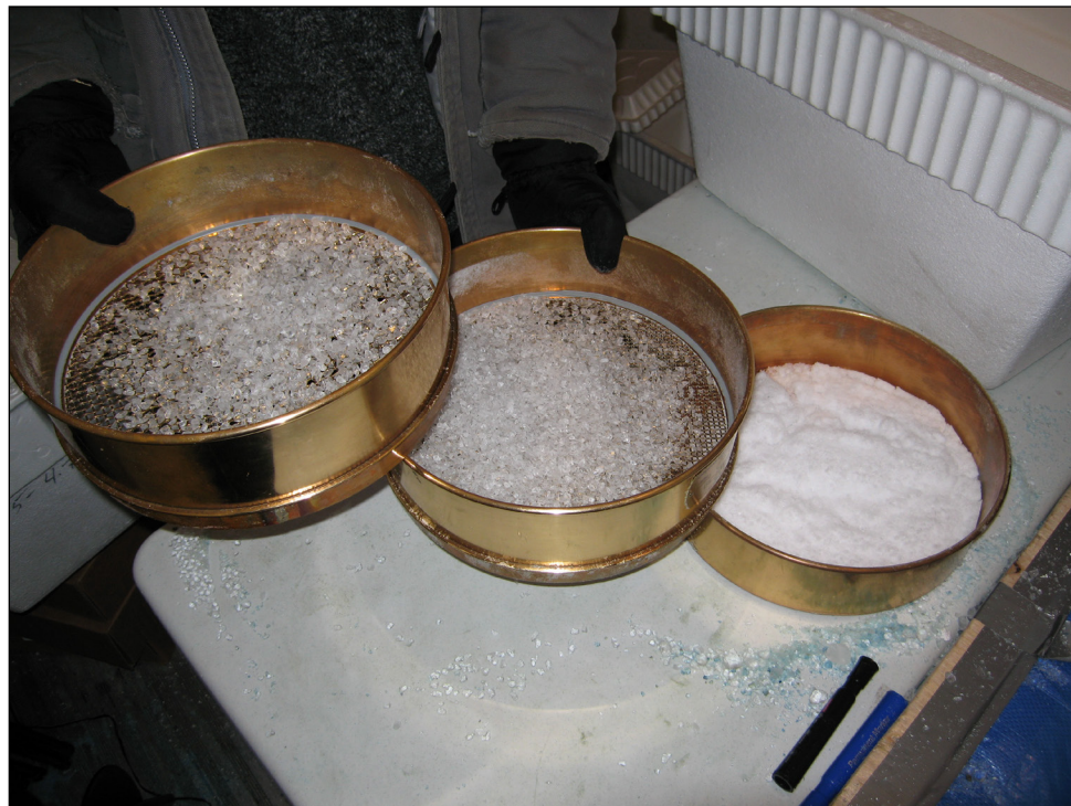
Photo 2.8: Calibrated Sieves Used to Obtain Desired Size Distribution
