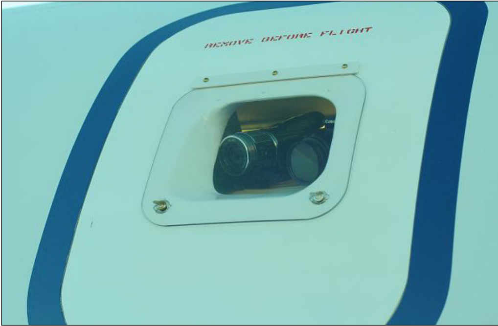
Photo 3.7: Still and Video Camera Overlooking Test Area
