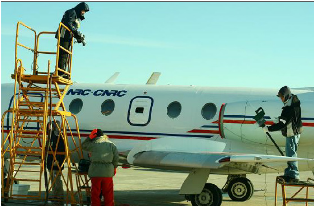
Photo 3.4: Freezing Rain Sprayer Setup
