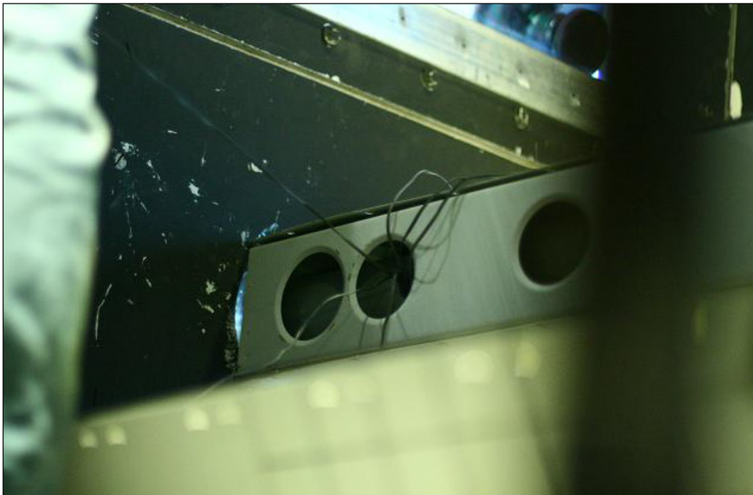
Photo 2.6: Temperature Probes Inside Wing Area
