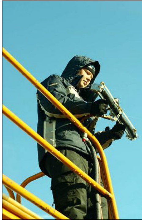
Photo 2.17: Freezing Rain Sprayer Hand-Held Spray Bar
