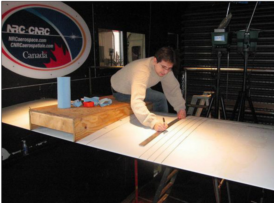
Photo 2.3: NACA 23012 Wing Section Used for Testing
