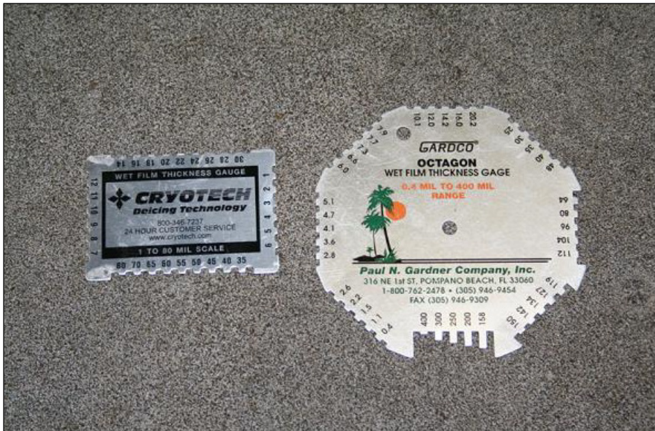
Photo 2.10: Wet Film Thickness Gauges
