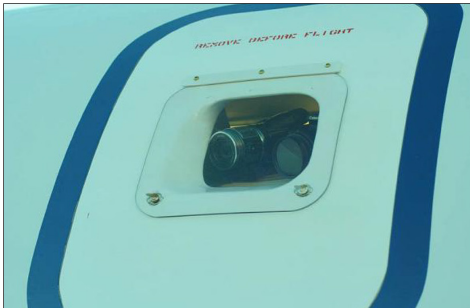
Photo 2.18: Camera Positioning Inside Emergency Exit Windows
