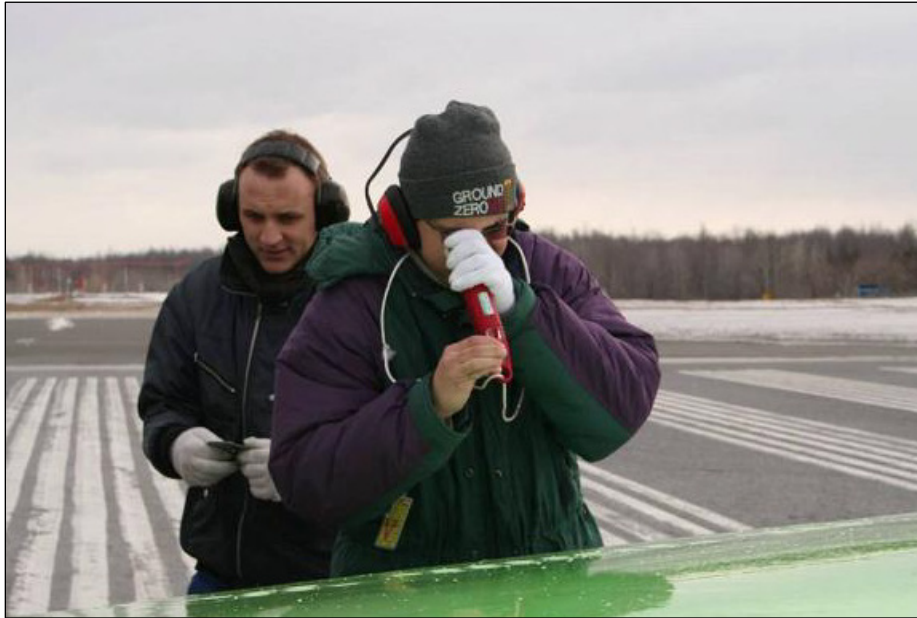
Photo 2.21: Fluid Freezing Point Measurement Using Hand-Held Brixometer
