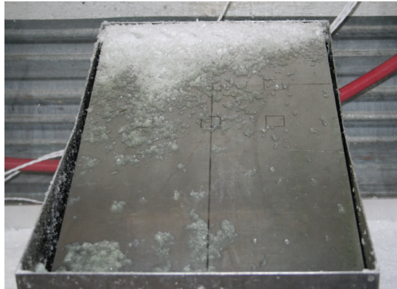
Photo 5.2: Fluid Failure During Mixed IP/SN Conditions – SN as Dominant Condition
