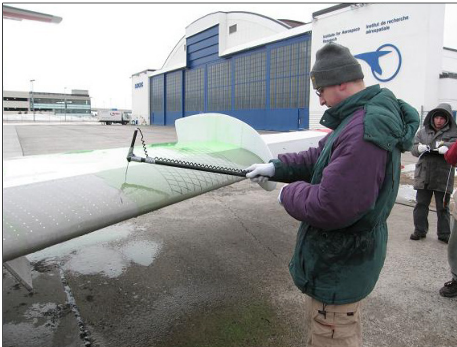
Photo 2.22: Wing Surface Temperature Measurement
