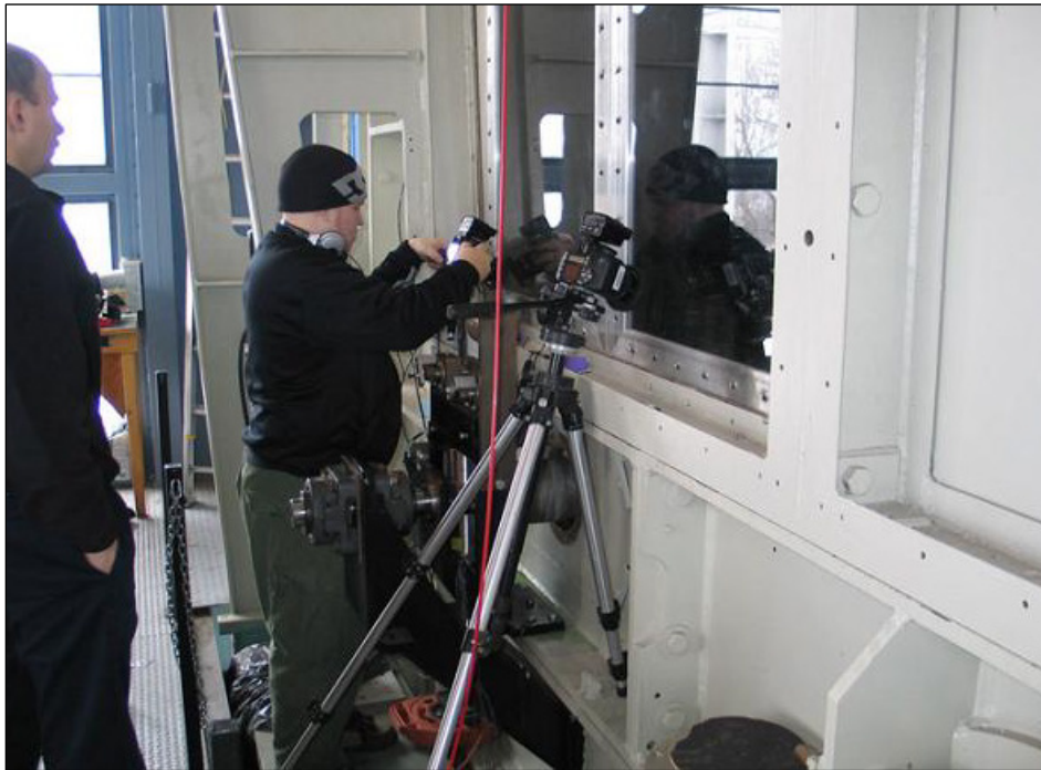
Photo 2.8: Wind Tunnel Setup for Digital Cameras
