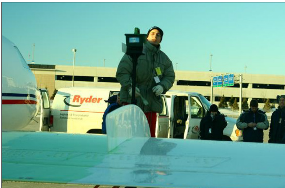
Photo 2.16: Ice Pellet Dispenser Setup for Falcon 20 Tests
