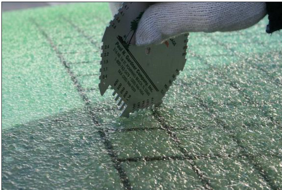
Photo 2.20: Fluid Thickness Measurement Using Wet Film Thickness Gauge
