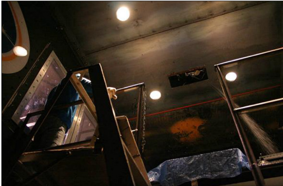
Photo 2.6: Ceiling-Mounted Freezing Rain Sprayer
