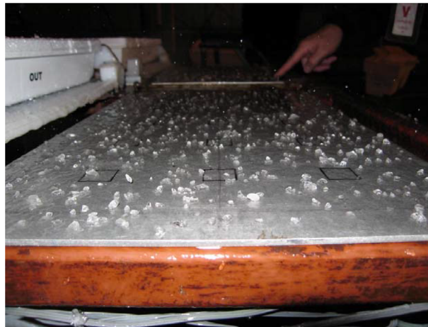
Photo 5.2: Adherence to 15 cm Line Caused by Light Mixed Icing (ZR / IP)
