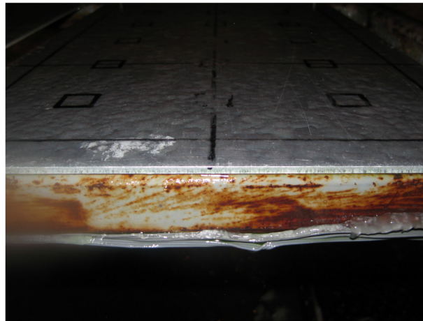
Photo 5.1: First Adherence Caused by Light Freezing Rain Alone
