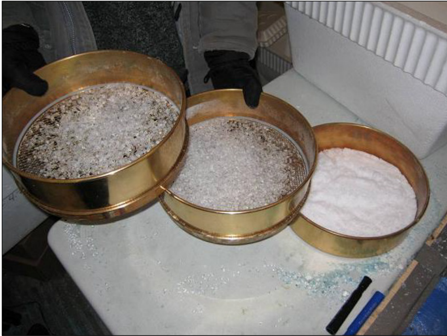
Photo 2.25: Calibrated Sieves Used to Obtain Desired Size Distribution
