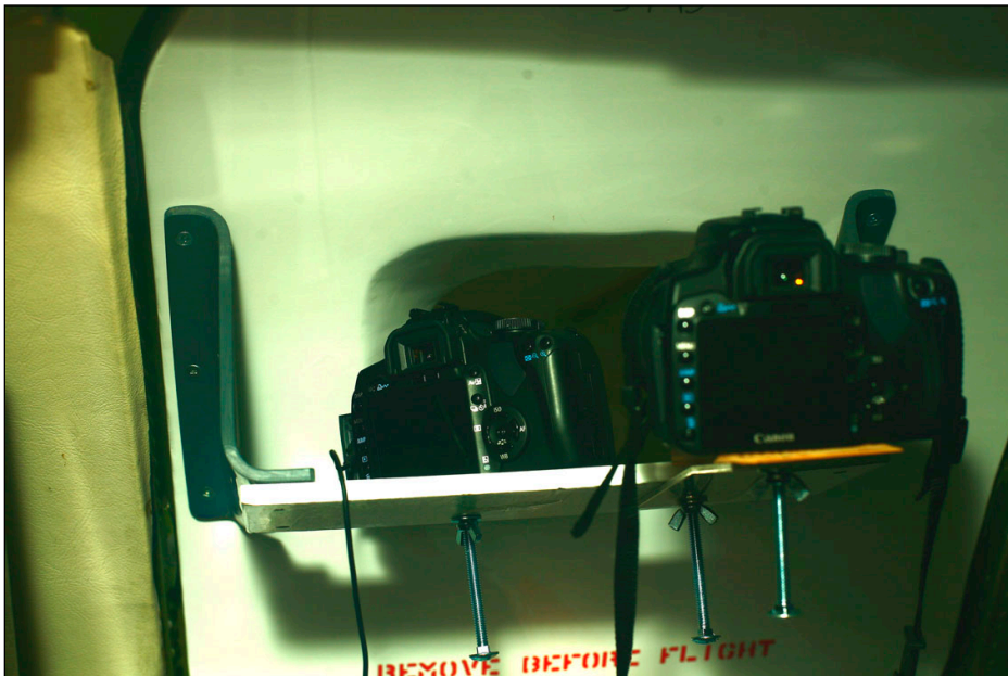
Photo 2.6: Camera Positioning in Emergency Exit Windows (View from Inside)
