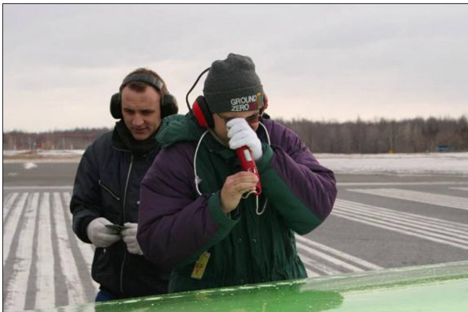
Photo 2.10: Fluid Freezing Point Measurement Using Hand-Held Brixometer
