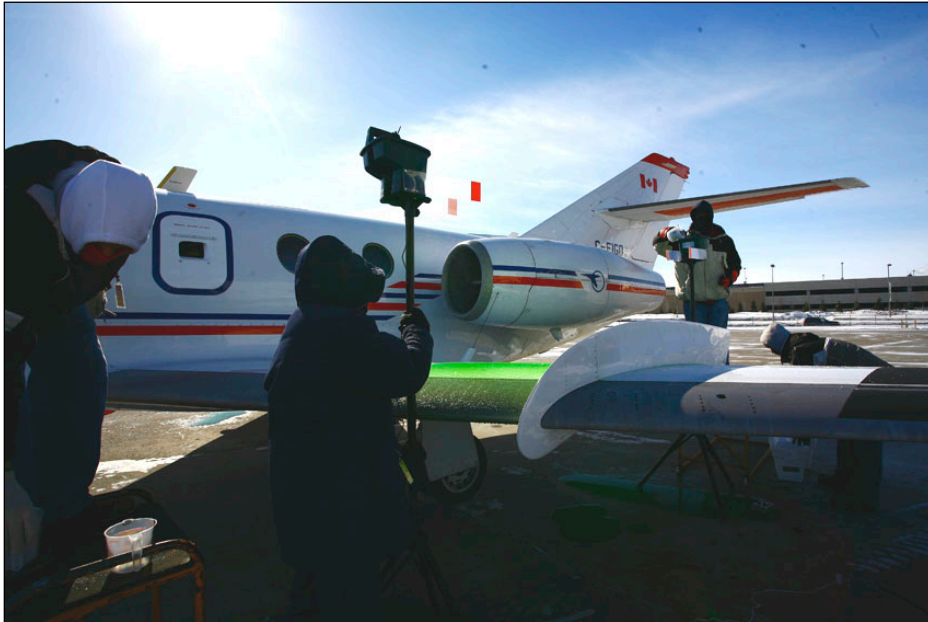
Photo 2.5: Ice Pellet/Snow Dispenser Setup for Falcon 20 Tests
