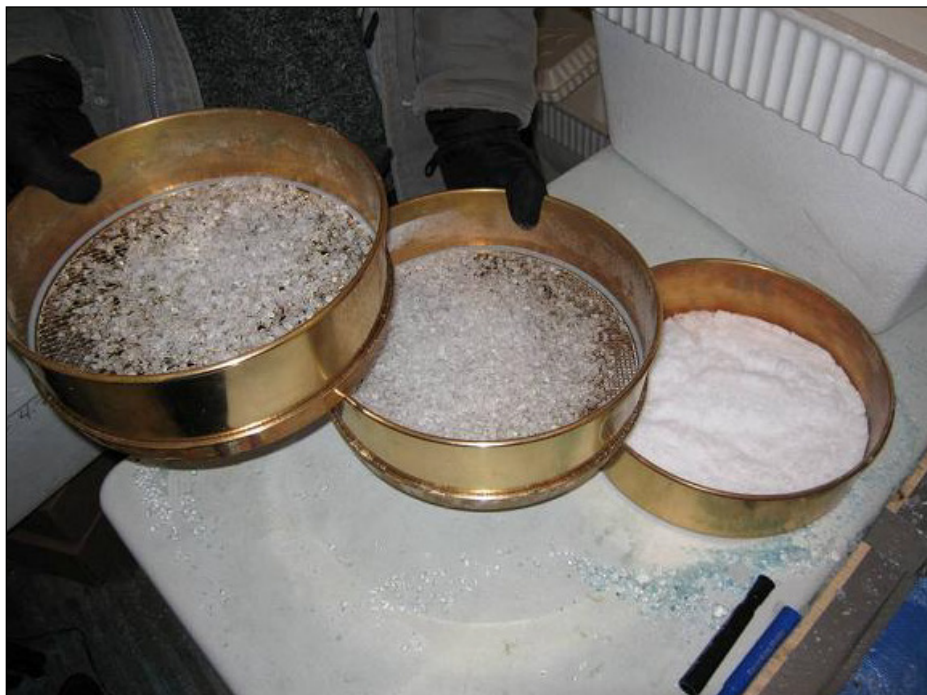
Photo 2.14: Calibrated Sieves Used to Obtain Desired Size Distribution
