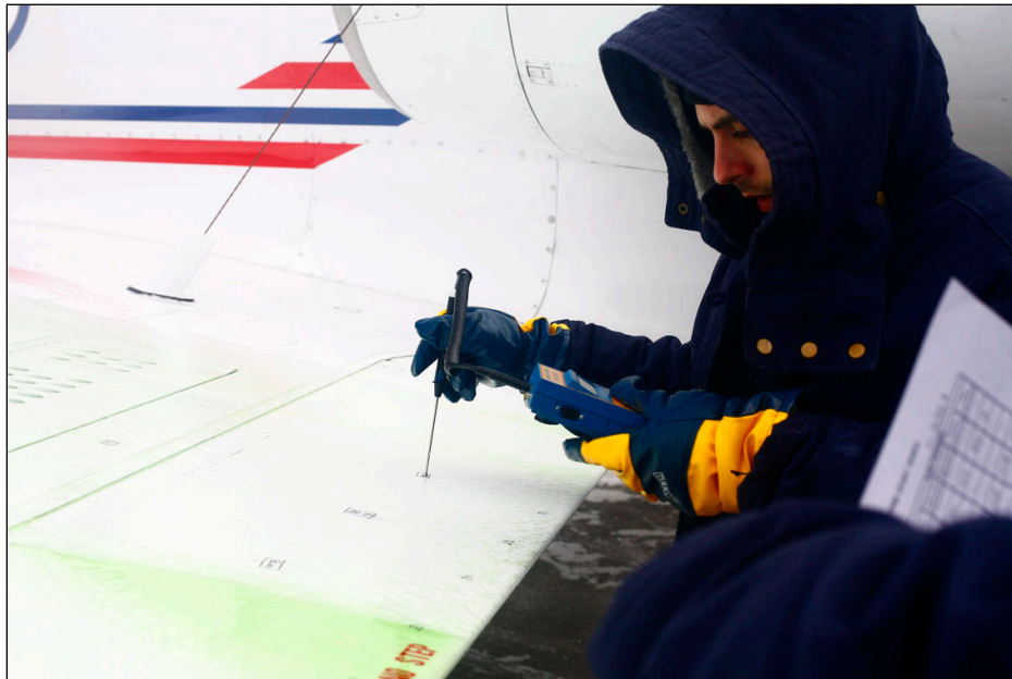
Photo 2.11: Wing Surface Temperature Measurement
