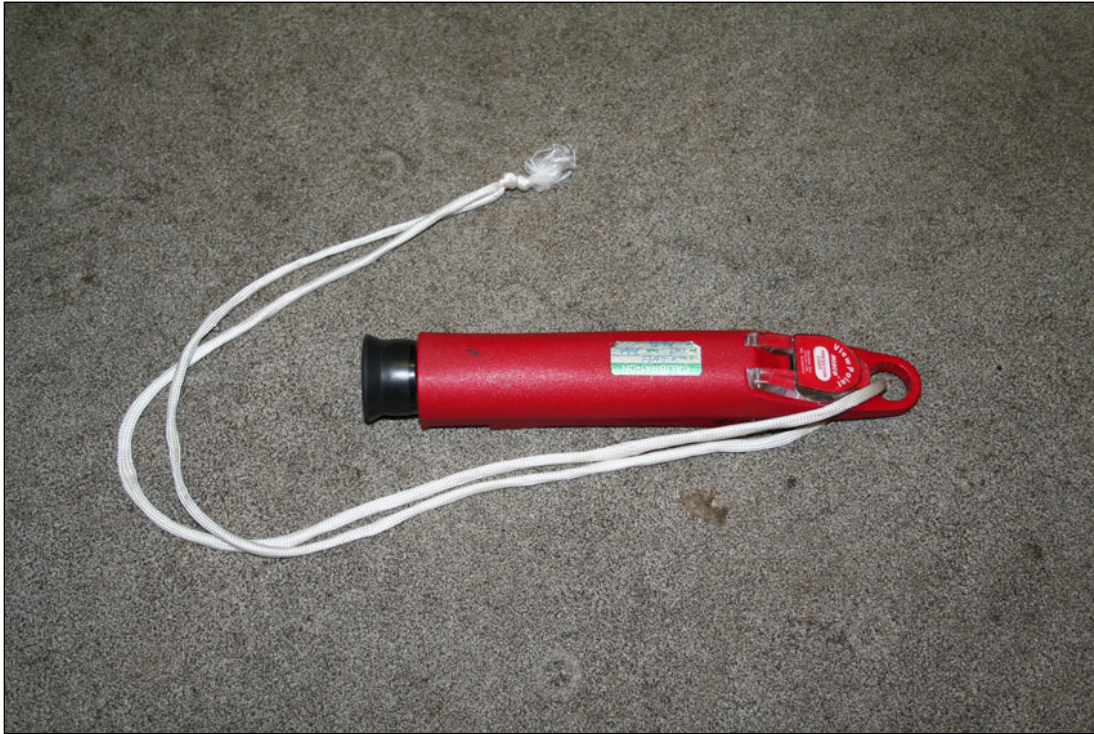
Photo 2.15: Hand-Held Brixometer (Misco 10431VP)
