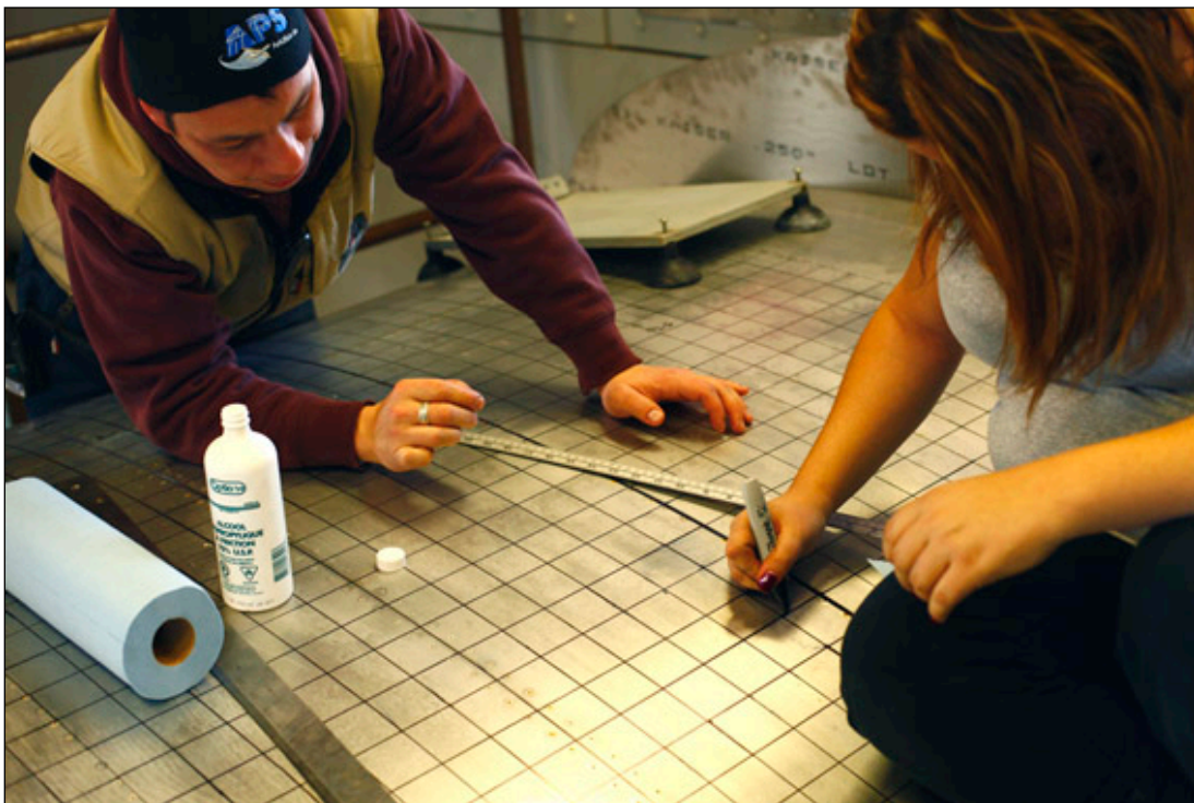
Photo 2.4: Grid Markings on NASA LS(1)-0417 Wing Section
