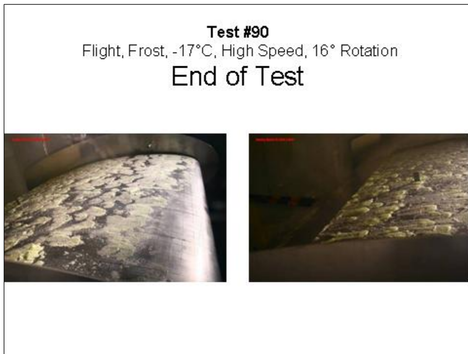
Photo 7.10: Test #90 – End of Test
