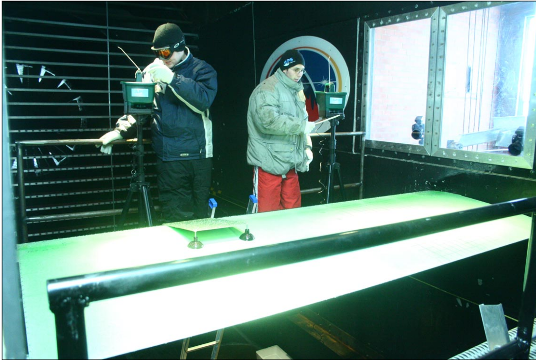
Photo 2.7: Ice Pellet Dispensers Operated by APS Personnel
