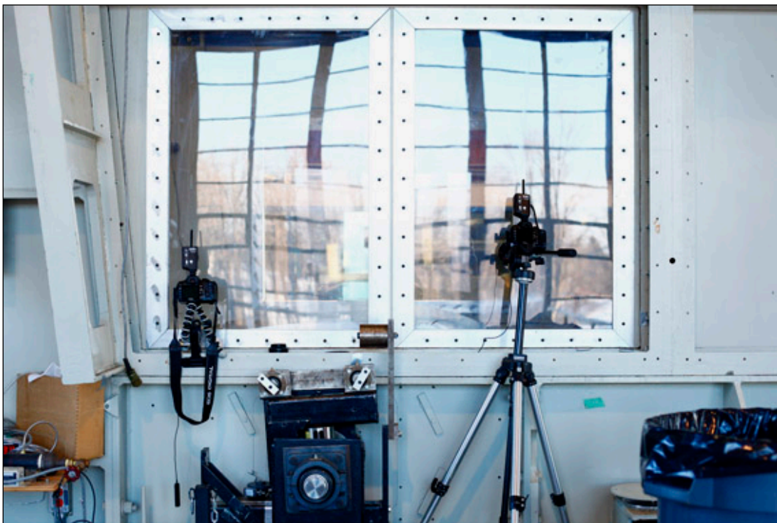
Photo 2.10: Wind Tunnel Setup for Digital Cameras
