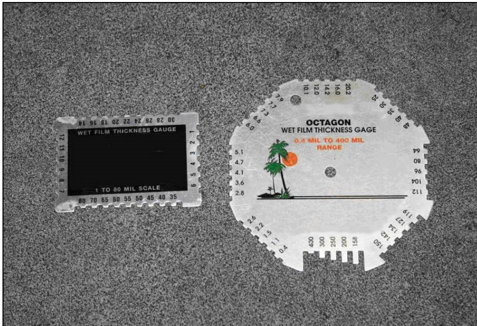
Photo 2.10: Wet Film Thickness Gauges
