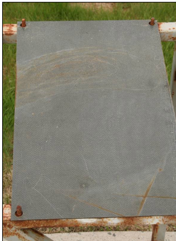
Photo 2.6: Unpainted Composite (Comp 05) Flat Plate
