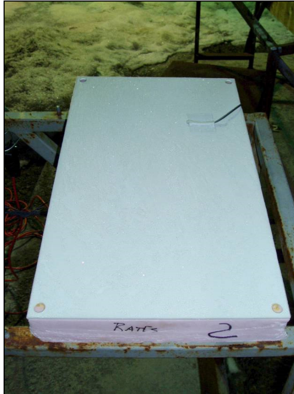
Photo 2.9: White-Painted Aluminum Frosticator Plate
