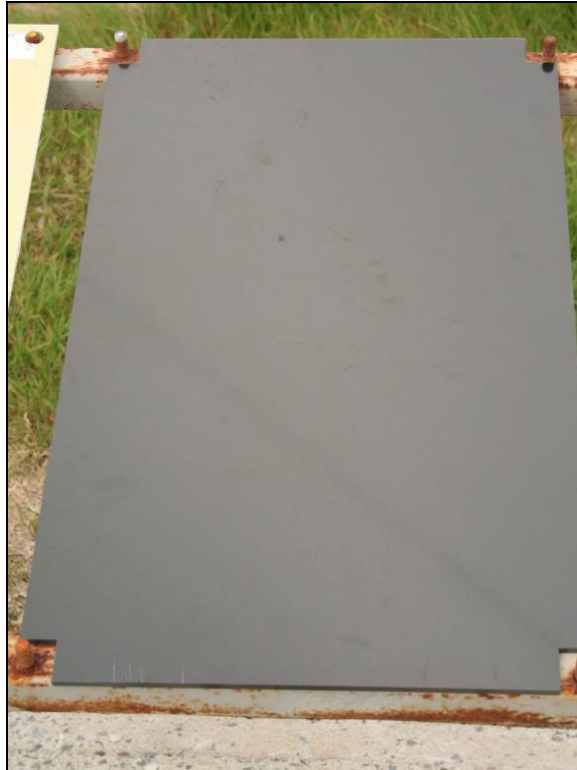
Photo 4.3: Unpainted Carbon Fibre Unidirectional Tape Test Plate
