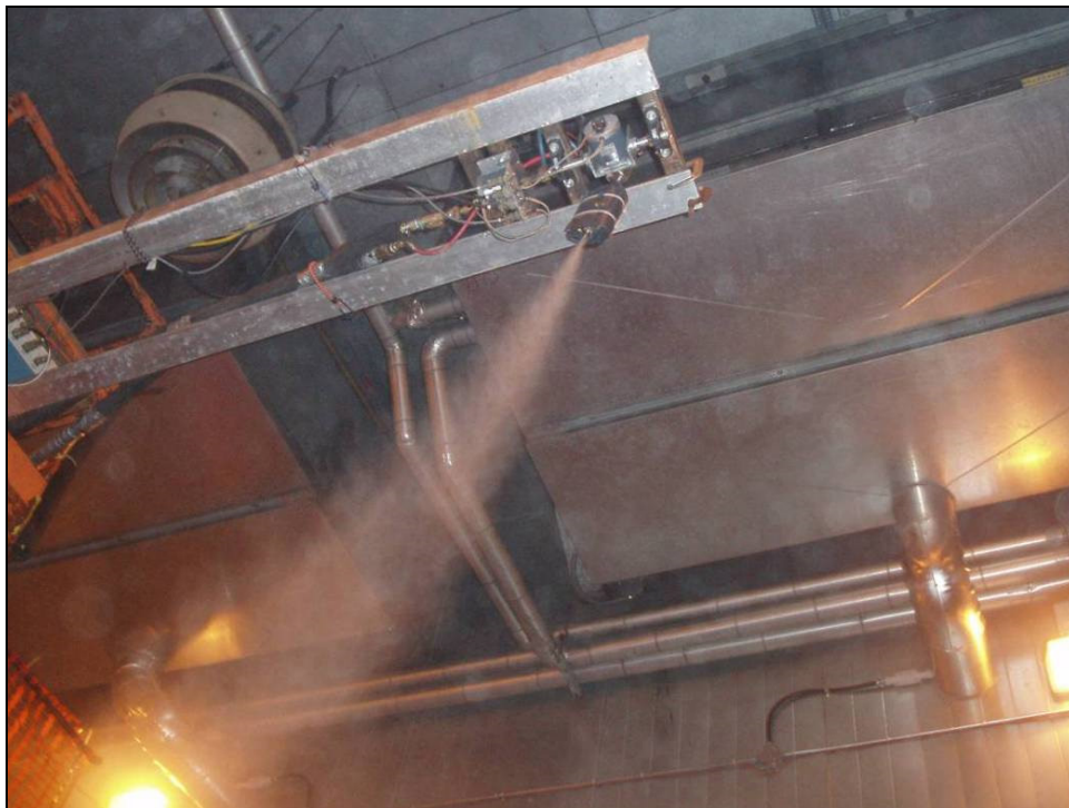
Photo 2.4: Sprayer Assembly Used to Produce Fine Droplets
