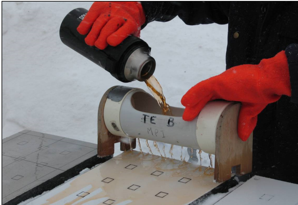
Photo 2.12: Twelve-Hole Spreader Used for Fluid Application
