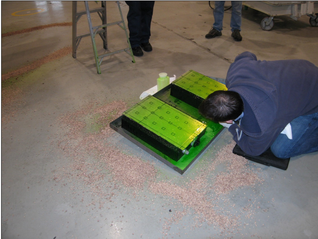
Photo 2.4: Leading Edge Thermal Equivalent Boxes (With Fluid)
