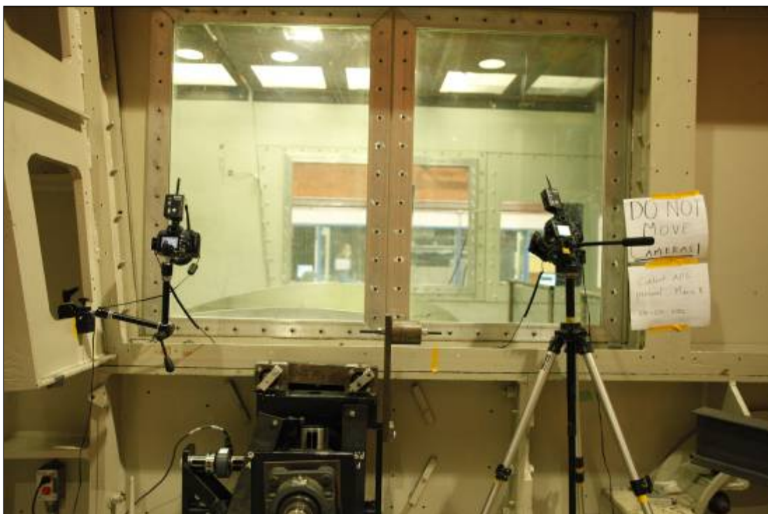
Photo 2.10: Wind Tunnel Setup for Digital Cameras
