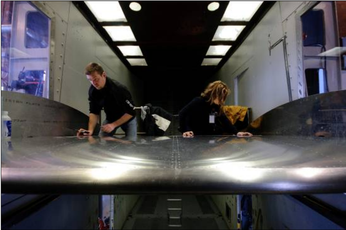
Photo 2.3: Supercritical Wing Section Used for Testing
