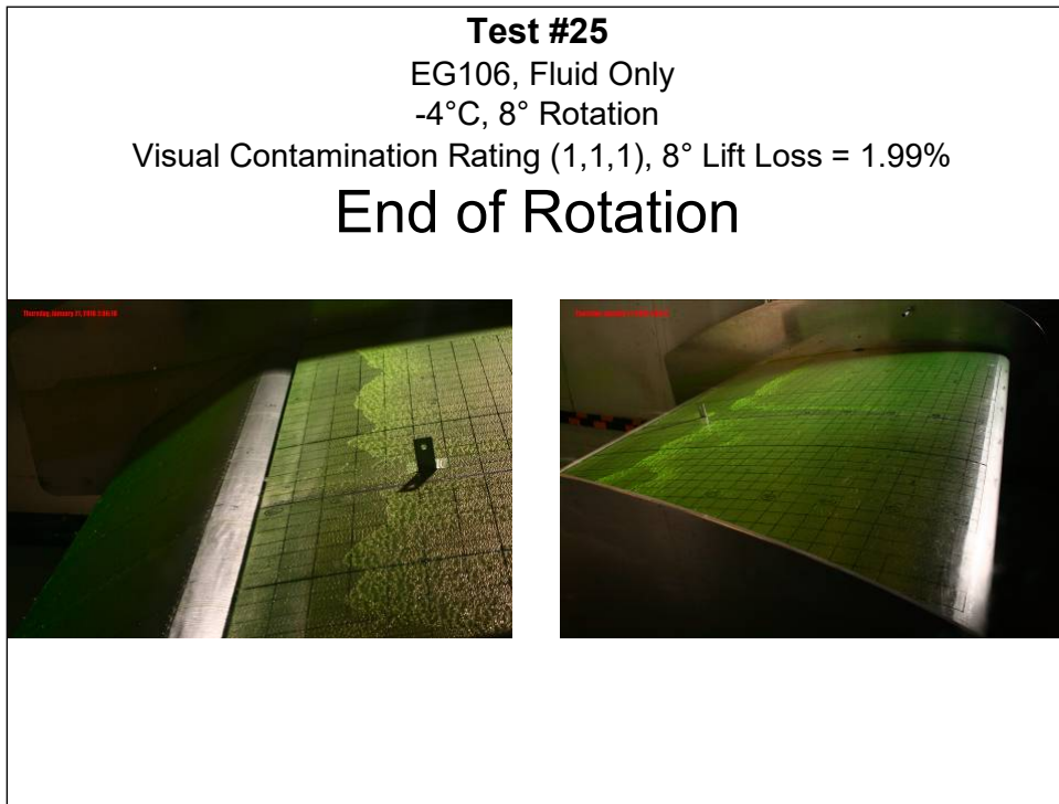
Photo 11.37: Test #25 – End of Rotation
