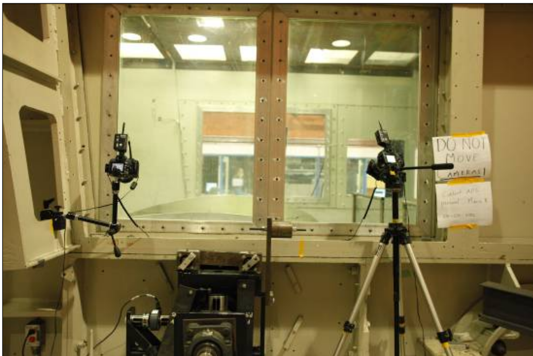
Photo 2.10: Wind Tunnel Setup for Digital Cameras
