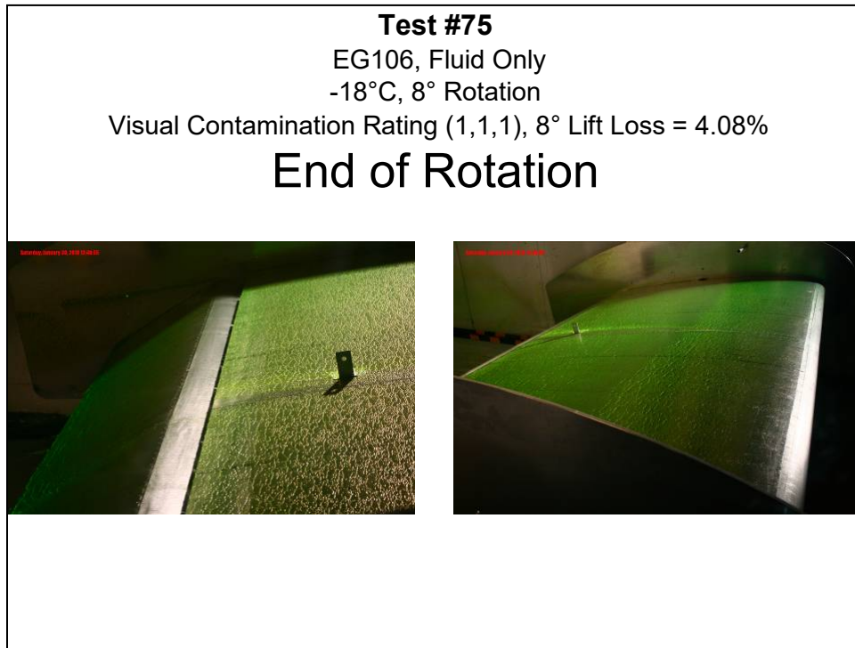
Photo 10.61: Test #75 – End of Rotation
