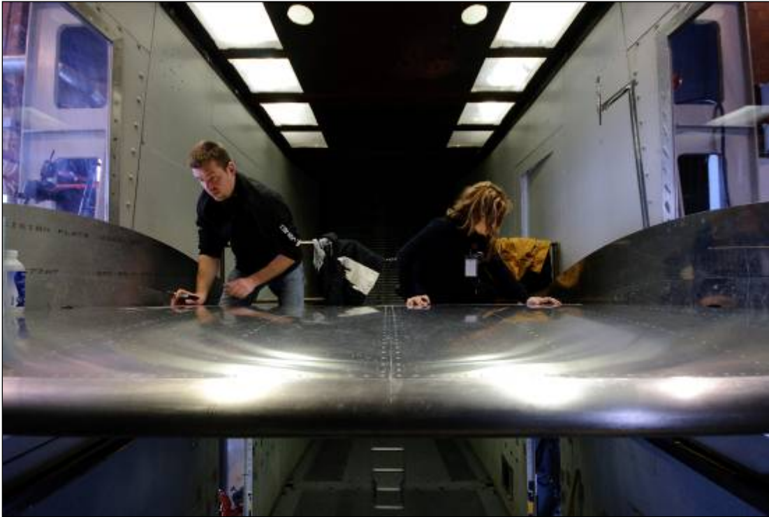
Photo 2.3: Supercritical Wing Section Used for Testing
