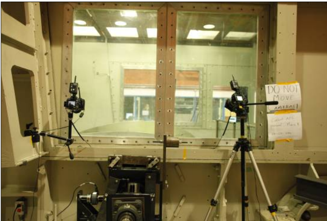
Photo 2.10: Wind Tunnel Setup for Digital Cameras
