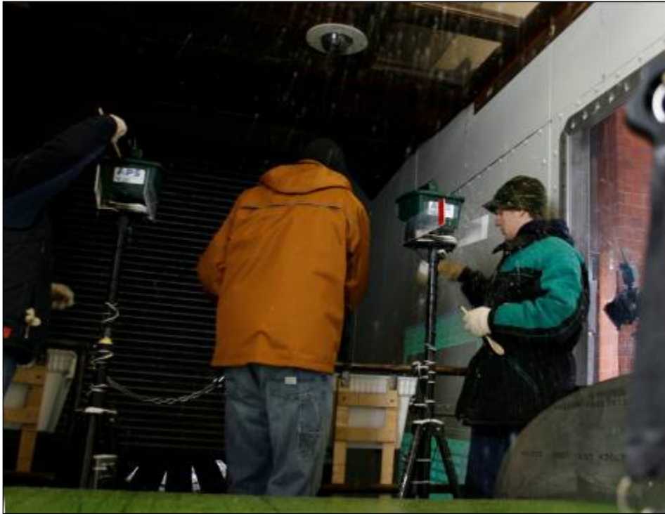
Photo 2.7: Ice Pellet Dispensers Operated by APS Personnel
