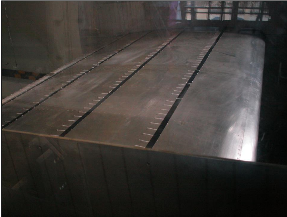
Photo 6.3: Tufts Flow Visualization
