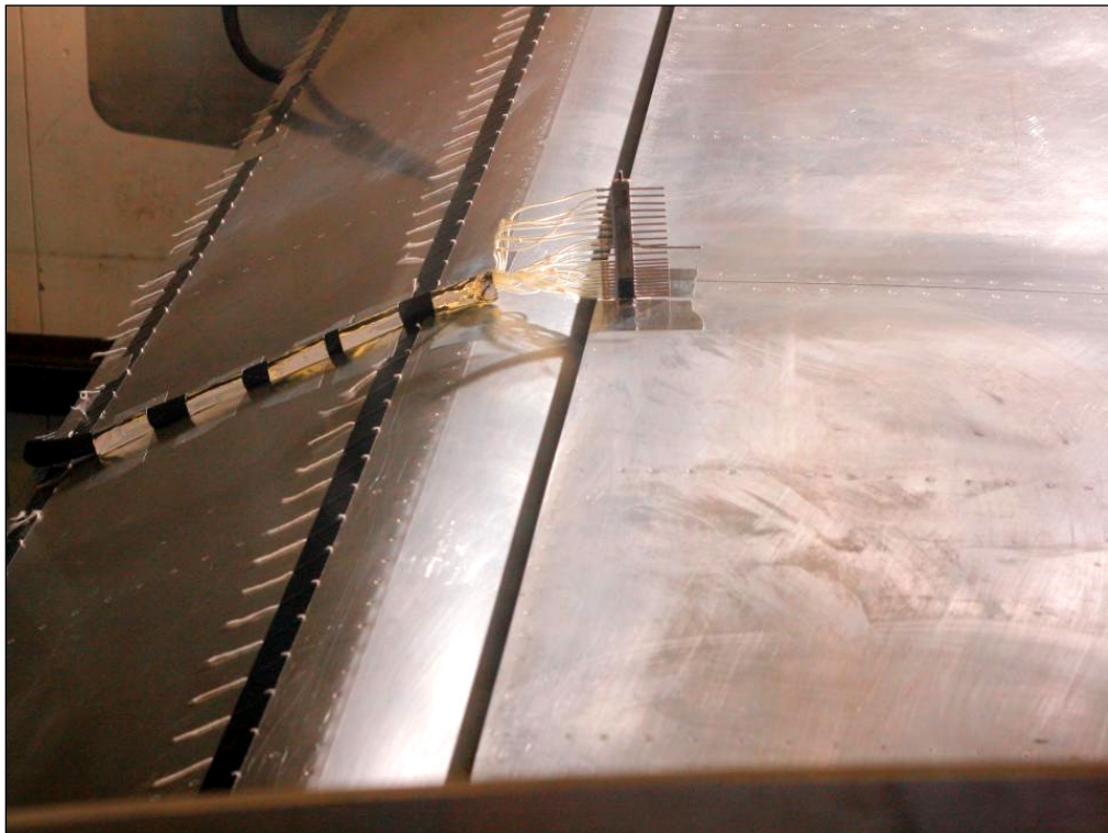
Photo 6.4: Boundary Layer Rake Tests
