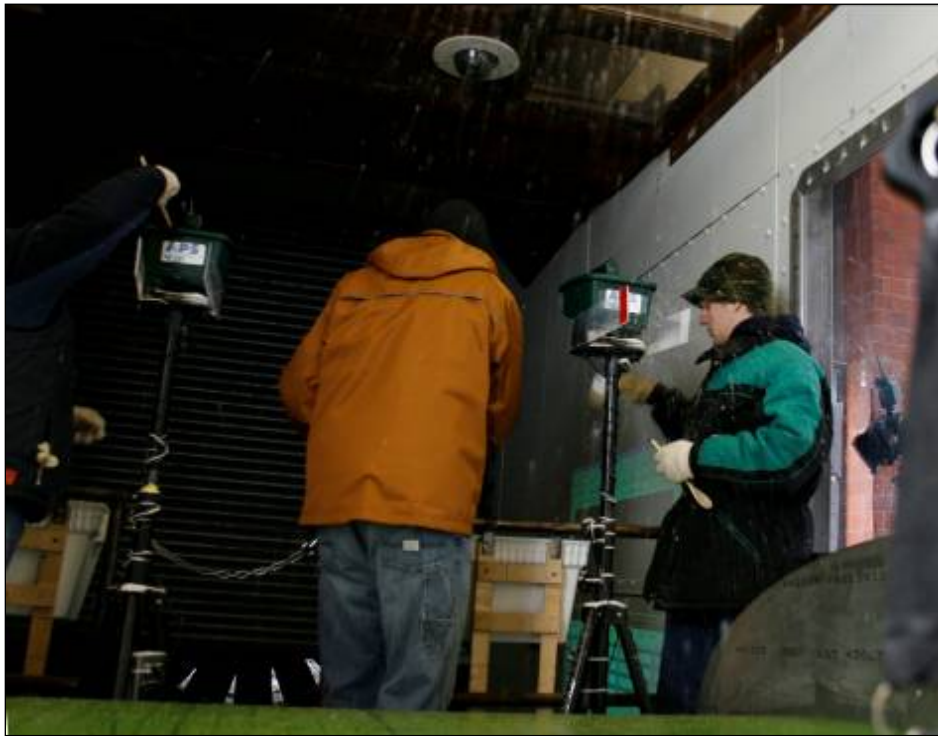
Photo 2.7: Ice Pellet Dispensers Operated by APS Personnel
