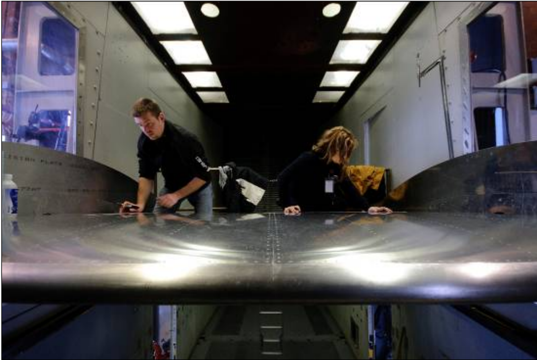
Photo 2.3: Thin High-Performance Wing Section Used for Testing
