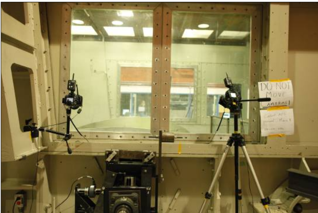
Photo 2.10: Wind Tunnel Setup for Digital Cameras
