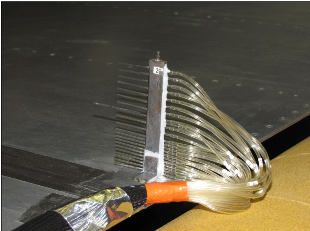
Photo 5.2: Boundary Layer Rake Tests
