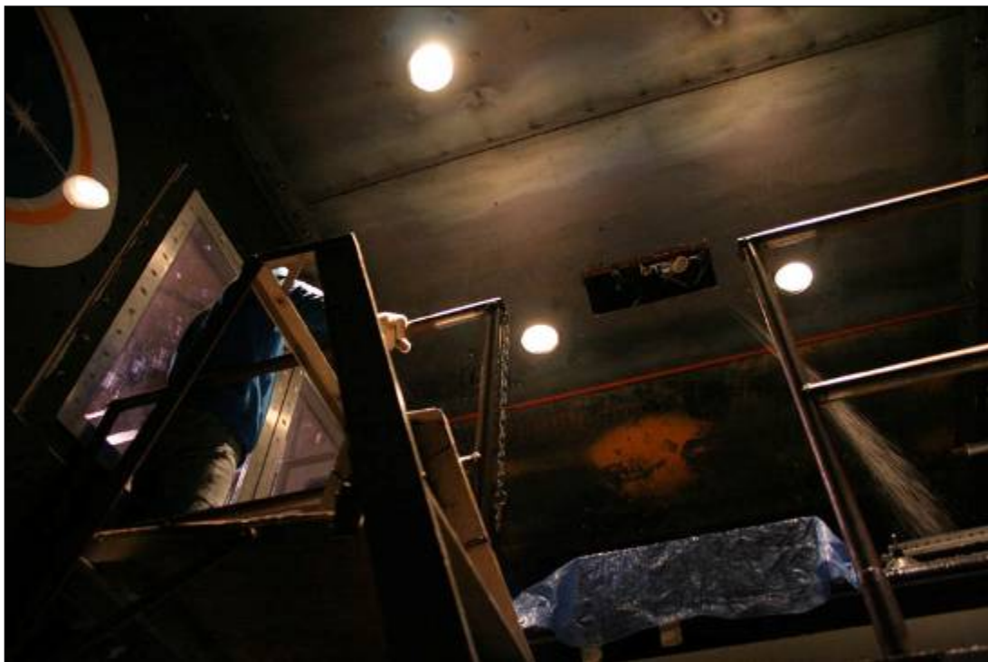
Photo 2.8: Ceiling-Mounted Freezing Rain Sprayer
