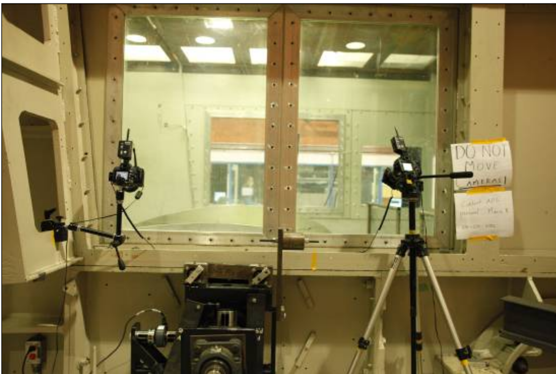
Photo 2.10: Wind Tunnel Setup for Digital Cameras
