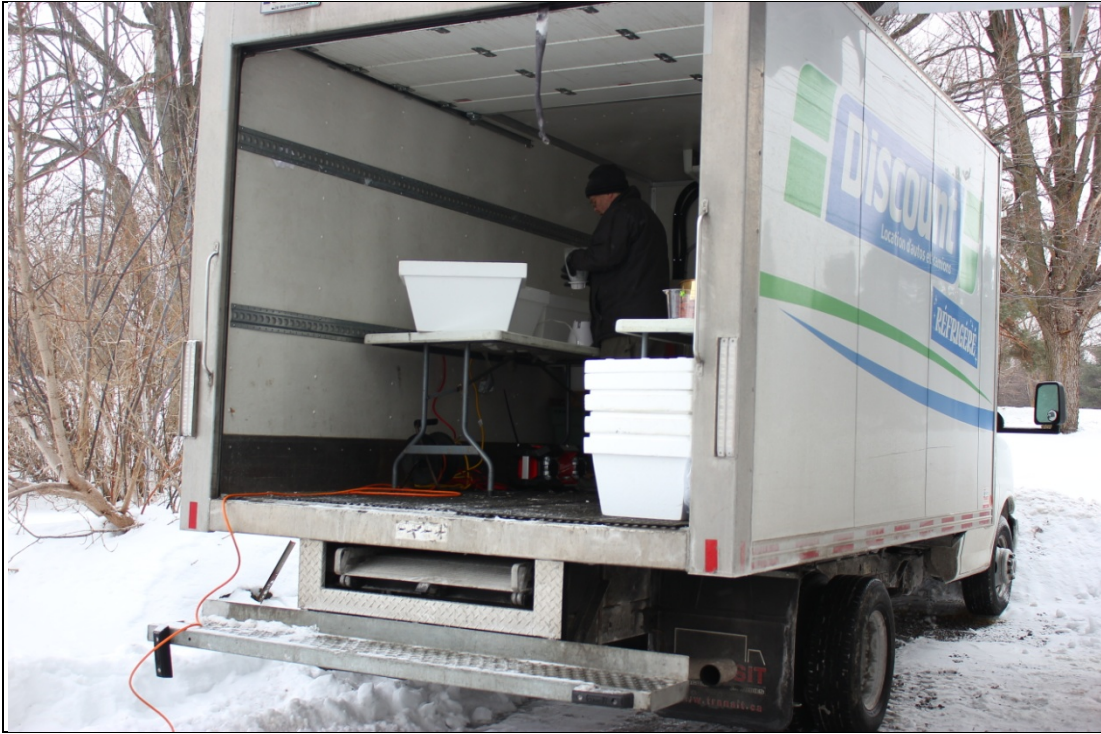
Photo 2.5: Refrigerated Truck Used for Manufacturing Ice Pellets
