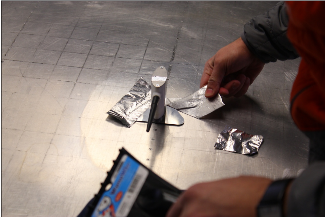
Photo 3.1: Installation of APM Unit with Speed-Tape to Wing
