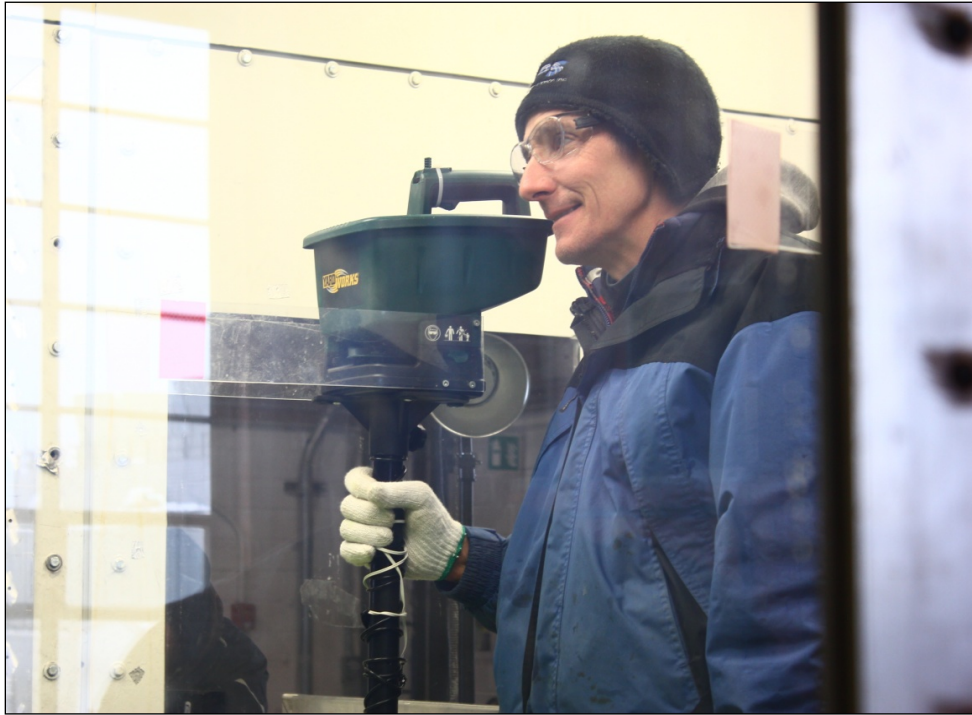
Photo 6.1: Old Ice Pellet Dispenser System
