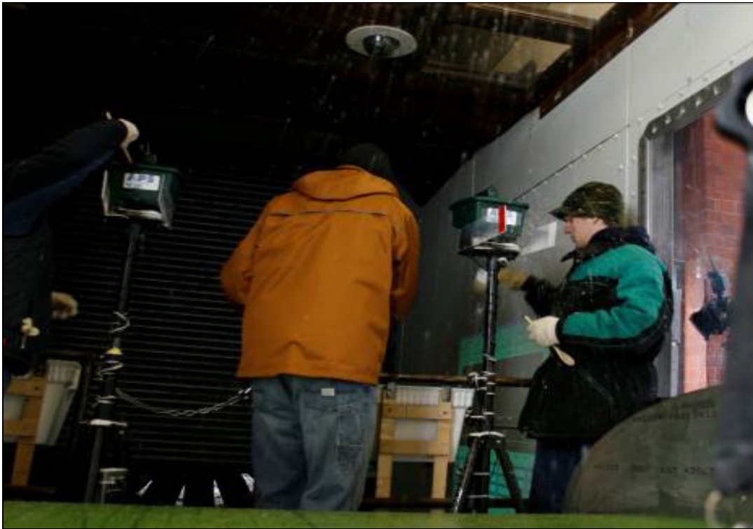
Photo 2.7: Ice Pellet Dispensers Operated by APS Personnel
