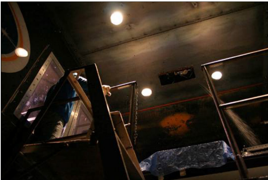
Photo 2.8: Ceiling-Mounted Freezing Rain Sprayer
