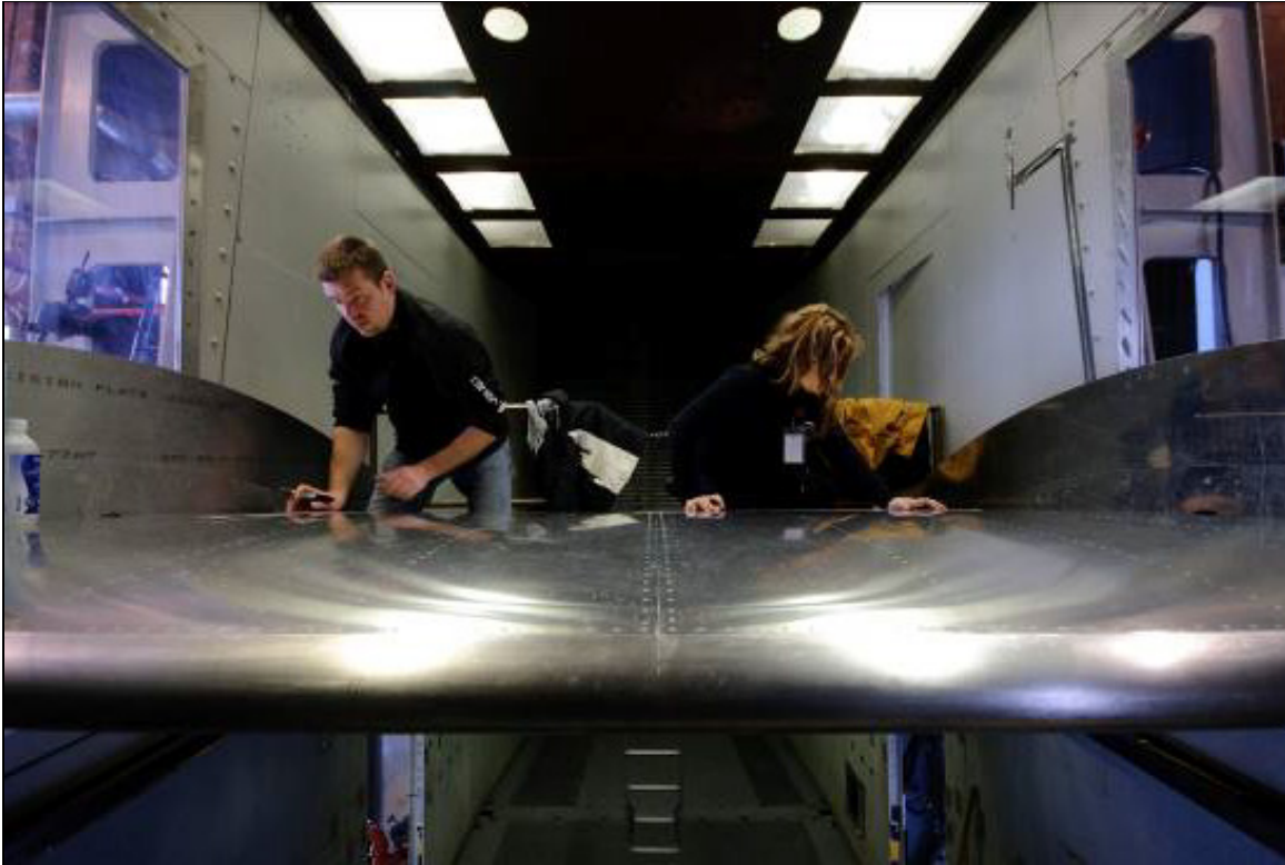
Photo 2.3: Thin High-Performance Wing Section Used for Testing
