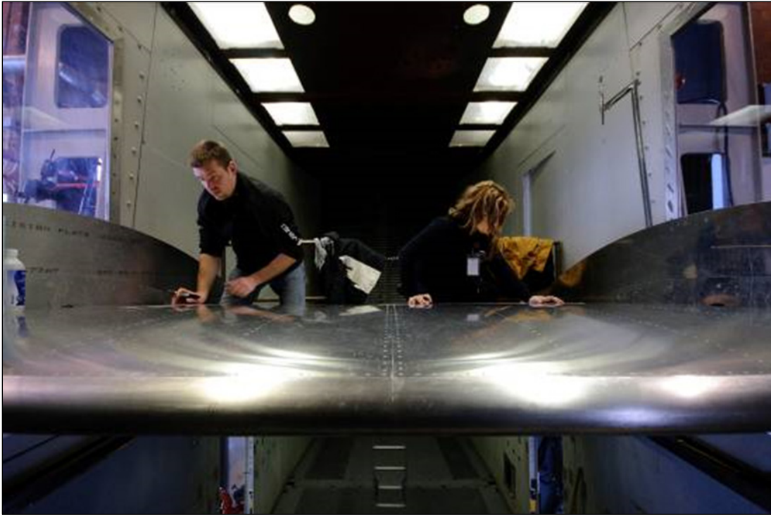
Photo 2.3: Thin High-Performance Wing Section Used for Testing
