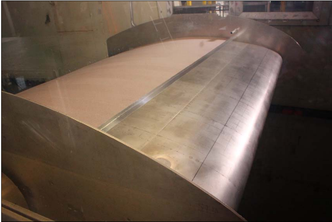
Photo 6.3: Sandpaper Roughness Tests
