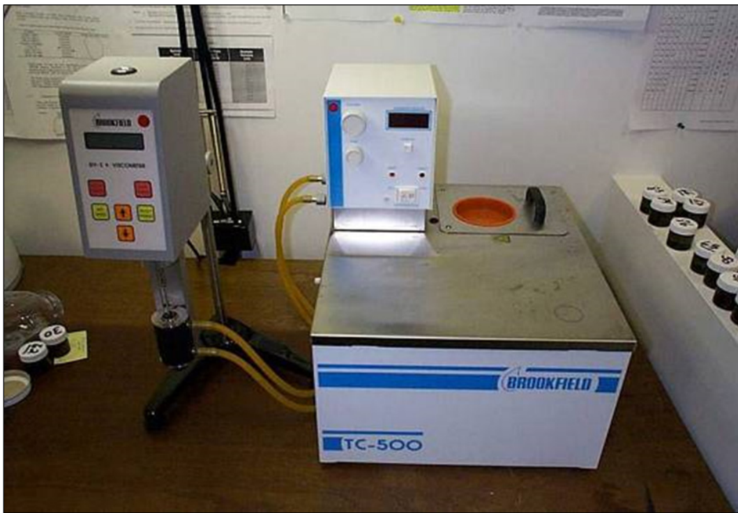
Photo 2.14: Brookfield Digital Viscometer Model DV-1 +
