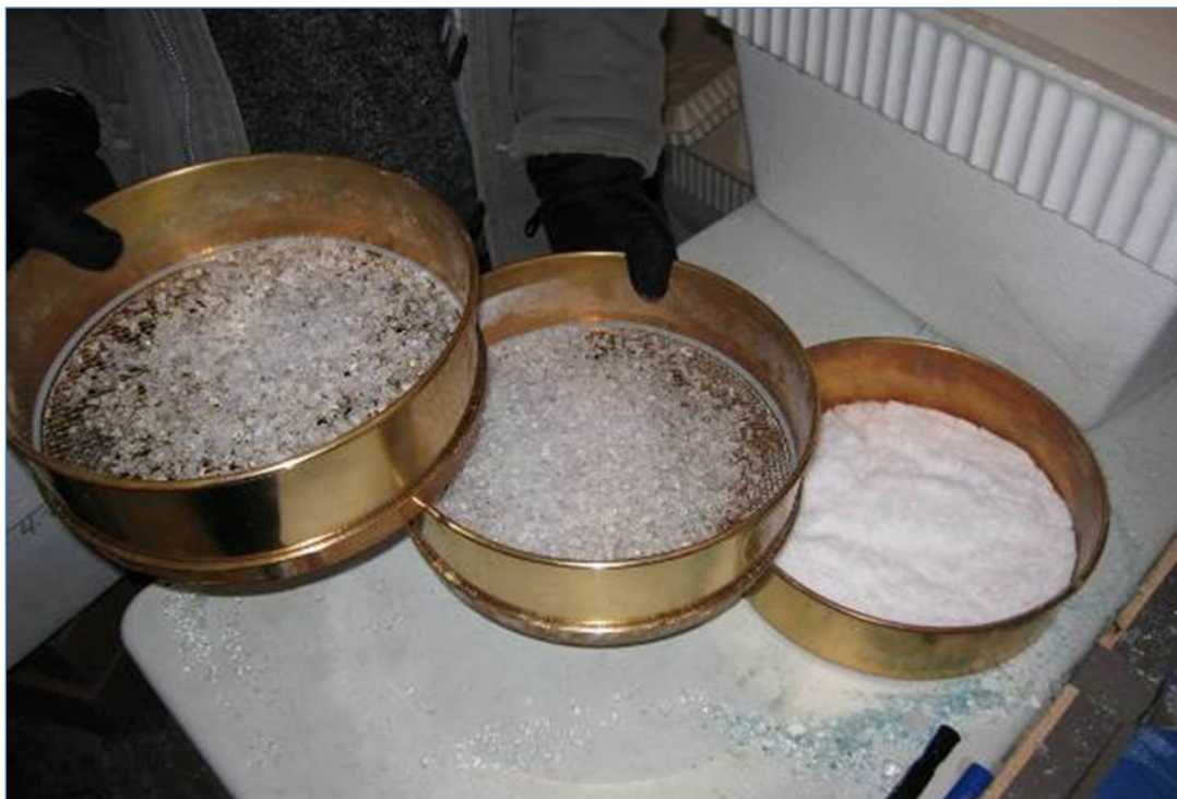
Photo 2.6: Calibrated Sieves Used to Obtain Desired Size Distribution
