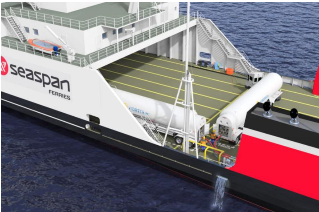
Figure 34: Onboard LNG Tanker Truck Bunkering (Seaspan Ferries, 2015)
