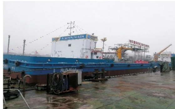
d. 3 rd generation (liquid input/output at the top of the tank with refueling function)
