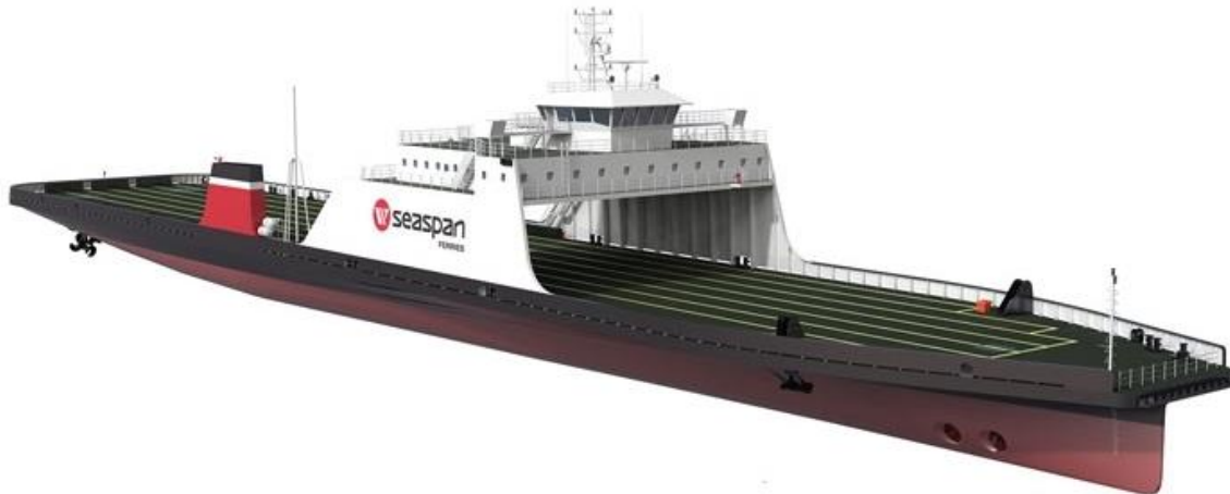
Figure 57: Seaspan Hybrid Ferry with Storage Battery and Dual Fuel Engine Propulsion
