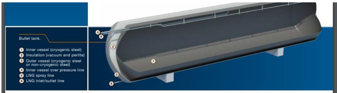
Figure 14: Bullet Type Storage Tank (Wartsila)
