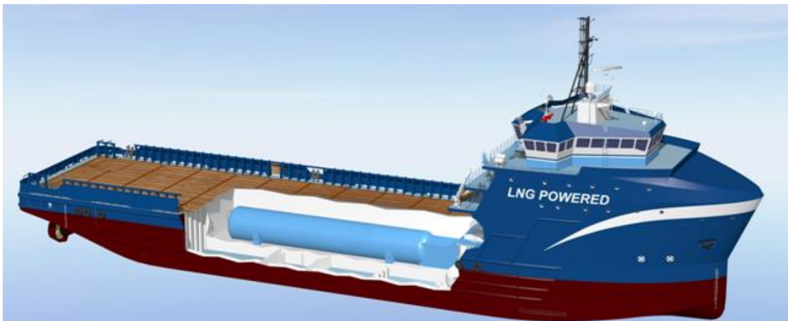
Figure 40: LNG Powered PSV with Type C Tank
