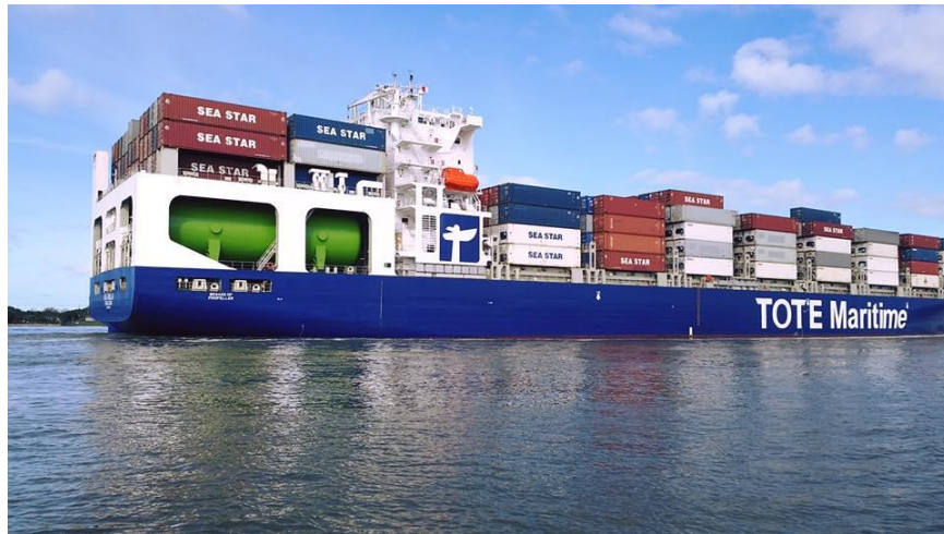
Figure 50: TOTE Isla Bella Dual Fuelled Marline Class Containership with Direct Drive Slow-Speed Engine
